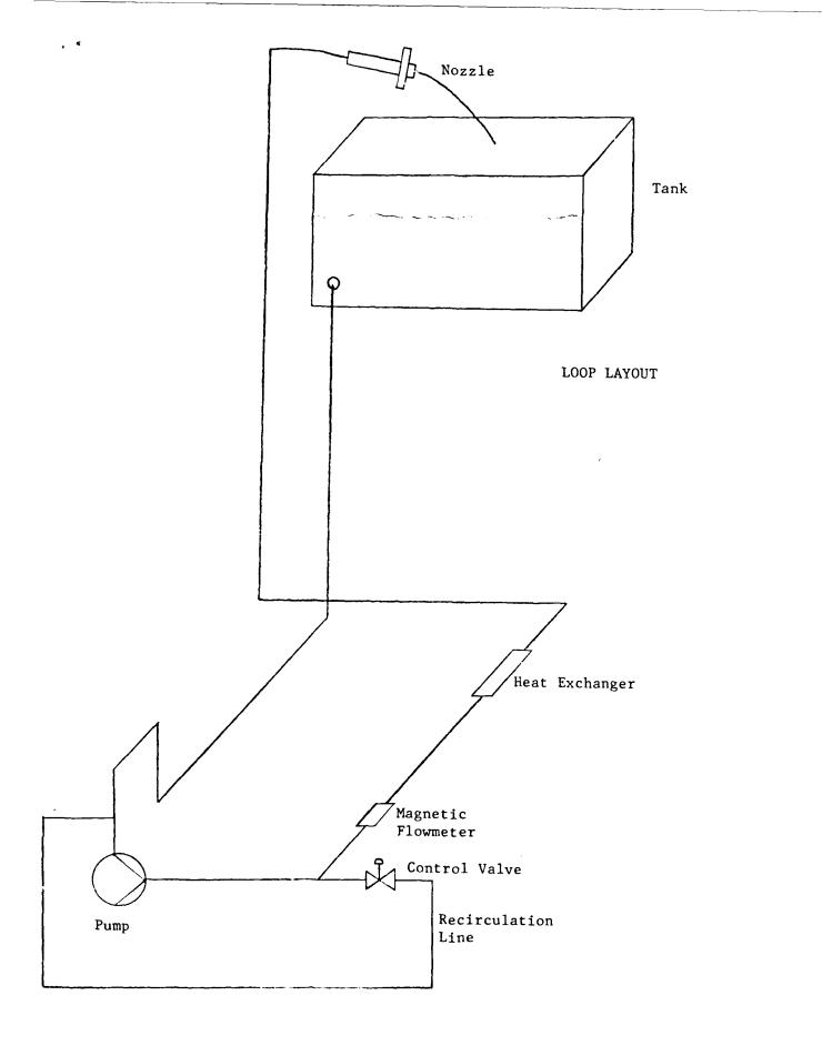
Figure-3 Primary Liquid Test Loop
