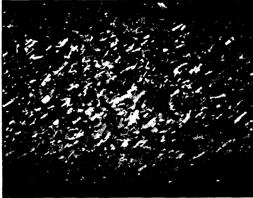
Fig. 7. The melt-textured longitudinal section of sample 10377-15B MT6 in polarized light showing finer grain size compared with the sample 10377-15B MT5 due to higher maximum temperature at 1006°C but the travelling speed was too fast for producing sufficient liquid phase. The sample shows very slight grain alignment (200X)
