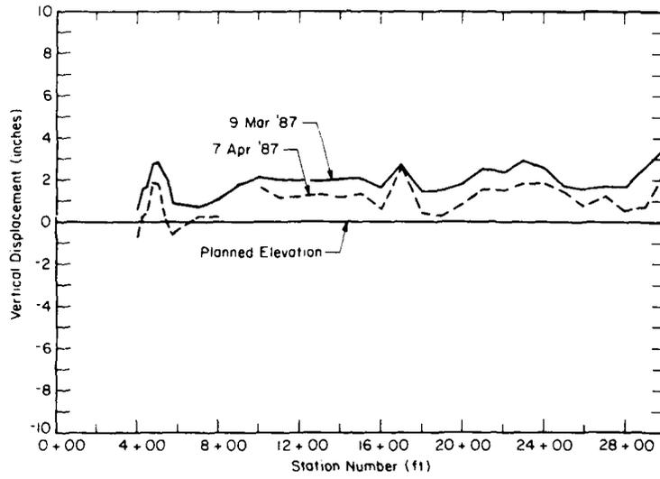
Figure 10. Surface elevations along centerline—Newton Field.
