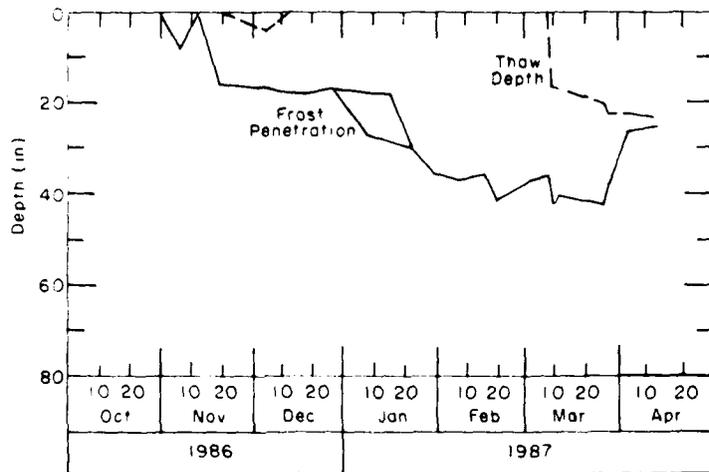
c. Frost/thaw depth vs time—Newton Field.
