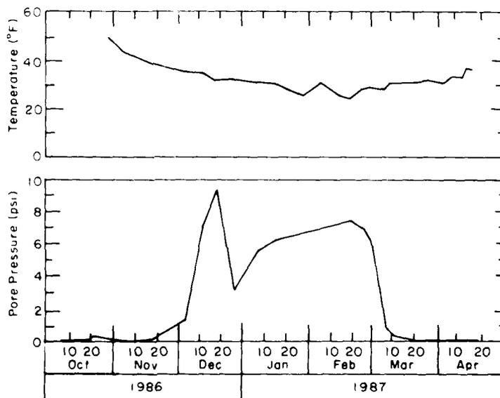
Figure 22. Correlations between tensiometer readings and frost determined by thermocouple readings.
