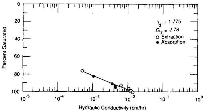
Figure A3. Hydraulic conductivity—Newton Field station 4+55, subgrade.
