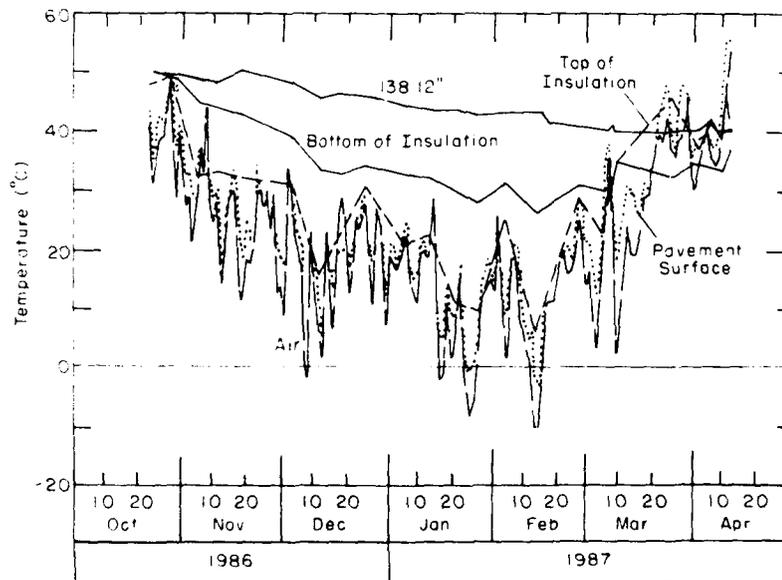
Figure 19. Air, surface, and subsurface temperature vs time.
