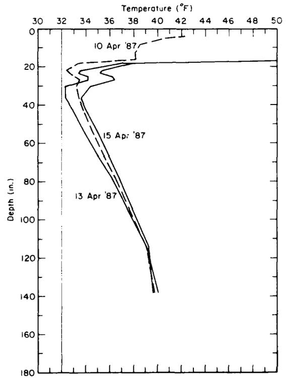
Figure 15. Temperature vs depth immediately beneath the insulation (thawing)—Newton Field.
