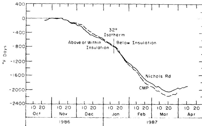
b. Air freezing index vs time.
