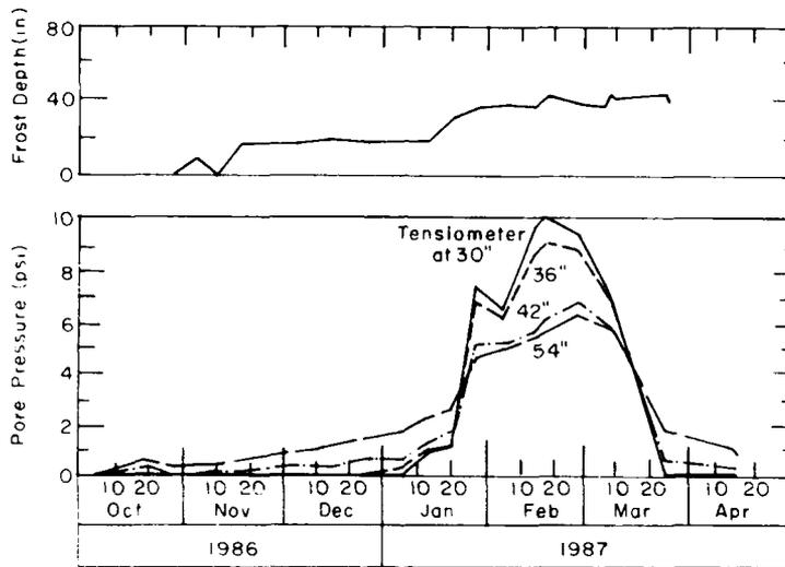
c. Newton Field—tensiometer readings at 30, 36, 42, and 54 in.
