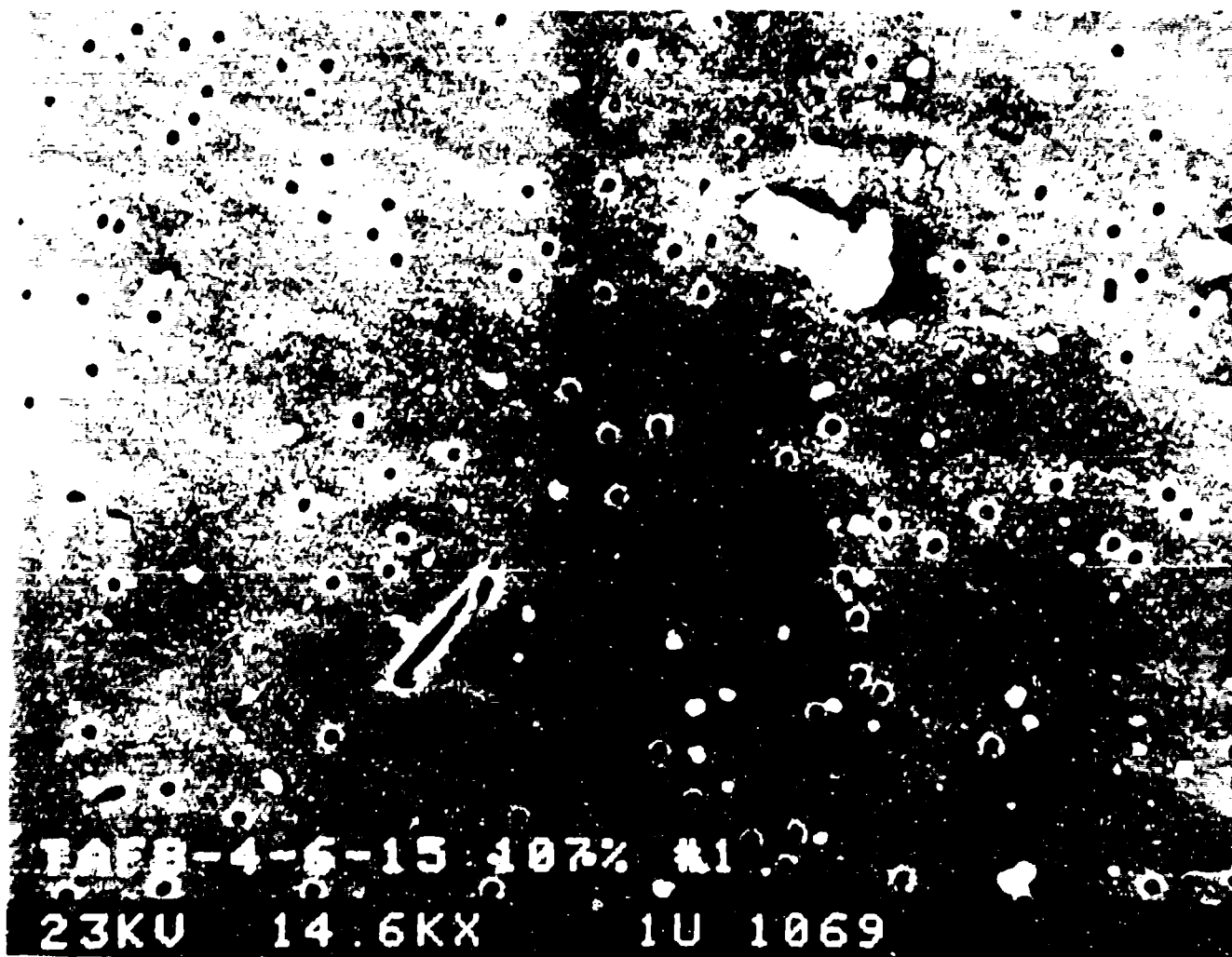
Figure 18. Photomicrograph of Exhaust Particles From F110 Engine At Intermediate Power (Filter Pores are 0.1 \mu\text{m} Diameter)
