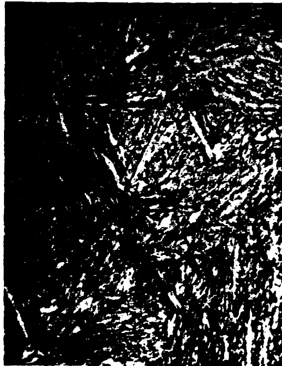
Figure 19. Photomicrograph of an etched muzzle end sample revealing a tempered martensitic microstructure (1000X).
