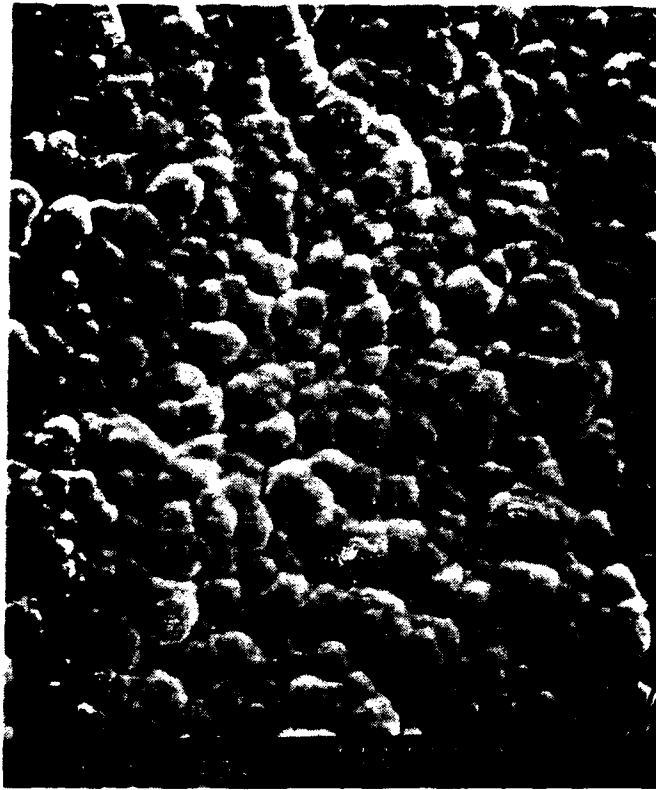
Figure 4. SEM micrograph of a SiC-coated composite after oxidation test at 1500°C, 10 hours.
