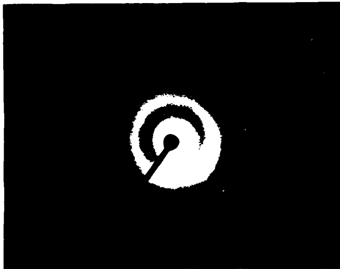
Figure 30. TEM Selecting Area (SAD) Pattern of the Glass Phase Shown in Figure 29.
