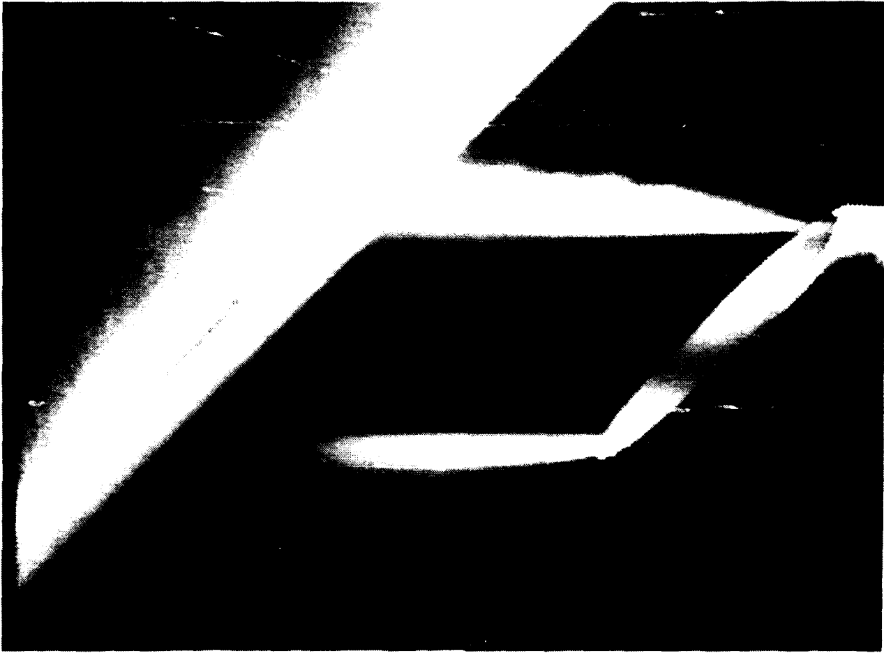
Figure 14. Simultaneous axial and transverse cross-sections of unexcited jet; U = 20 m/s.
