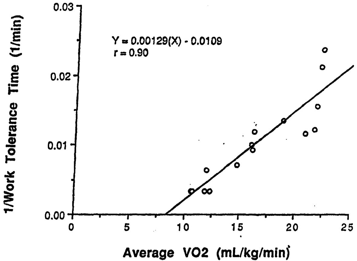
**Figure 20.** Inverse of work tolerance time plotted against the average metabolic rate for TOPP High and 30°C.
