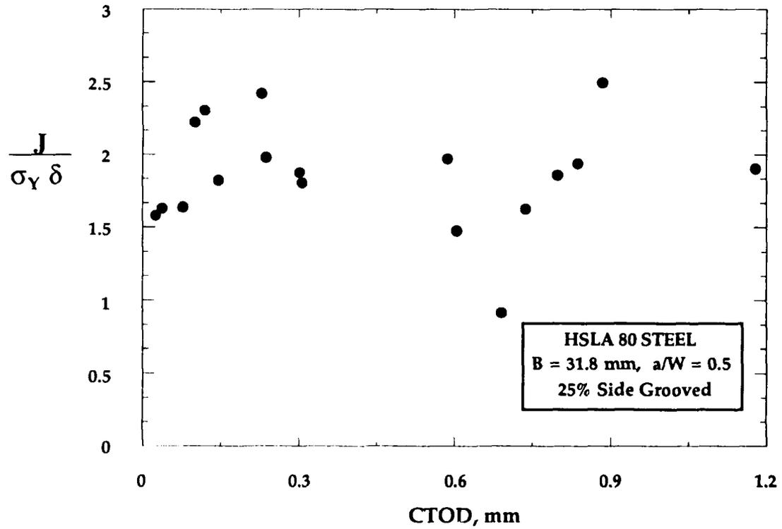
FIGURE 4.8 Experimental J-CTOD ratio for the HSLA 80 steel.
