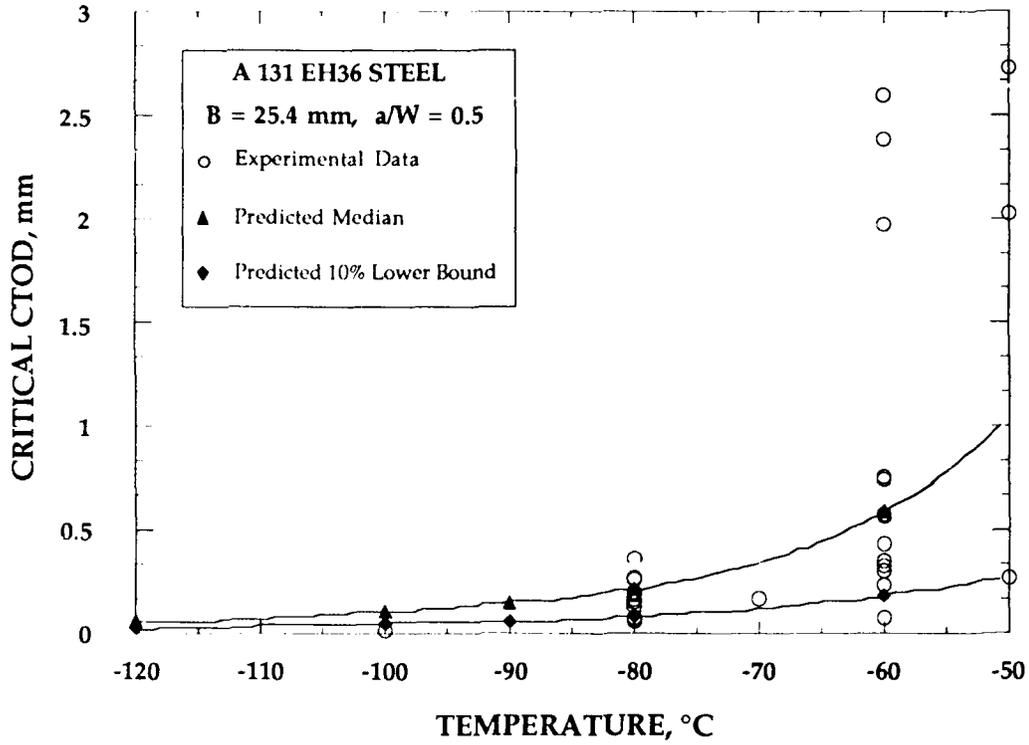
FIGURE 4.13 Predicted and experimental CTOD values for A 131 EH36 steel.
