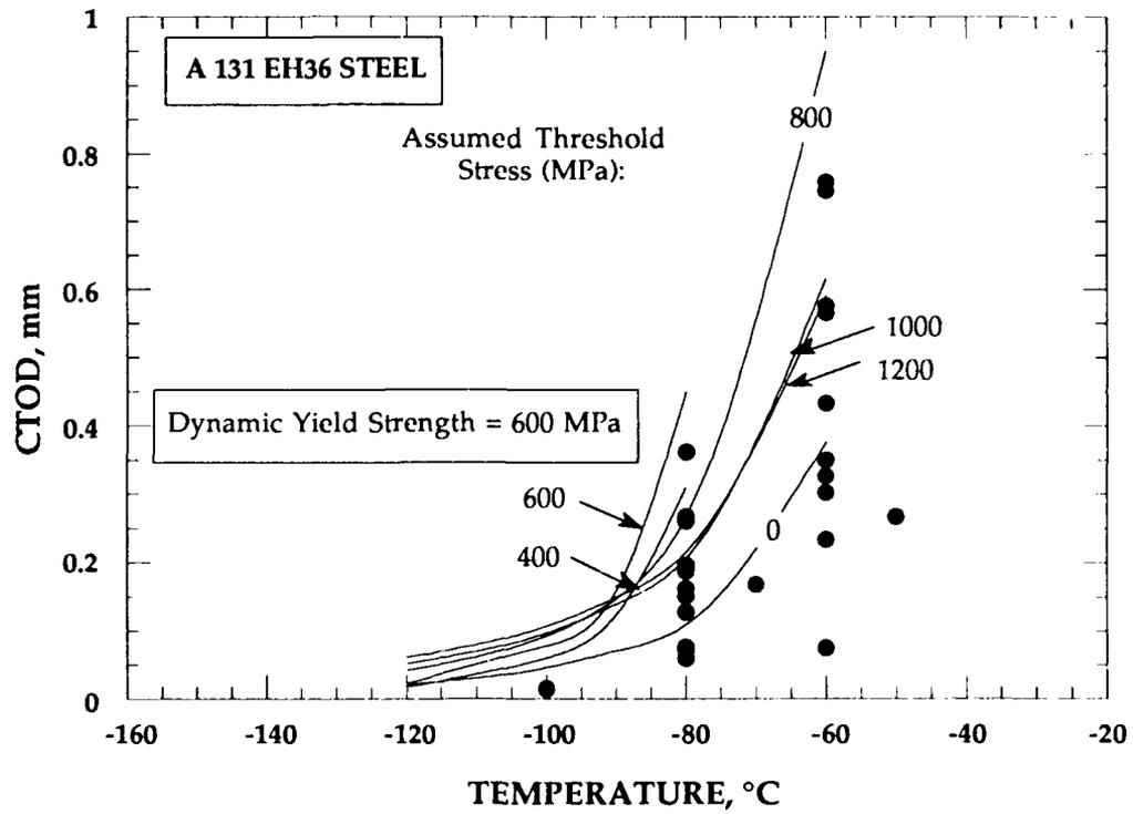
FIGURE 4.15 Effect of the assumed threshold stress on predicted CTOD in the A 131 EH 36 steel.
