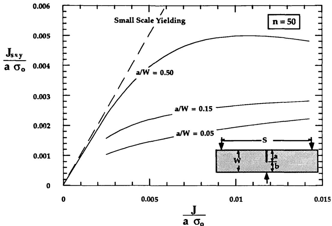
FIGURE 3.15 Comparison of effective and apparent driving force for  $n = 50$
