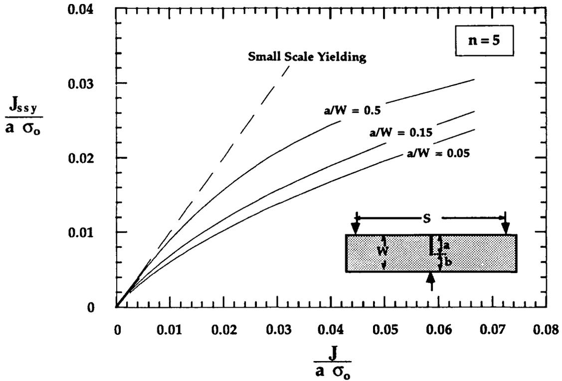
FIGURE 3.13 Comparison of effective and apparent driving force for  $n = 5$
