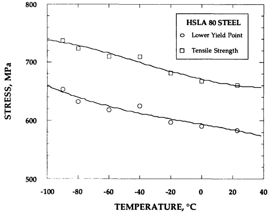
FIGURE 2.3 Quasistatic tensile properties of the HSLA 80 steel plate.
