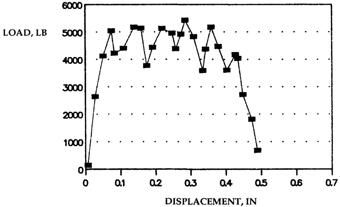
FIGURE 2.6 Load elongation curve for A131 EH36 steel at 23°C. Strain rate = 280 s<sup>-1</sup>
