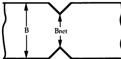
(b) HSLA 80 side grooved specimens (T-L orientation).
