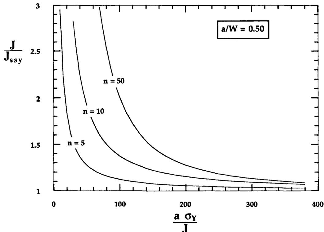
FIGURE 3.16  $J/J_{ssy}$  as a function of strain hardening,  $J$  and flow stress.
