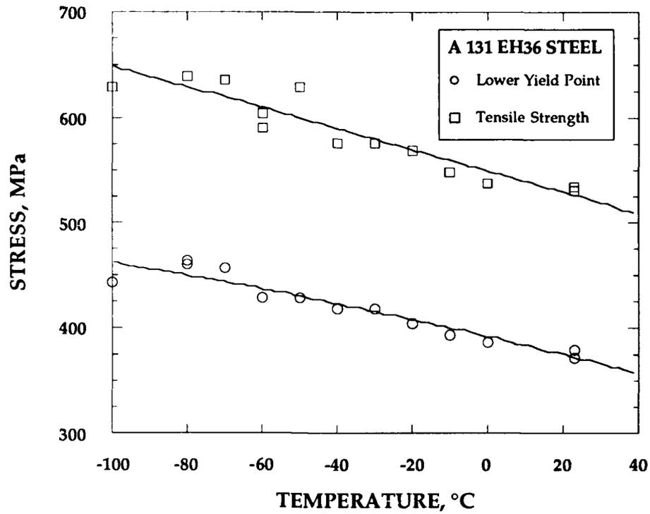
FIGURE 2.2 Quasistatic tensile properties of the A131 EH36 steel plate.
