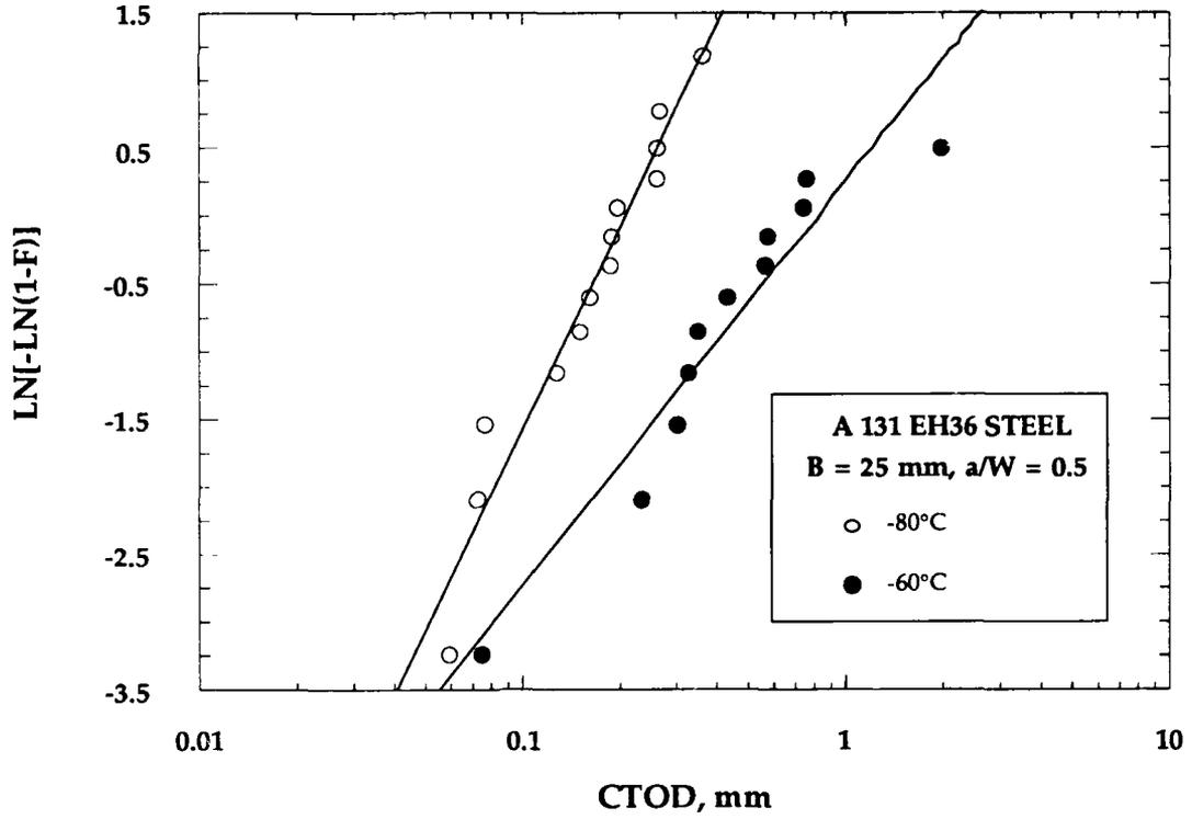
FIGURE 2.18 Weibull plot of CTOD data in the transition region for A 131 EH36 steel.
