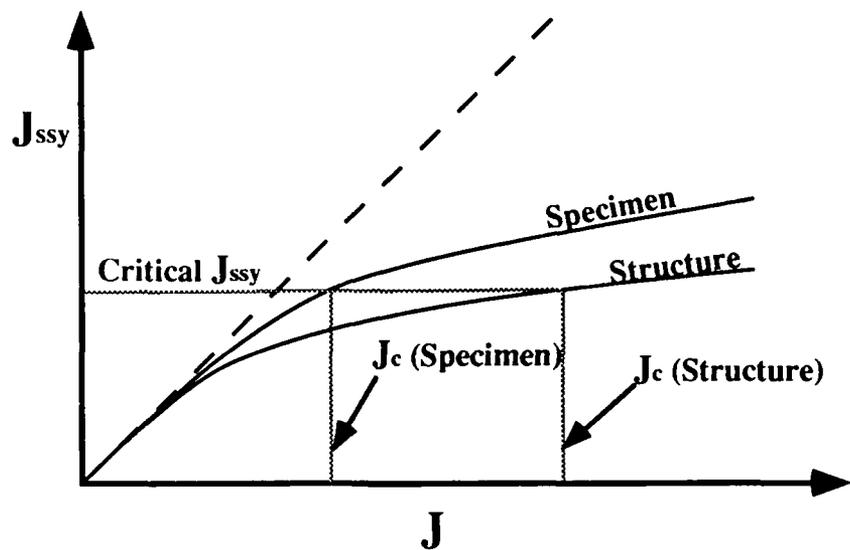
FIGURE 3.24 Correlation of  $J_c$  values for a structure and a test specimen.
