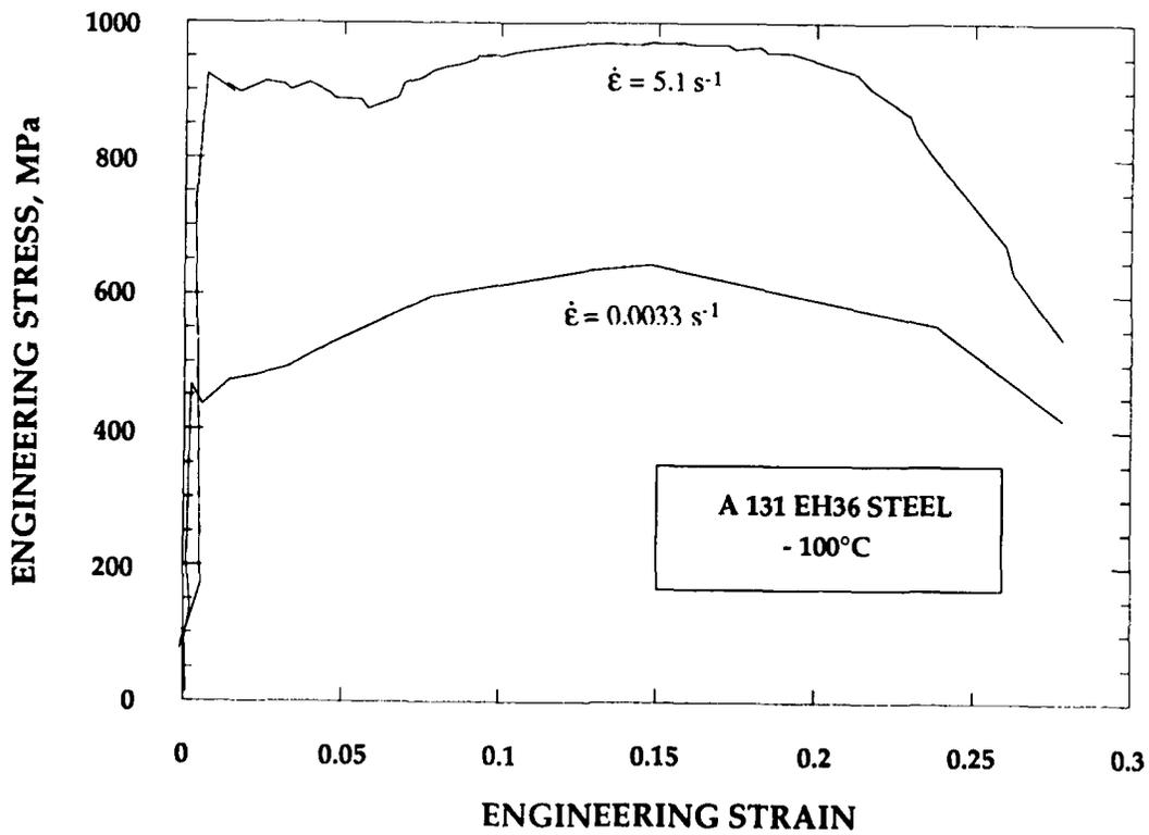
FIGURE 2.9 Effect of strain rate on flow behavior of A131 EH36 steel at -100°C.
