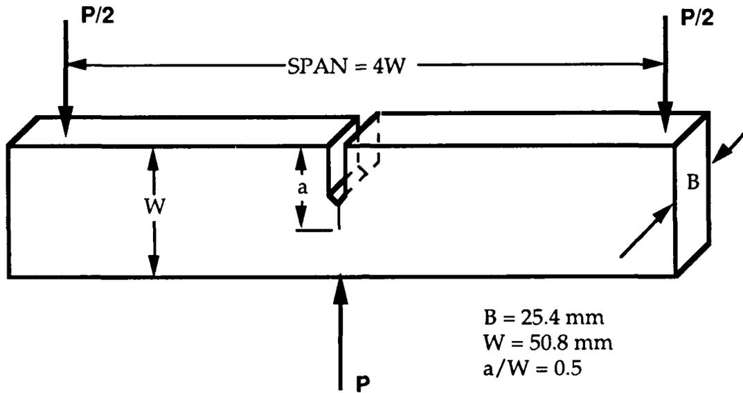
(a) A 131 EH36 steel specimens (L-T orientation).
