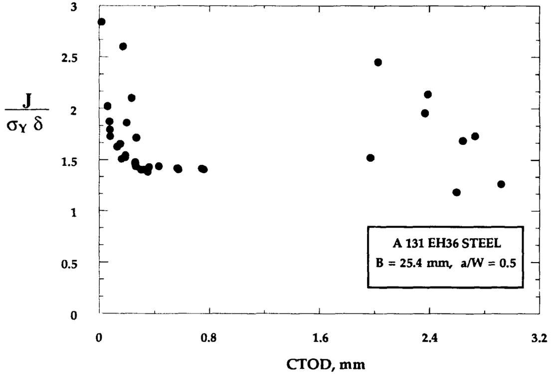
FIGURE 4.7 Experimental J-CTOD ratio for the A 131 EH36 steel.
