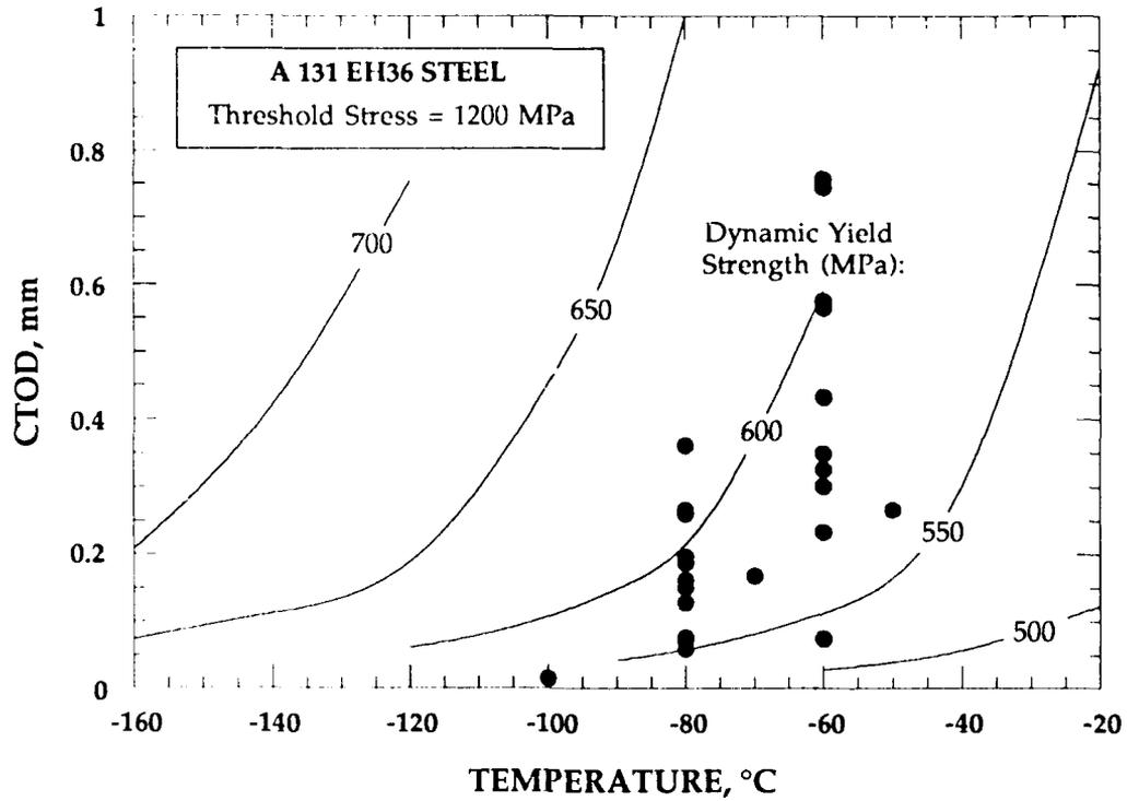
FIGURE 4.17 Effect of the dynamic yield strength on predicted CTOD in the A 131 EH 36 steel.
