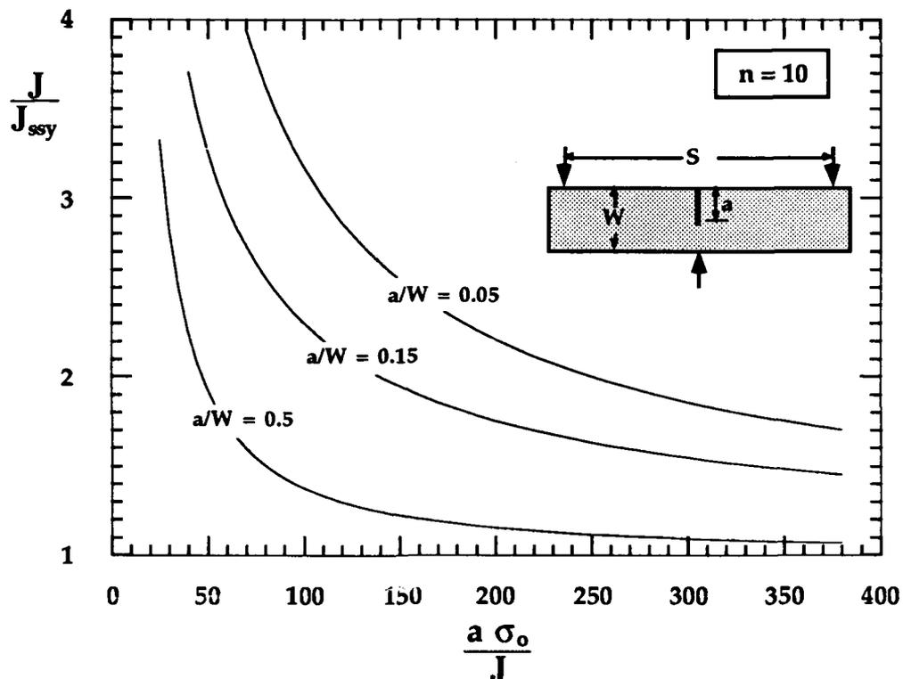
FIGURE 3.11 Effect of crack length and  $a/W$  on the  $J/J_{ssy}$  ratio for  $n = 10$ .
