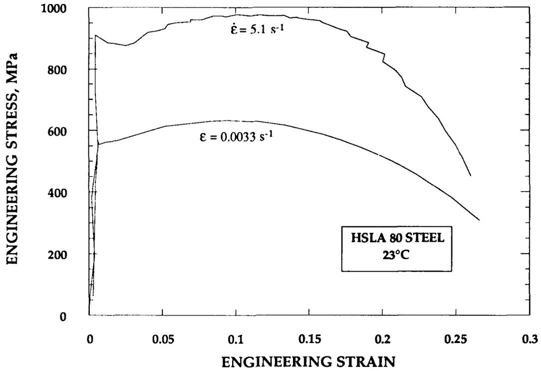
FIGURE 2.10 Effect of strain rate on flow behavior of HSLA 80 steel at 23°C.
