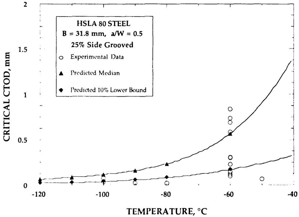
FIGURE 4.14 Predicted and experimental CTOD values for HSLA 80 steel.
