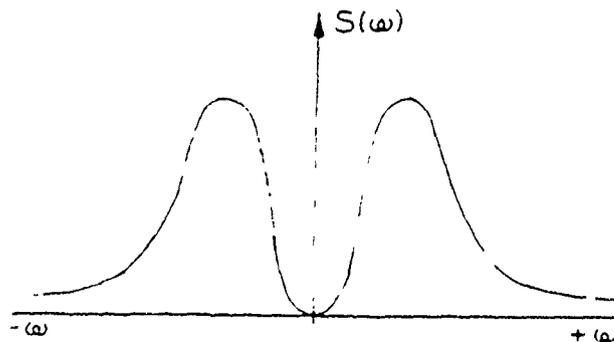
Figure 2.8. Two-sided Spectral Density.
