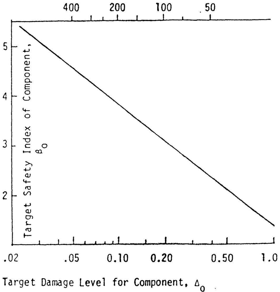
FIG. 9.10 EXAMPLE: THE TARGET SAFETY INDEX AS A FUNCTION OF THE TARGET DAMAGE LEVEL FOR A COMPONENT
