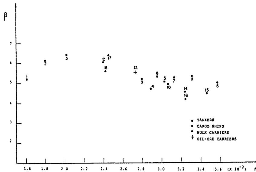
Figure 5.9. Safety Index  $\beta$  for Eighteen Ships
