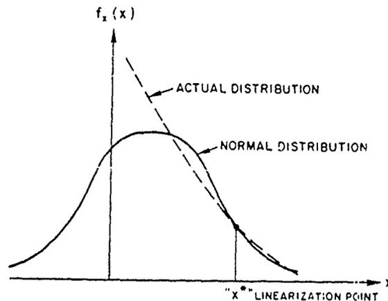
Figure 5.2. Equivalent Normal Distribution at Linearization Point
