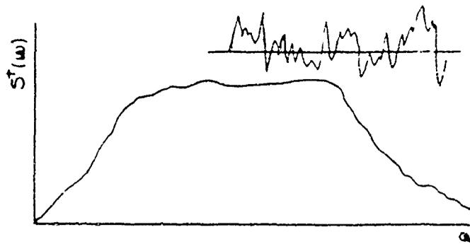
Figure 2.11. Spectrum of a Wide Band Process.
