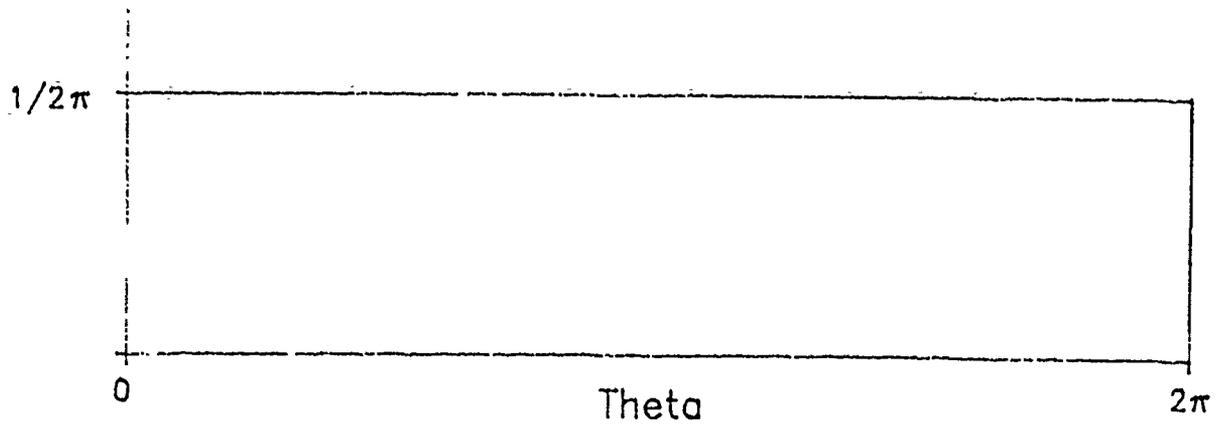
Figure 7.1. Analytically Derived PDF of Theta
