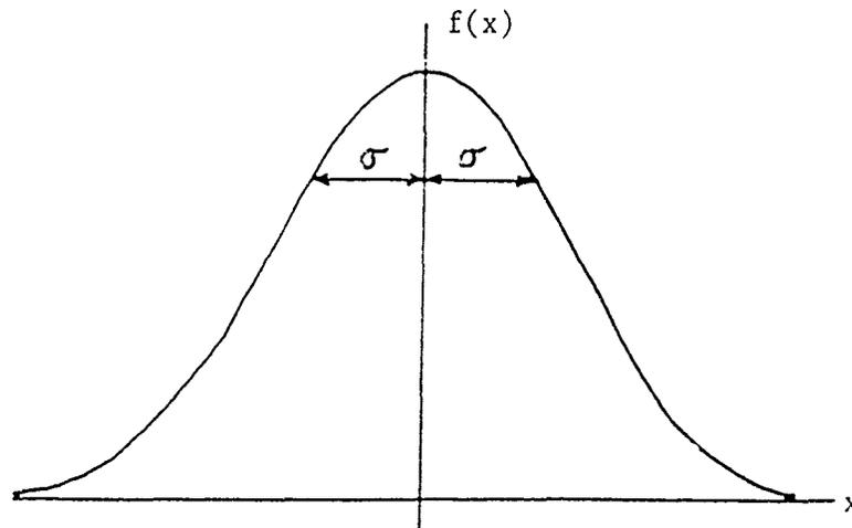
Figure 2.13. Probability Density Function of Wave Elevation
