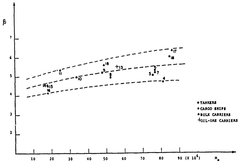
Figure 5.8. Safety Index  $\beta$  for Fifteen Ships
