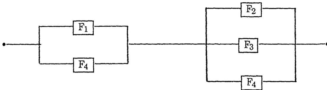
Figure 8.3. Schematic Representation of Parallel Subsystems Connected in a Series (Minimal Cut Set)
