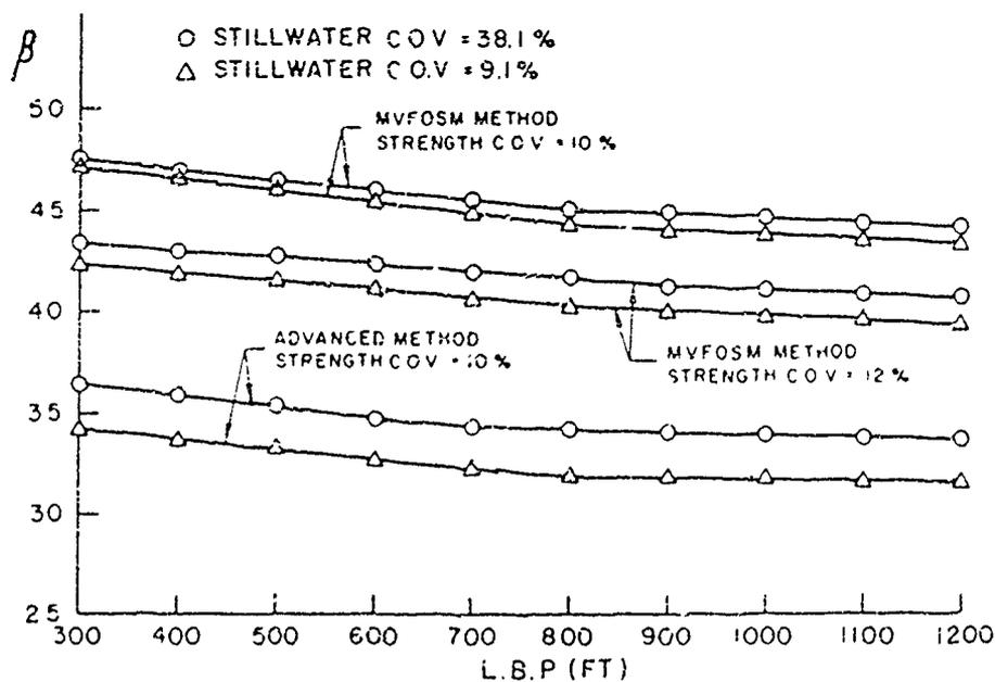
Figure 10.13. Safety Index (ABS) versus length between perpendiculars of Ships
