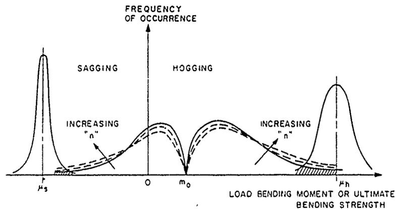
Figure 4.3. Probability of failure under extreme bending moment
