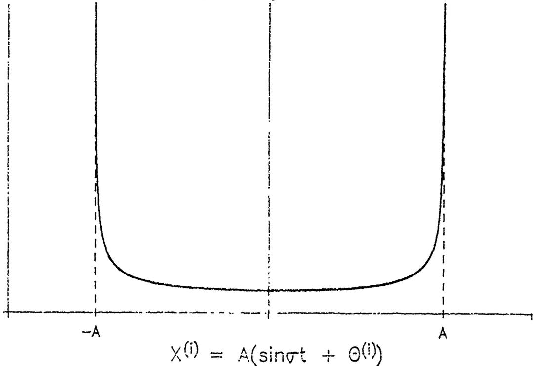
Figure 7.2. Analytically Derived PDF of X
