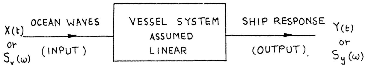
Figure 2.18. Input/Output System.
