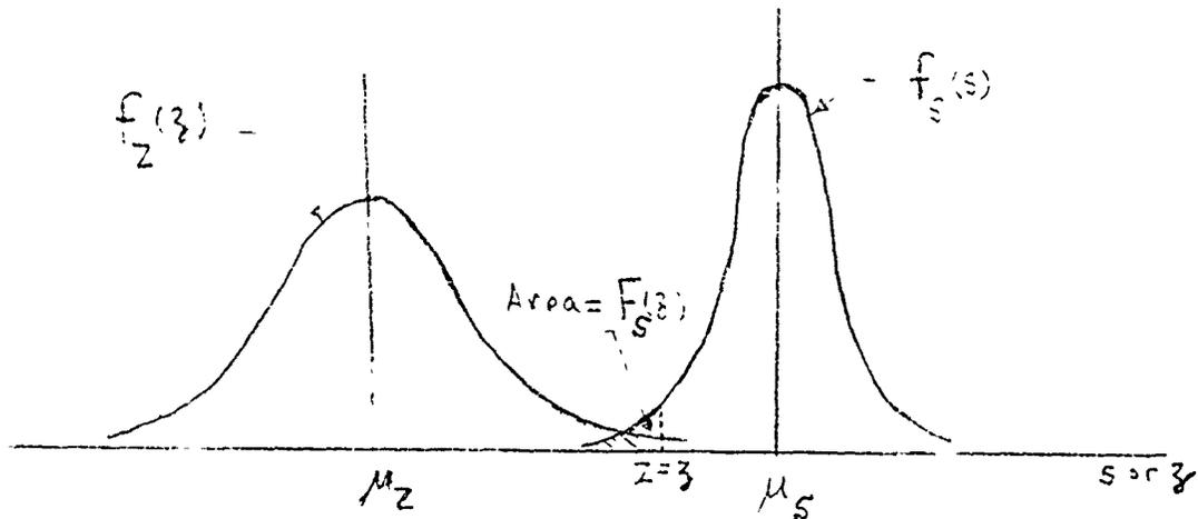
Figure 1.2. Load and Strength Probability Density Functions
