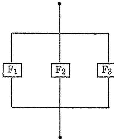
Figure 8.2. Schematic Representation of a Parallel System.
