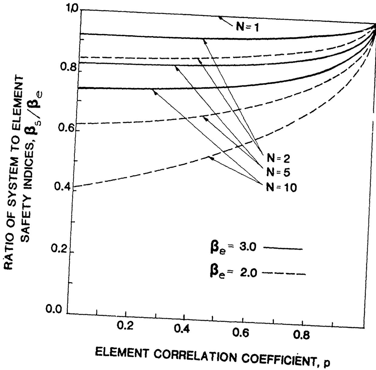
**FIG. 9.13 SAFETY INDICES FOR SERIES SYSTEM OF N ELEMENTS**
