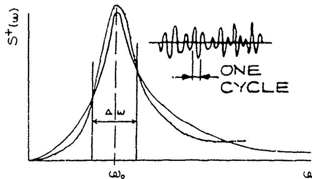
Figure 2.10. Spectrum of a Narrow Band Process
