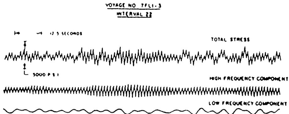
Figure 2.27. Decomposition of a stress time history of a Great Lakes vessel into low and high frequency components.
