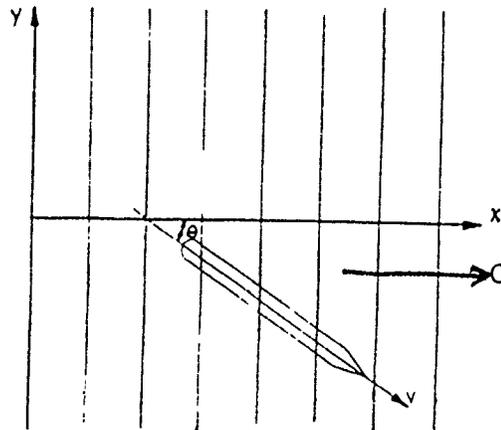
Figure 2.21. Heading Angle in Regular Waves.
