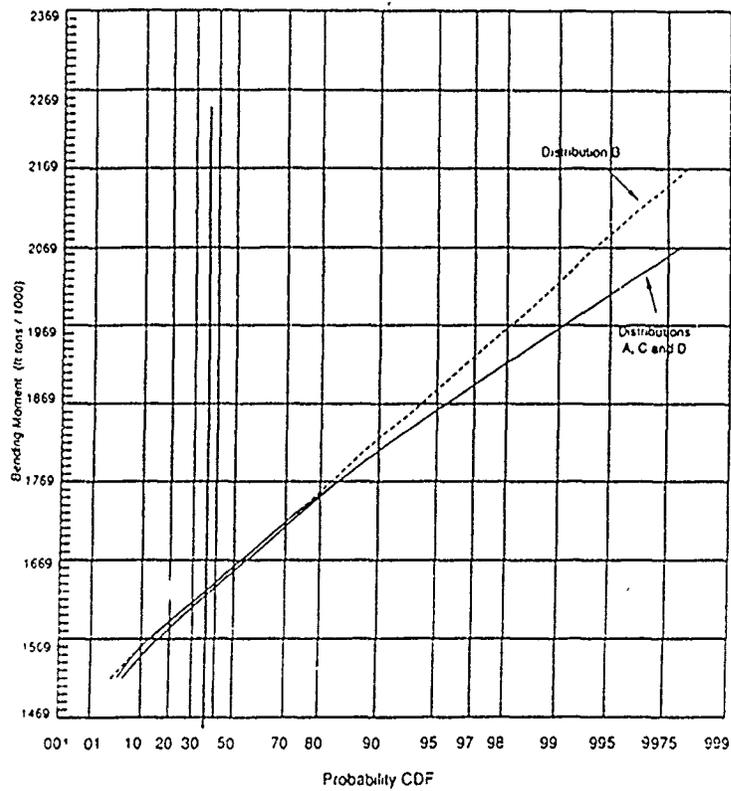
Figure 2.23. Standard Extremal Variate - Bending Moment on a Tanker.
