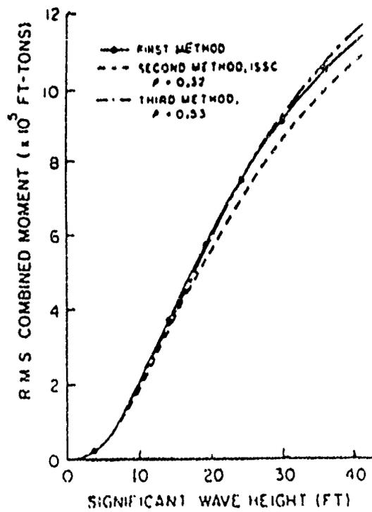
Figure 2.35. Comparison of combined bending moment responses as computed by three methods.
