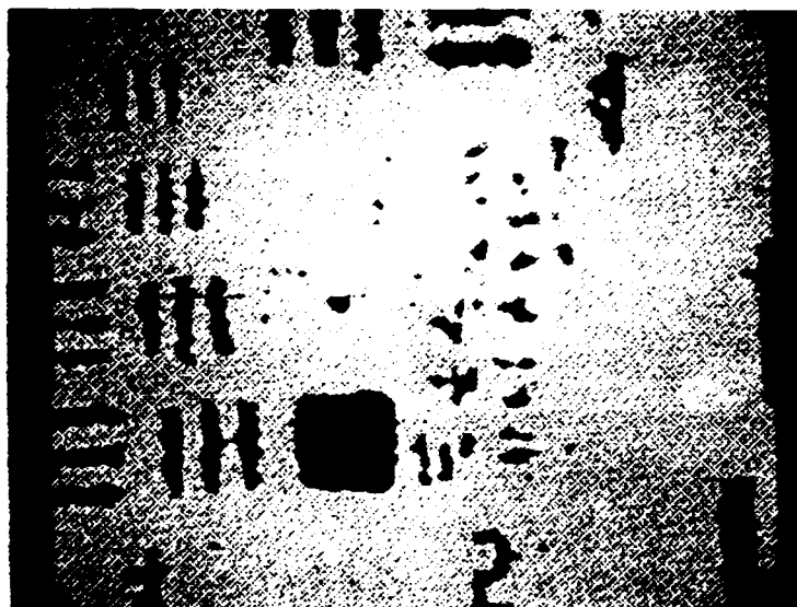
Figure 3.7: Thresholded image after application of Sigma filter. (Threshold value = 140.)
