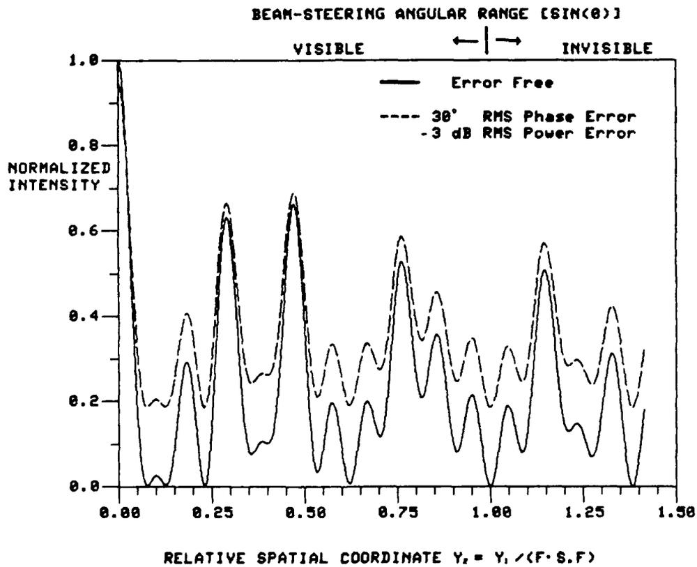
FIGURE 9: NORMALIZED INTENSITY PATTERN OF AN OPTIMUM APERIODIC ARRAY [Base line =  $10.5 \lambda_R$  at 12.5 GHz; Element locations( $\lambda_R$ ): -5.25, -1.54, 0.98, and 5.25,  $H = \ell_N/30$ ]
