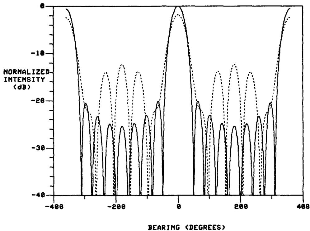
FIGURE 21: NORMALIZED DOA PATTERN OF A RECEIVER USING A CIRCULAR ANTENNA ARRAY FOR  $T_y = 0.88$  and  $H/\ell = 0.2$
