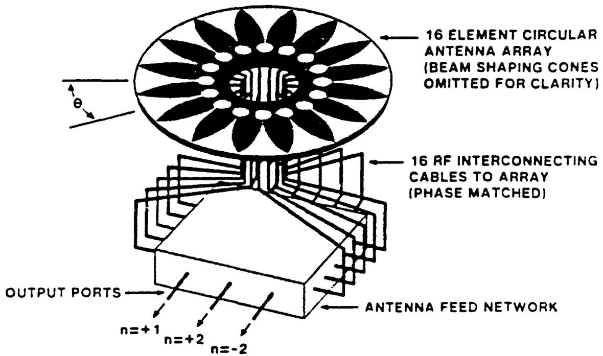
FIGURE 5: CIRCULAR ANTENNA ARRAY AND FEED NETWORK
