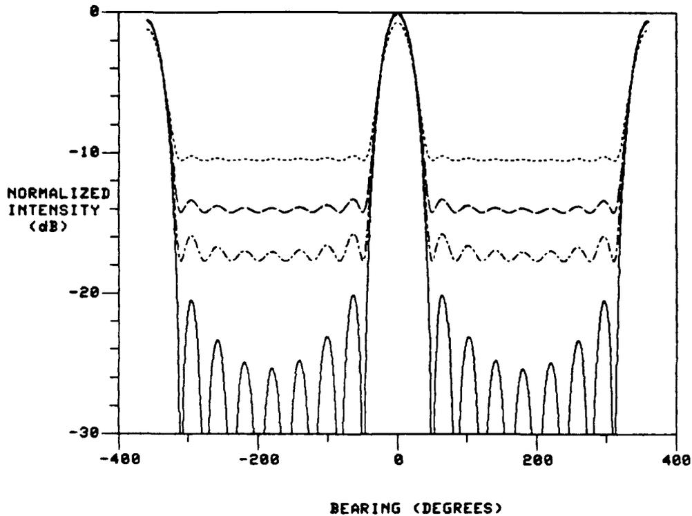
FIGURE 20: NORMALIZED DOA PATTERN OF A 9-CHANNEL RECEIVER USING A CIRCULAR ANTENNA ARRAY FOR OPTIMUM  $T_y = 0.88$  and  $H/\ell = 0.2$
