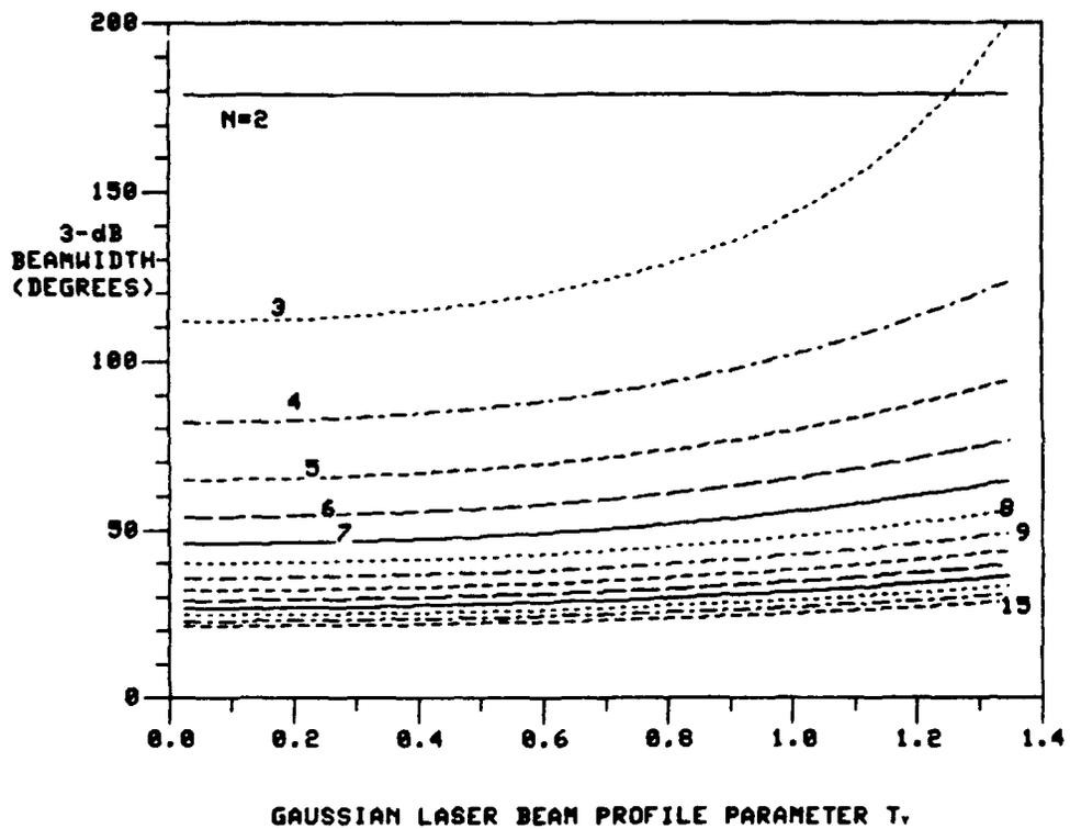
FIGURE 15: 3-dB BEAMWIDTH VERSUS  $T_y$  FOR A N-CHANNEL RECEIVER USING A CIRCULAR ANTENNA ARRAY ( $H/\ell = 0.2$ )
