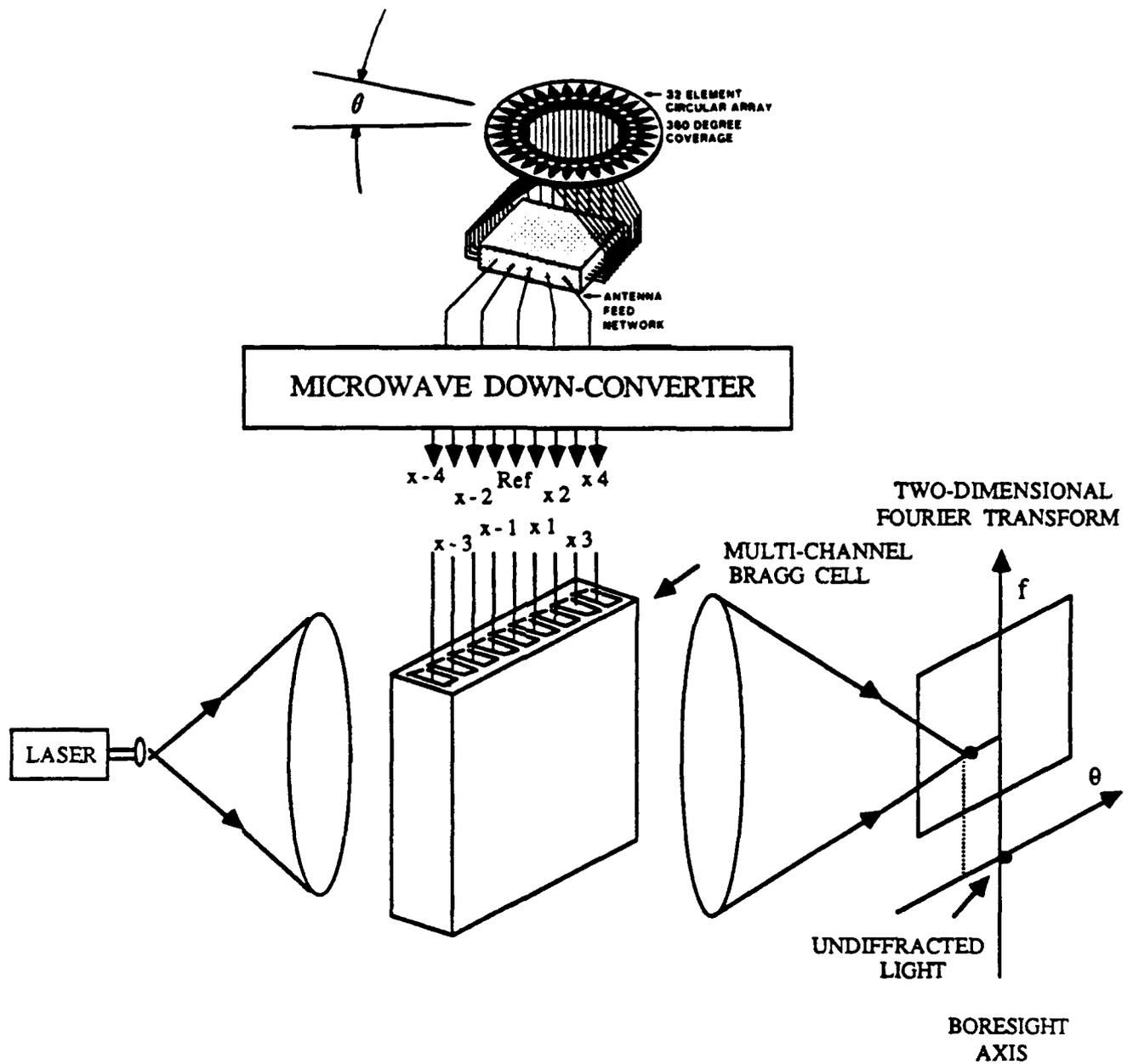
FIGURE 7: TWO-DIMENSIONAL ACOUSTOOPTIC RECEIVER USING A CIRCULAR ANTENNA ARRAY AND A BUTLER MATRIX
