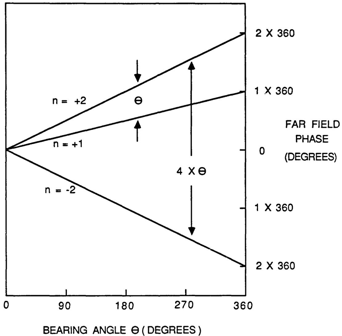
FIGURE 6: PHASE IN THE FAR FIELD VERSUS BEARING ANGLE
