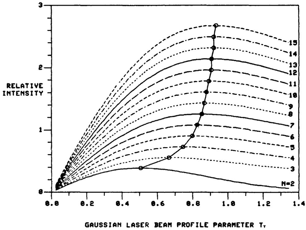
FIGURE 14: RELATIVE PEAK INTENSITY OF DOA PATTERN VERSUS  $T_y$  FOR A N-CHANNEL RECEIVER USING A CIRCULAR ANTENNA ARRAY ( $H/\ell = 0.2$ )
