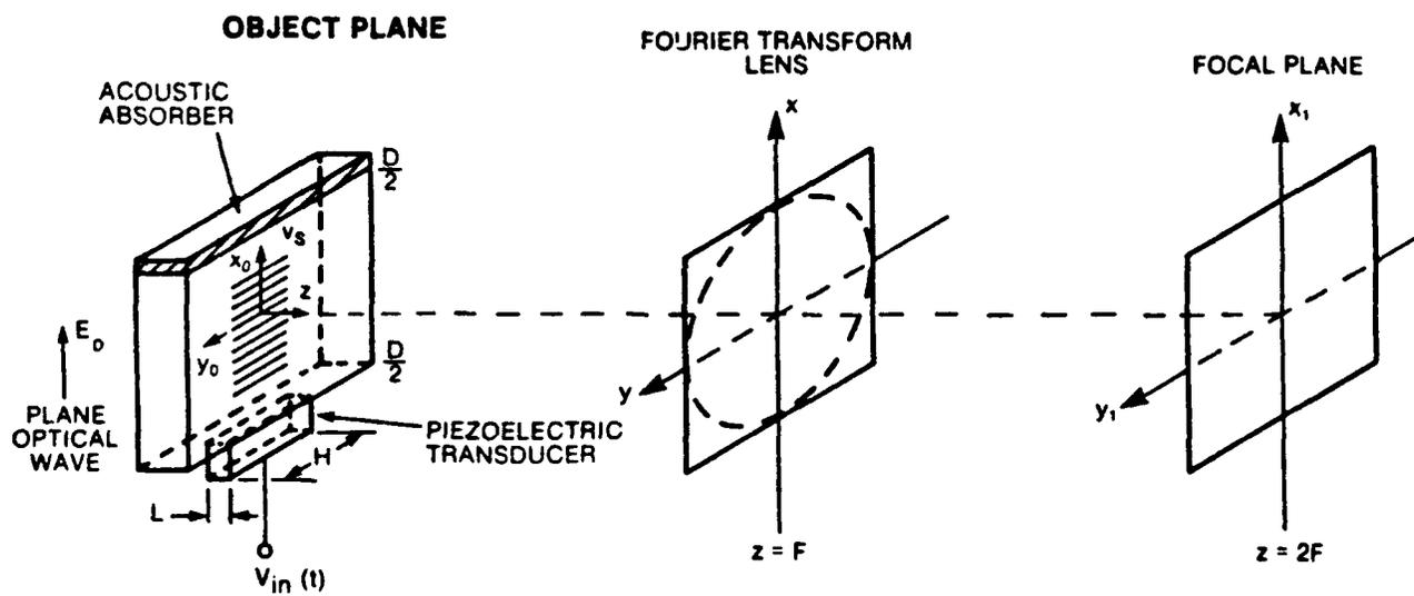
FIGURE 2: FOURIER TRANSFORMING CONFIGURATION
