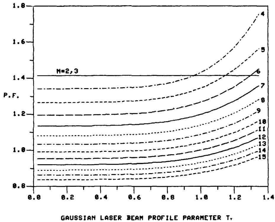
FIGURE 18: P.F. VERSUS  $T_y$  FOR A N-CHANNEL RECEIVER USING A CIRCULAR ANTENNA ARRAY ( $H/\ell = 0.2$ )
