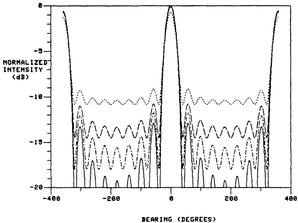
FIGURE 19: NORMALIZED DOA PATTERN OF A 9-CHANNEL RECEIVER USING A CIRCULAR ANTENNA ARRAY FOR
