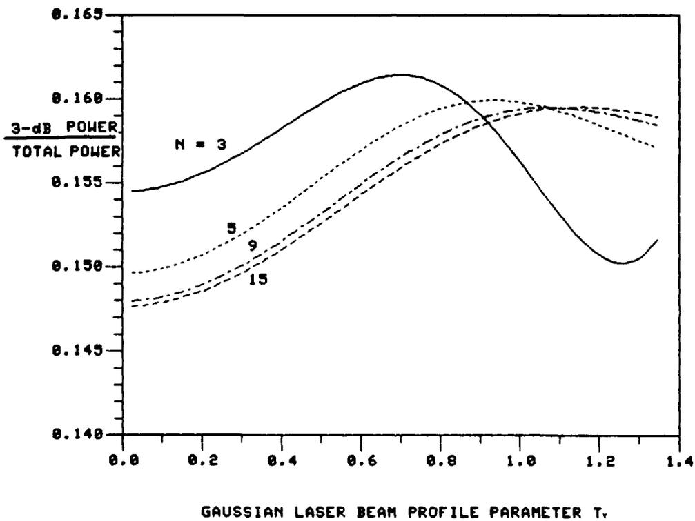
FIGURE 17: RATIO OF 3-dB BEAMWIDTH POWER TO TOTAL POWER VERSUS  $T_y$  FOR A N-CHANNEL RECEIVER USING A CIRCULAR ANTENNA ARRAY ( $H/\ell = 0.2$ )
