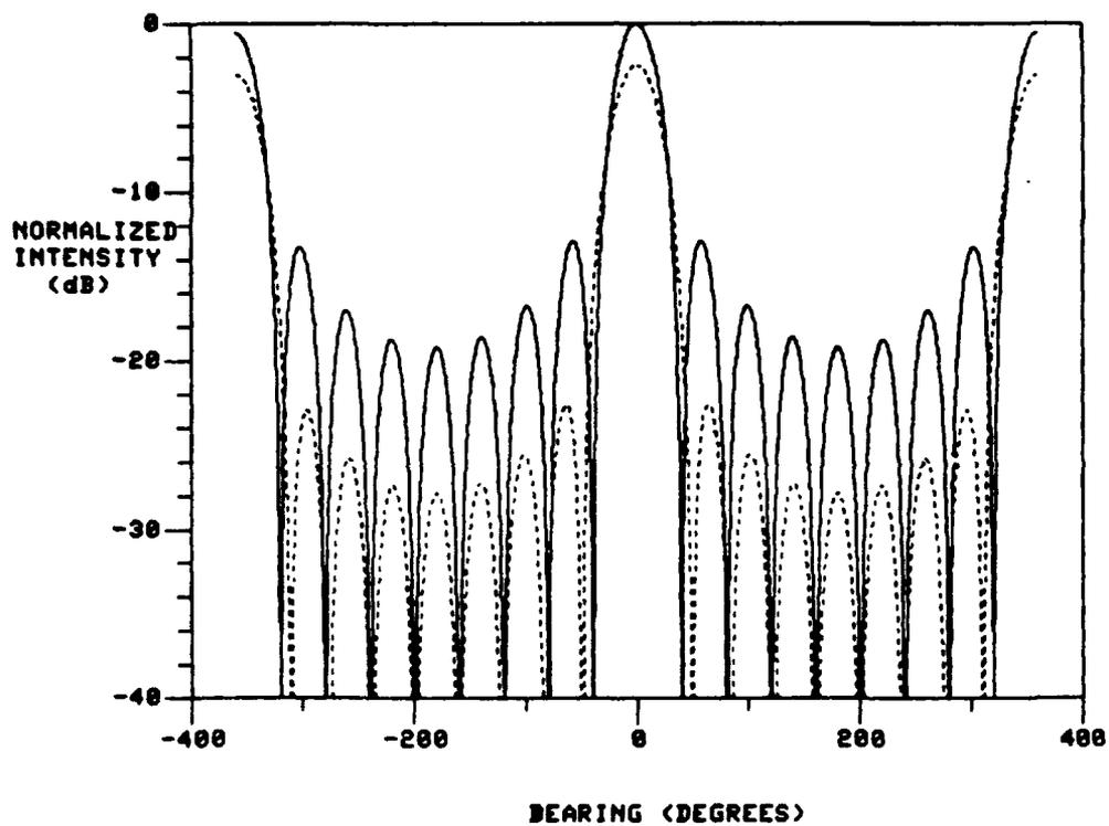
FIGURE 12: NORMALIZED DOA PATTERN OF A 9-CHANNEL RECEIVER USING A CIRCULAR ANTENNA ARRAY
