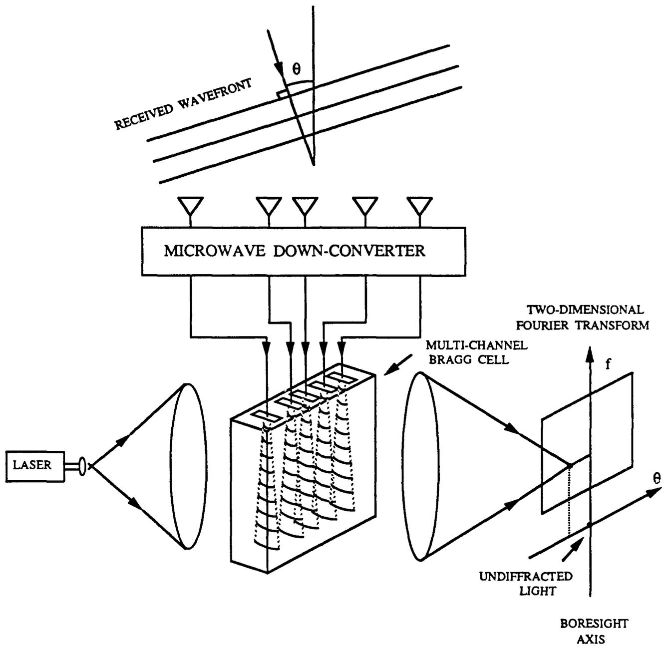
FIGURE 1: TWO-DIMENSIONAL ACOUSTO-OPTIC FOURIER TRANSFORMING SIGNAL PROCESSOR
