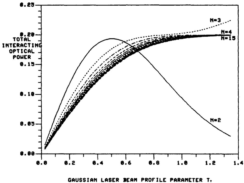
FIGURE 13: TOTAL INTERACTING OPTICAL POWER VERSUS  $T_y$  FOR A N-CHANNEL RECEIVER USING A CIRCULAR ANTENNA ARRAY ( $H/\ell = 0.2$ )
