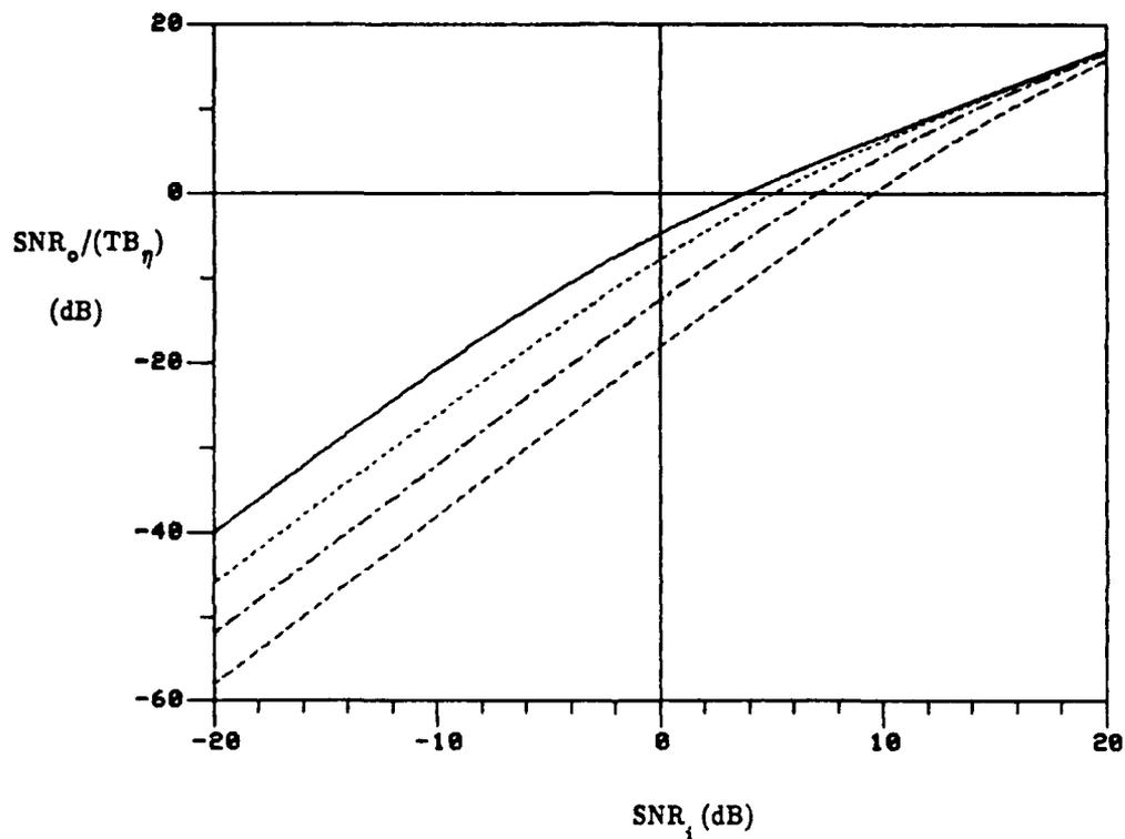
FIGURE 8: NORMALIZED OUTPUT SIGNAL-TO-NOISE RATIO VERSUS INPUT SIGNAL-TO-NOISE RATIO
