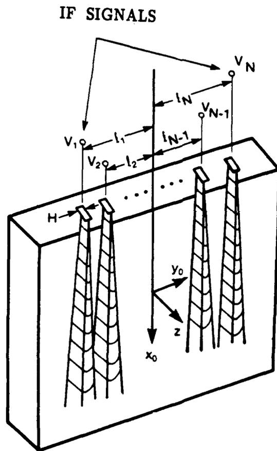
FIGURE 4: MULTI-CHANNEL BRAGG CELL CONFIGURATION
