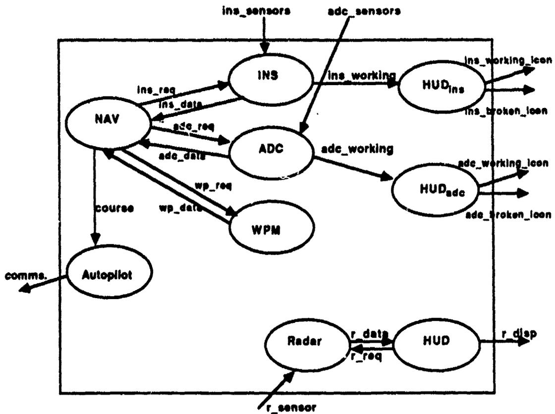
Figure 8.1: Processes in Temporal Logic Specification
