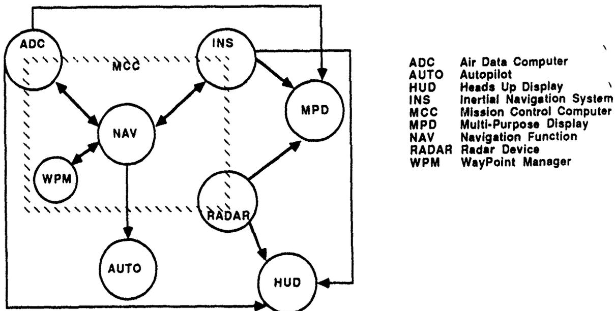
Figure 5.1: Avionics System to Be Specified
