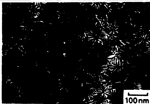
Figure 4. Chrysanthemum pattern in TEM of etched 18% Cr films. Courtesy of Y. Maeda and M. Takahashi (from Ref 49).
