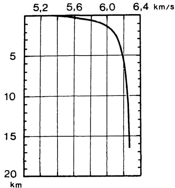
Fig. 8.10. P wave velocity versus depth for a medium granite after *BIRCH (1958)* according to a temperature gradient of 8 °C/km.
