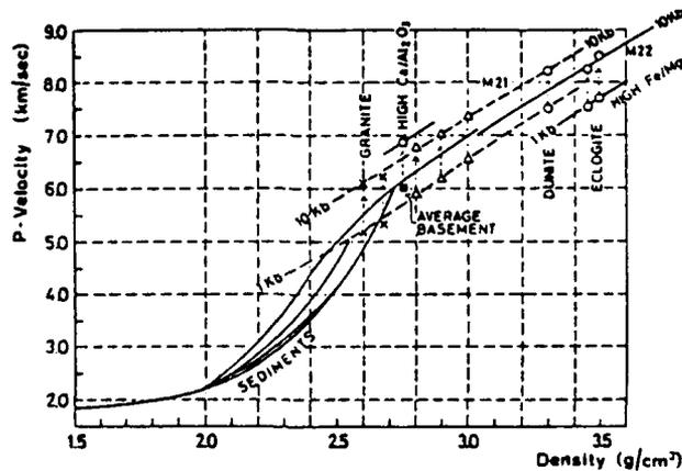
Fig. 3.14. Experimental velocity-density systematics after *WOOLLARD (1975)*.
