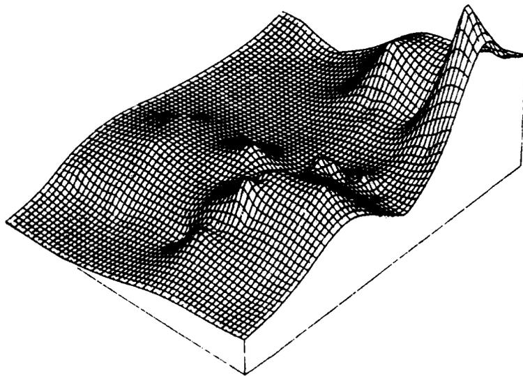
Fig. 8.2. Orthometric heights in test network "Rossdorf".
