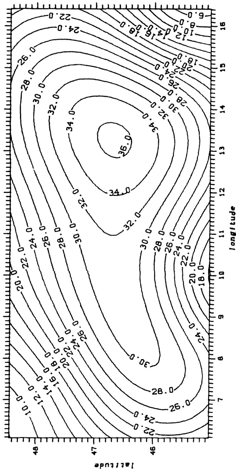
Fig. 3.8c. Gravity effect [mGal] of the variation of the lithosphere/asthenosphere boundary due to a density contrast of  $+0.029 \text{ g/cm}^3$ , in relationship to a normal lithospheric thickness of 105 km.
