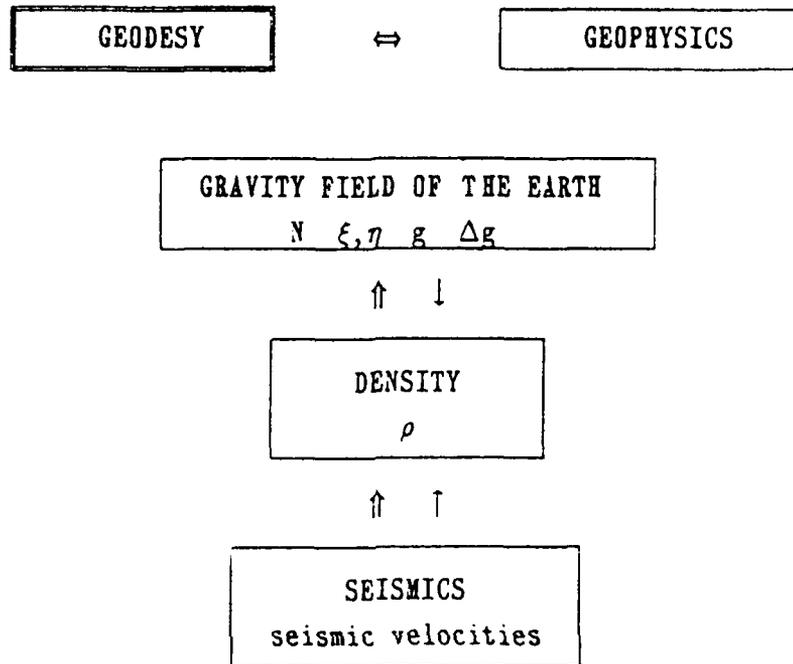
Fig. 2.1. Gravity, density, and seismic data in geodesy and geophysics (the corresponding arrows indicate the main goals and working directions of geodesy ( $\Rightarrow$ ) and geophysics ( $\rightarrow$ )).
