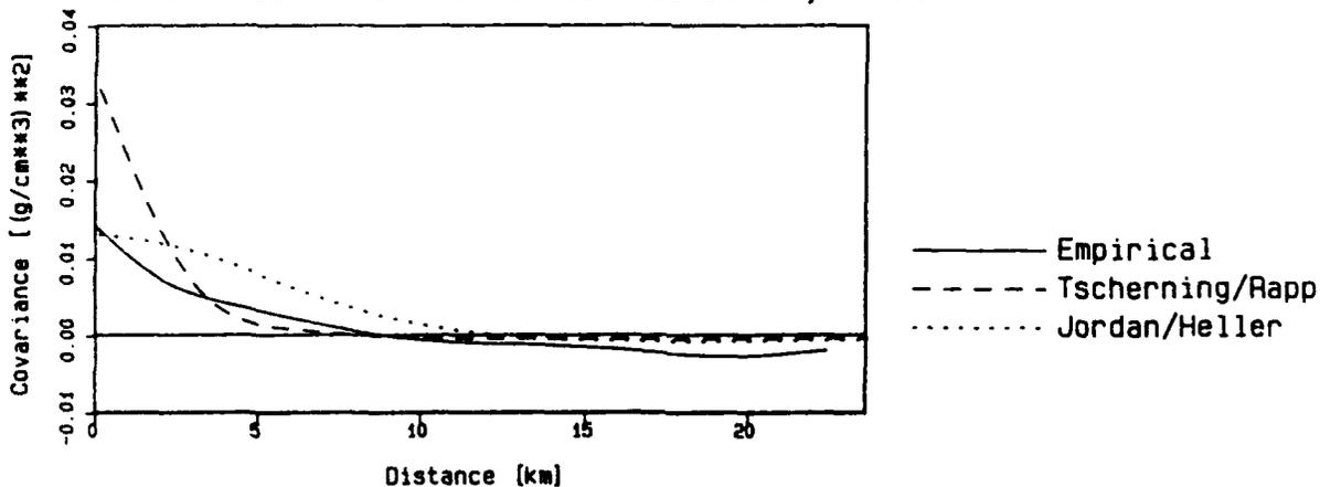
Fig. 9.2. Covariance functions for the test area "Rossdorf" (Bouguer gravity anomaly fit).
