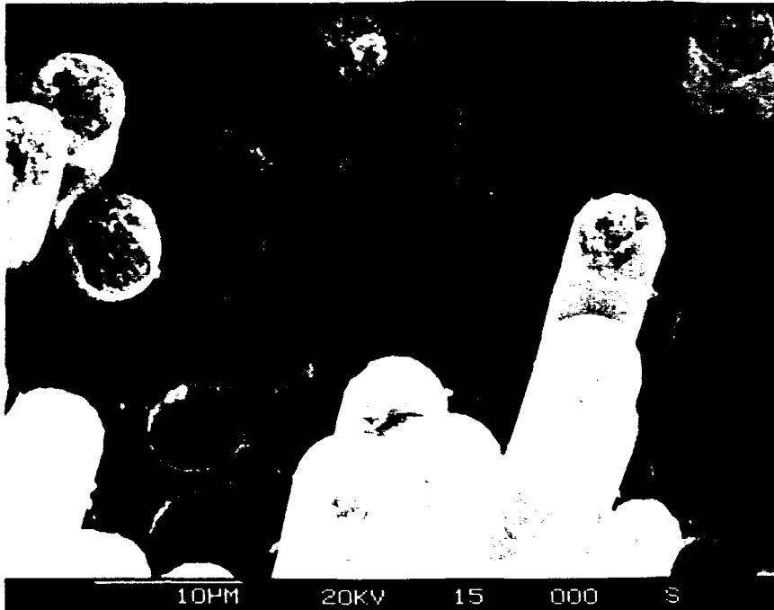
(b) 90/0 carbon/bismaleimide, predominantly pullout of individual fibers.
