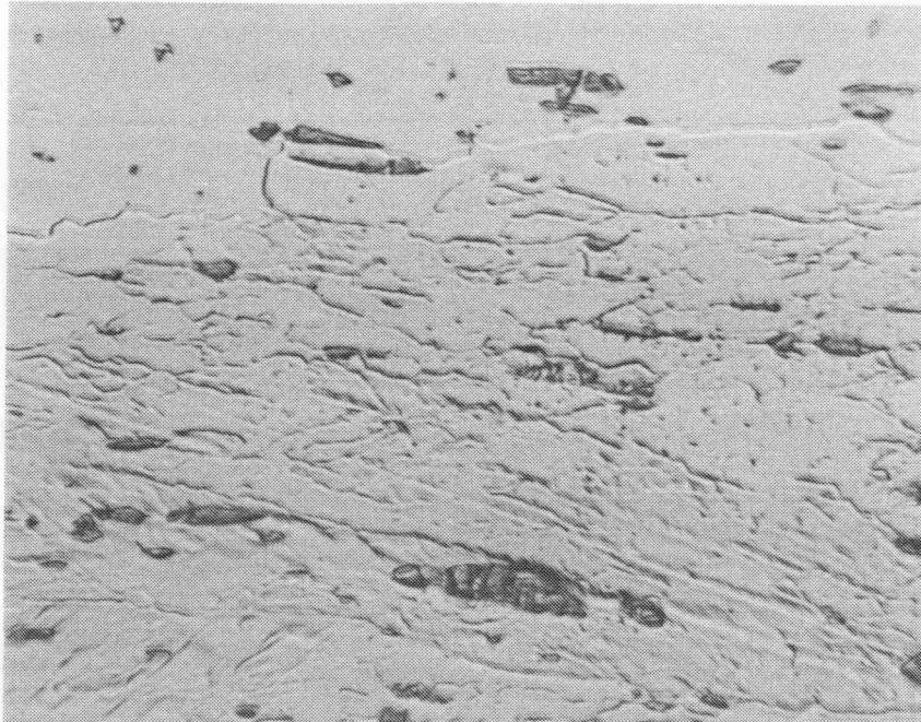
Figure 3 Longitudinal cross section from 30 mm diameter thoria-tungsten bar. Thoria particles and W grains are elongated due to unidirectional processing.
