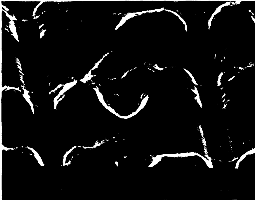
Figure E-11. Typical Vendor 2 Memory Cell at Top Passivation Layer (SEM 5000X)
