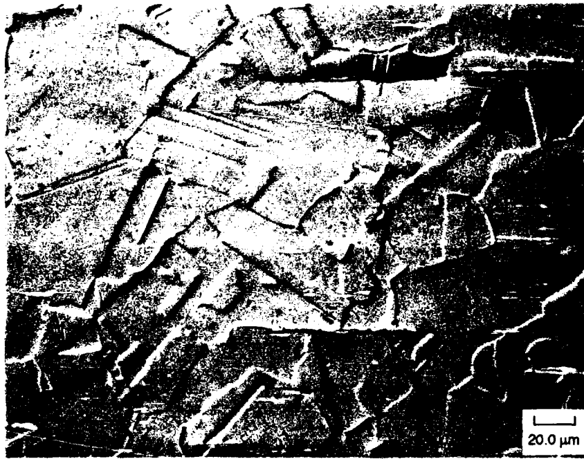
Figure 1.—Microstructure of as-received type 316 stainless steel.
