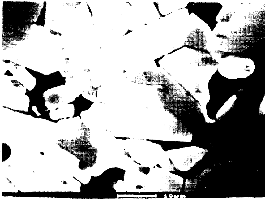
Figure 4. Scanning electron micrograph of polished cross-section of sample sintered at 950°C.
