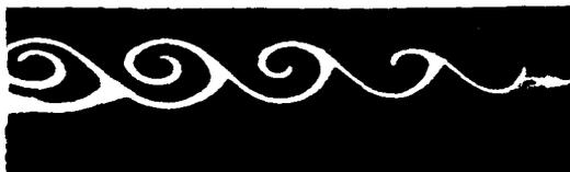
Figure 8. Single Scan of Vortice Formation After Splitter Plate (air flow right to left).
