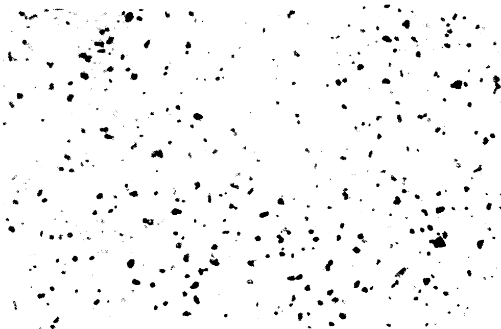
Figure 38. Optical micrograph of the guide tube showing no abnormalities within the microstructure of the 3003 drawn aluminum alloy. MAG 500X
