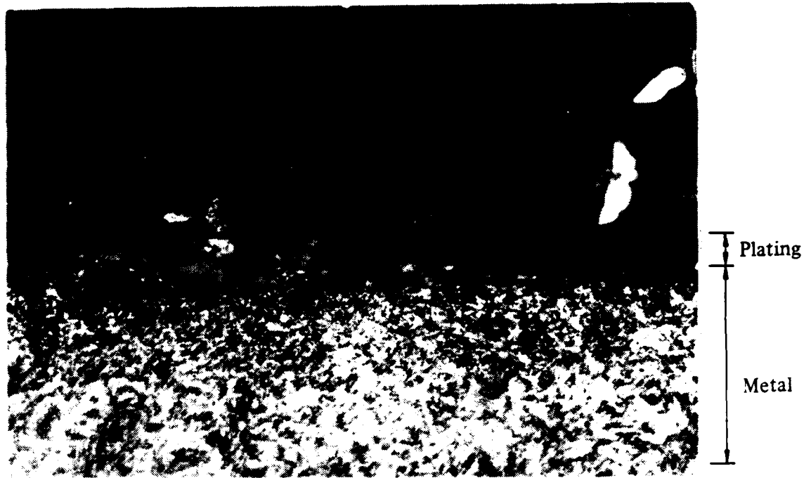
Figure 42. Optical micrograph of the setscrew revealing a plating thickness of 0.0005 inch. MAG 800X
