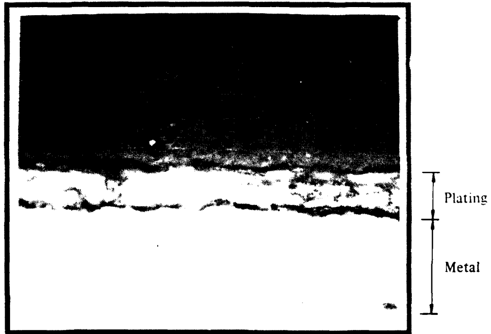
Figure 41. Optical micrograph of the self-locking nut revealing a plating thickness of 0.001 inch. MAG 500X
