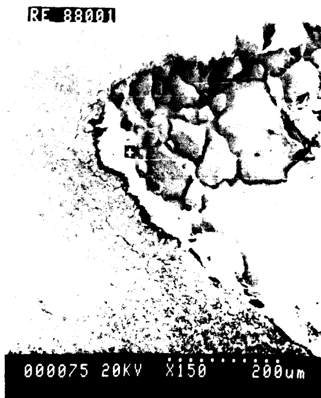
Figure 45. Degradation in Throat Region
