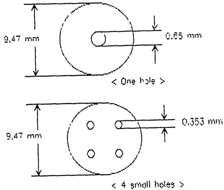
Figure 7. Faraday Cup Cover Hole, Schematic
