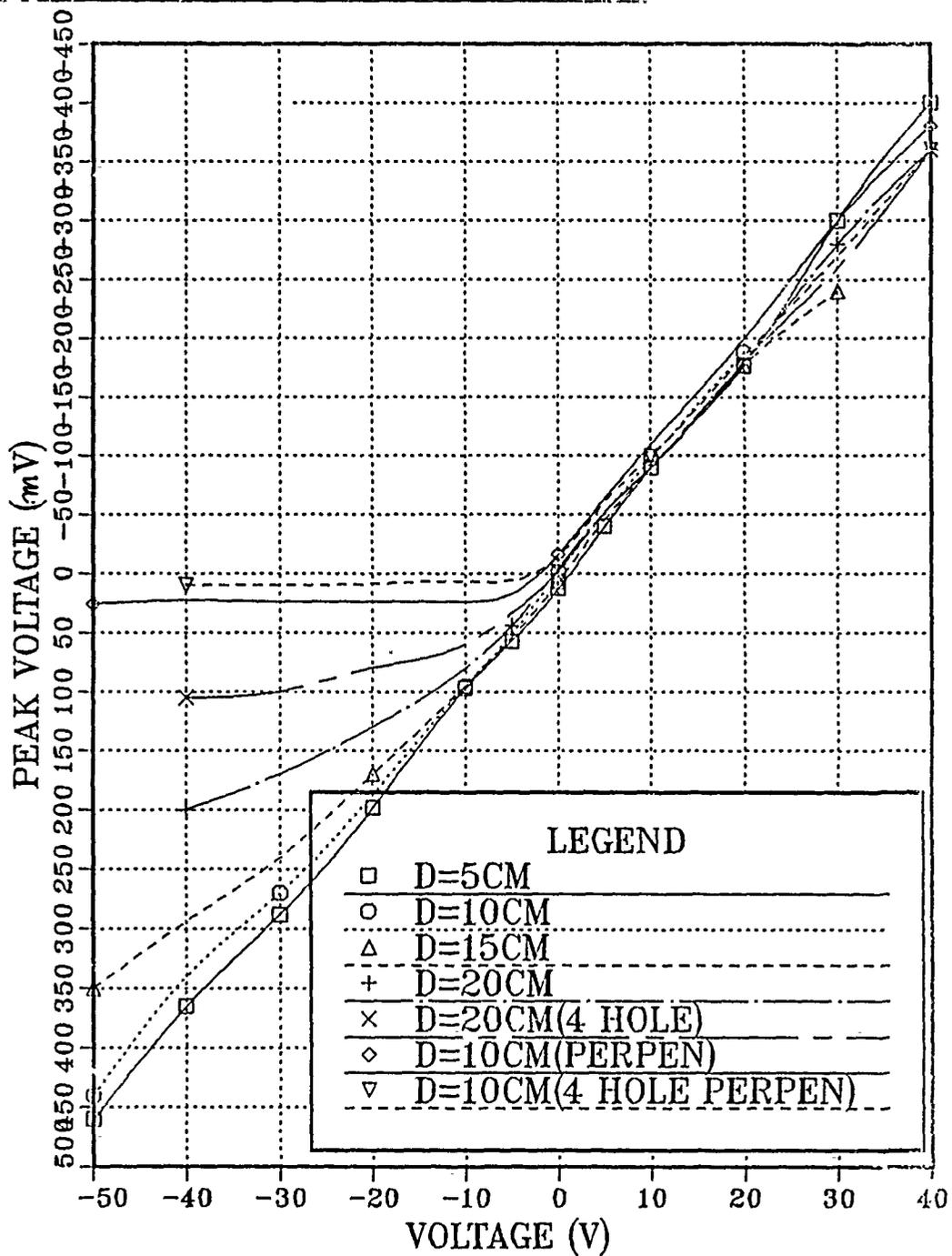
Figure 15. Peak Voltage vs Bias Voltage at Variable Distance ( Normal Faraday Cup)
