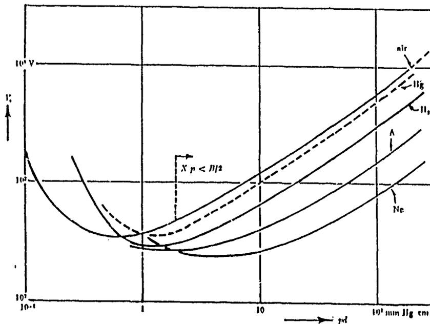
Figure 12. Sparking Potential (V) as a Function of The Reduced Electrode Distance Pd in Several Gases [Ref.14]
