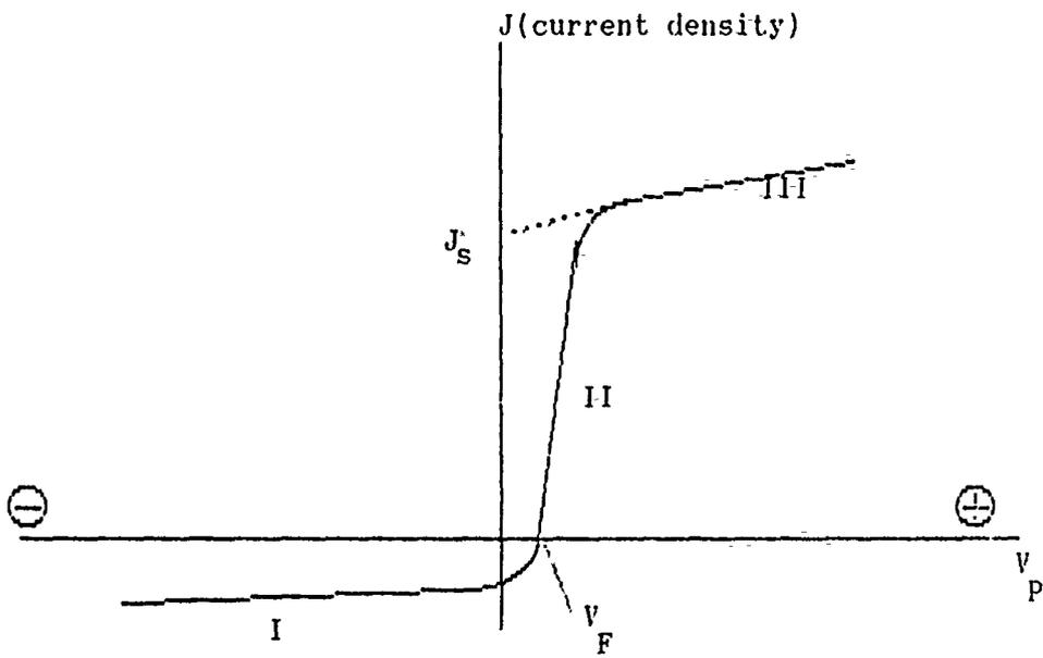
Figure 41. V-I Characteristics of Single Langmuir Probe
