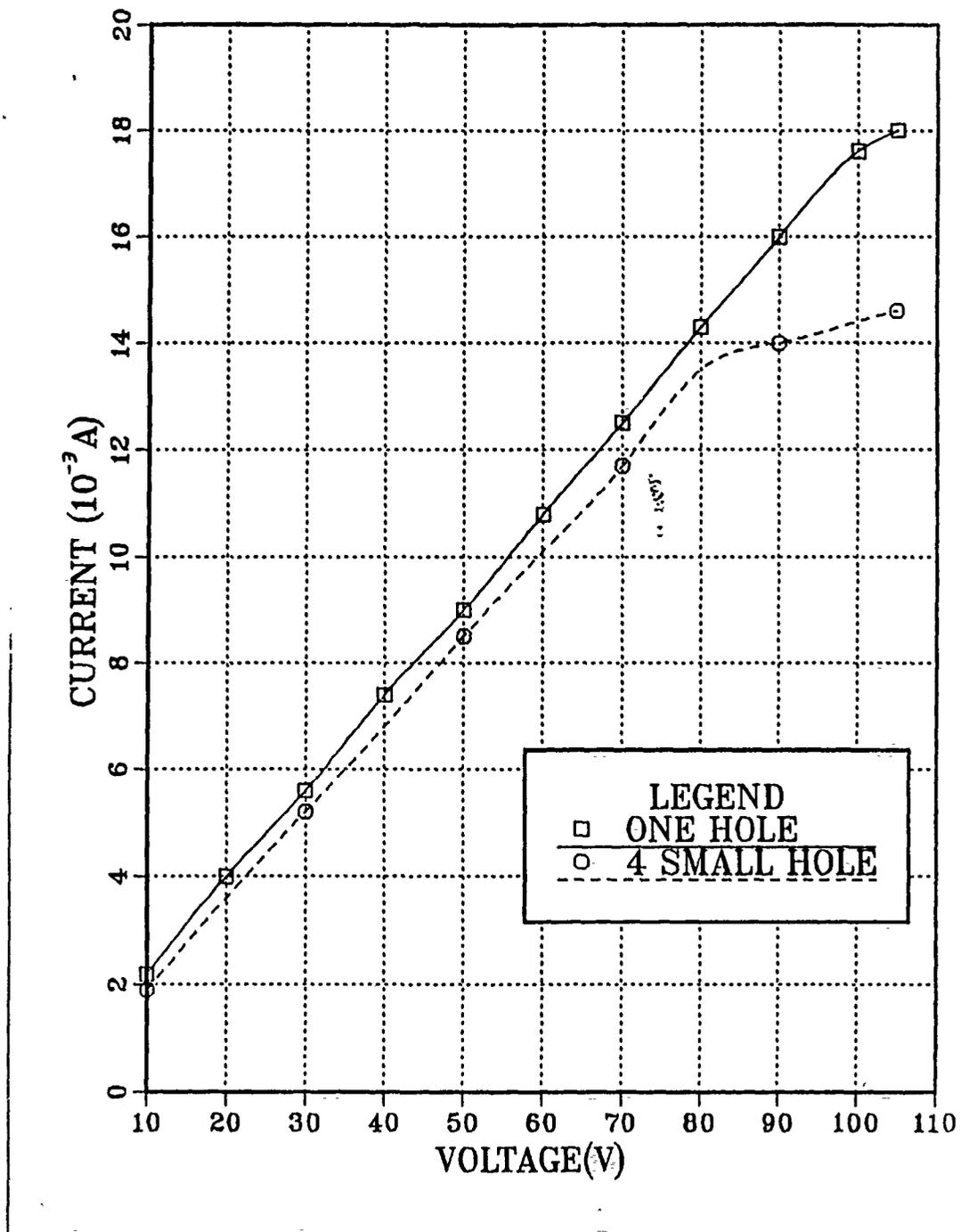
Figure 39. Current vs Bias Voltage (0 V to +105 V), Distance  $d=10$ cm
