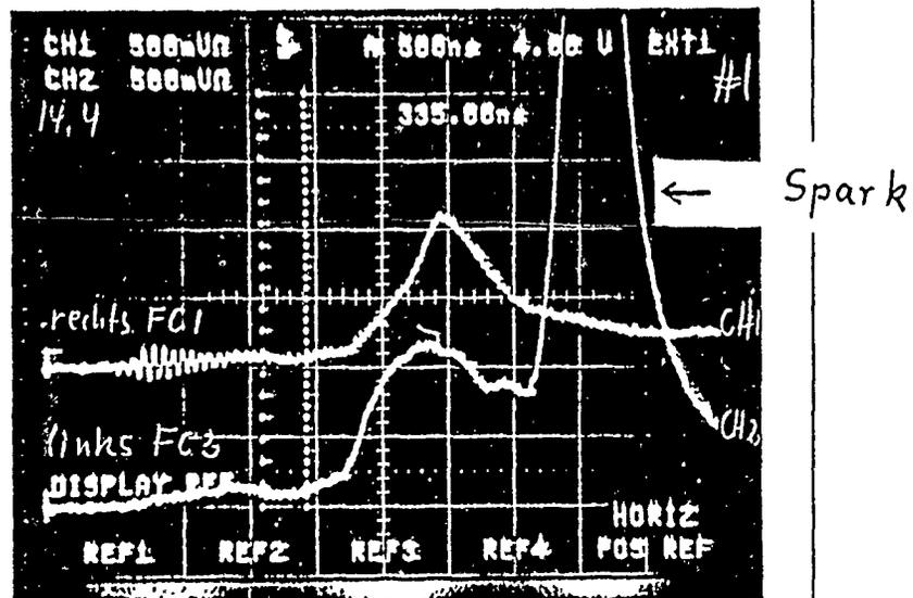
Figure 8. Comparison of Current Signals of Two Faraday Cups FC1 with 0.3 mm Entrance Hole and FC3 with 0.5 mm Hole. Bias  $V = -25$  Volt
