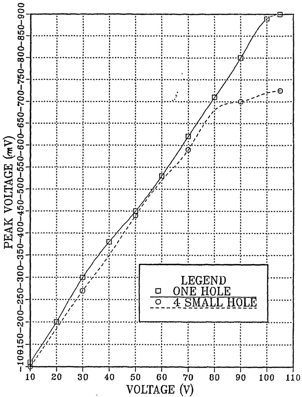
Figure 38. Peak Voltage vs Bias Voltage (0 v to + 105 V ), Distance d= 10cm
