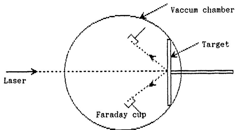
Figure 22. Perpendicular Orientation of Faraday Cup
