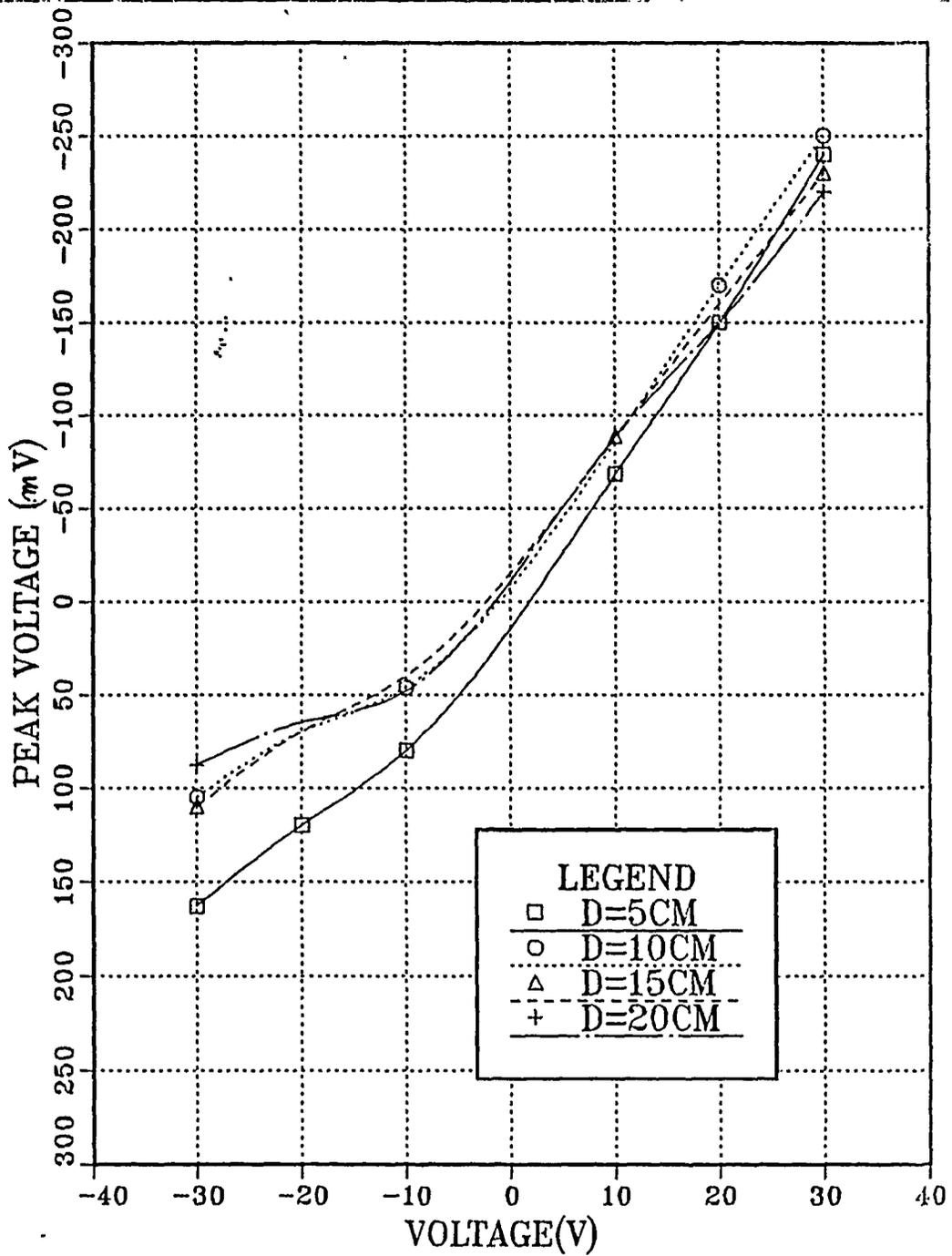
Figure 28. Peak Voltage vs Bias Voltage at Variable Distance (Soldered Faraday Cup)
