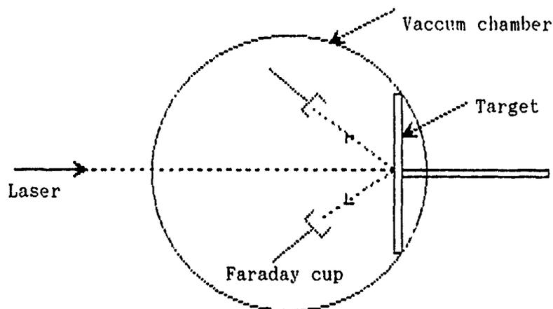
Figure 16. Parallel Orientation of Faraday Cup
