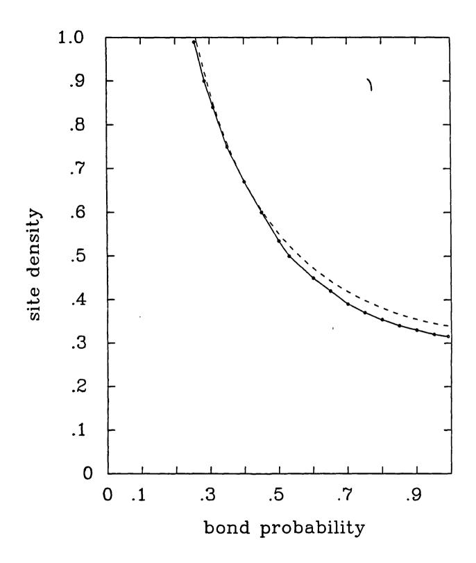
RANDOM SITE BOND PERCOLATION 3D SC lattice solid curve - SIMULATION broken curve - MSA @ PLOC
