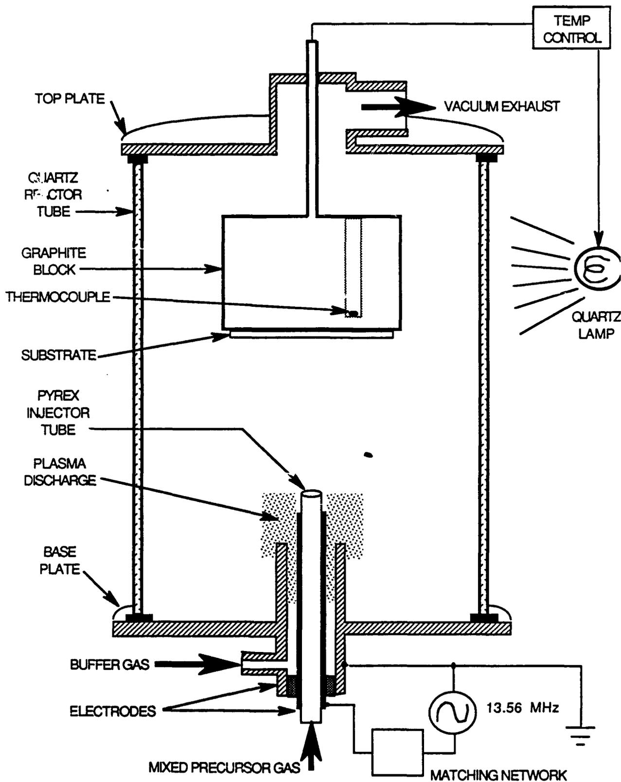
Figure 1. Deposition reactor chamber in test PEMOCVD set-up.
