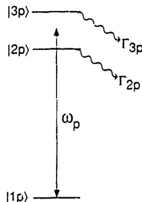
Fig. 1. Prototype system for inversion-free lasers.  $\Gamma_{2p}$  and  $\Gamma_{3p}$  are the decay rates, to the same continuum, of prototype states |2p> and |3p>.
