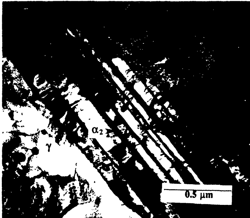
Fig. 12. Transmission electron micrograph of laminated alpha-two and gamma phases in TiAl region.
