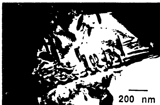
Fig. 18. Sample 158 (AR) annealed at 650 °C for 100 h. The decomposing \text{Ni}_2\text{Mo} ordered phase exists near the grain boundary where several ledges are seen.
