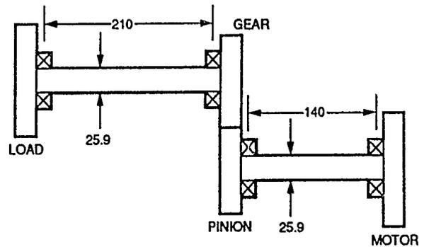
Figure 4. - The system of the second example. (Dimensions are in millimeters.)
