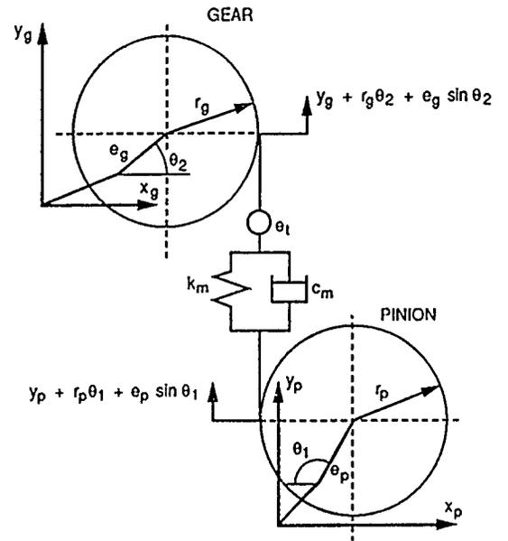
Figure 2. - Modeling of a gear mesh.
