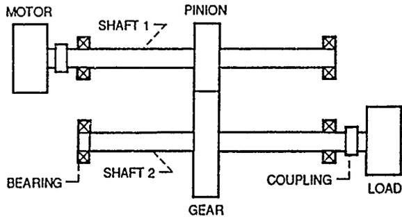
Figure 1. - A typical gear-rotor system.
