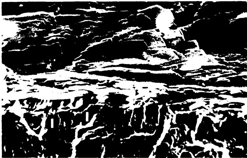
B. Fatigue crack initiation beneath the coating. Coating is in upper two-thirds of field of view, fatigue crack surface is in lower third. Intergranular facets are indicated by I. SEM X500
