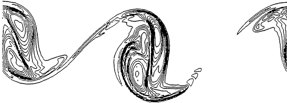
Fig. (4) Vorticity contours at  $t = 83.2 (\delta/U_0)$ , two-dimensional simulation.
