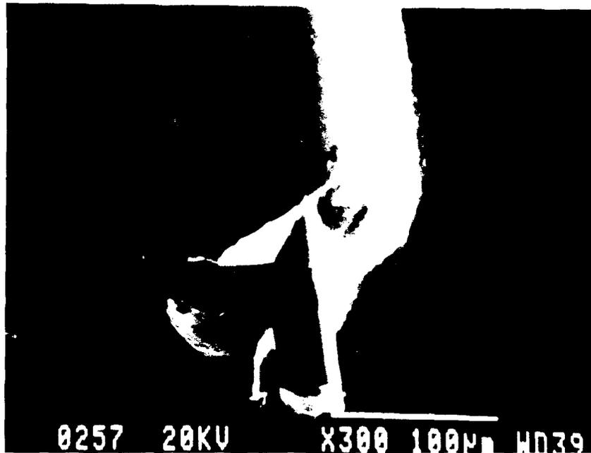
Figure 33. Fiber Series H Tensile Failure Location
