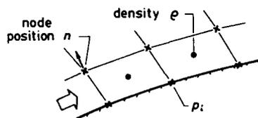
Figure 2: Six streamline nodes and two density variables determining surface pressure  $p_i$ .
