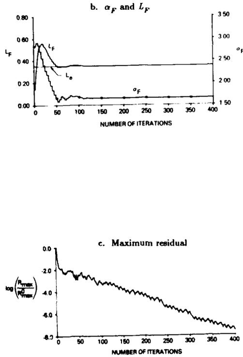
Figure 24. Iterative Histories for the Free-Air Solutions Using Scheme I ( $h = 4.6$ ,  $M_{\infty e} = 0.8$ ,  $L_e = 0.35$ ).
