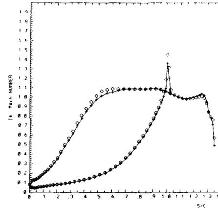
Fig. 14c Calculated (+) and required (o) Mach number distributions after 2 modifications
