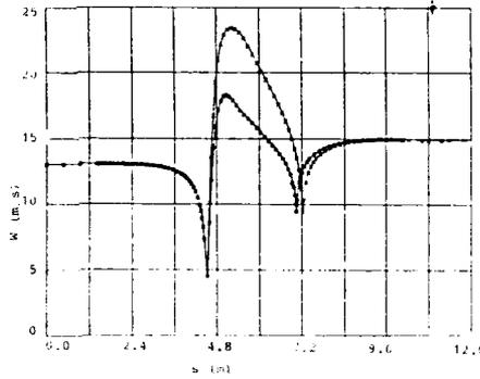
FIG. 8.6.1 Test case for the inverse method. The Hobson cascade.
