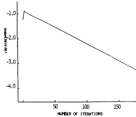
Fig. 13 Convergence history for the inverse design from a cascade of 12% biconvex airfoils to a straight channel at  $M_\infty = 0.62$ .
