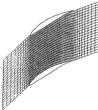
Fig. 6 H-grid discretization
