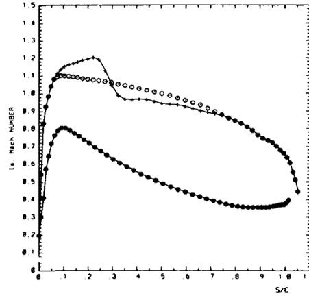
Fig. 13c Initial (+) and required (O) Mach number distributions
