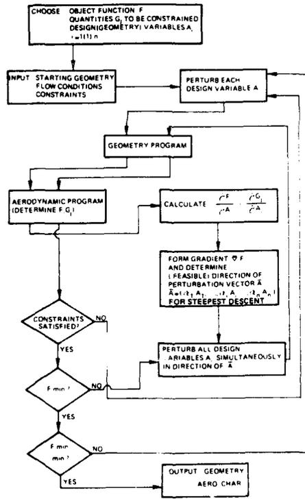
Figure 3. Flow chart of direct numerical optimization
