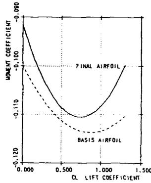
Fig. 33b - Off-design performance  $C_m$  - vs -  $C_L$  ( $M = 0.25$ ).
