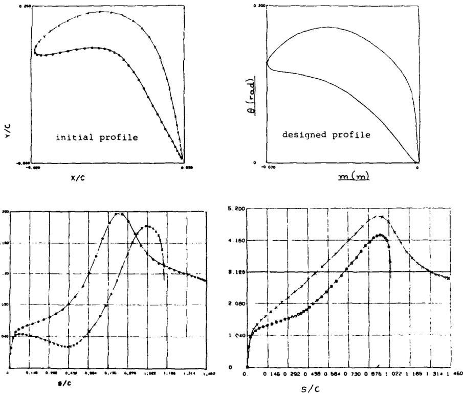
Fig.10.4 Design of a thicker profile using the inverse inviscid flow method.
