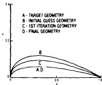
Fig. 42 - Viscous airfoil contour variation.
