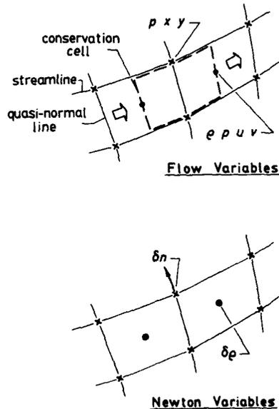
Figure 1: Euler grid node and variable locations.
