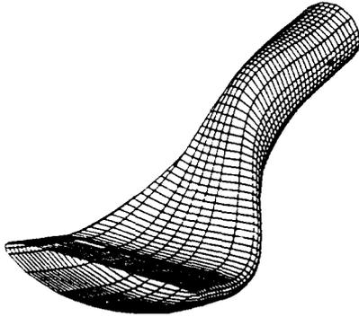
Fig. 7 Air intake scoop designed using Stanitz method [34]
