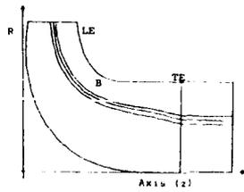
FIG. 8.6.2 Test case for the inverse method. A radial inflow turbine.
