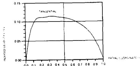
(a) propeller-induced tangential velocity
