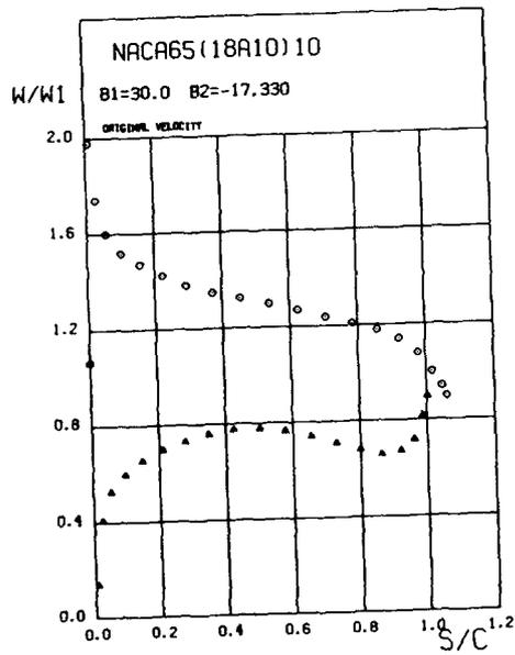
Fig. 4c Initial velocity distribution
