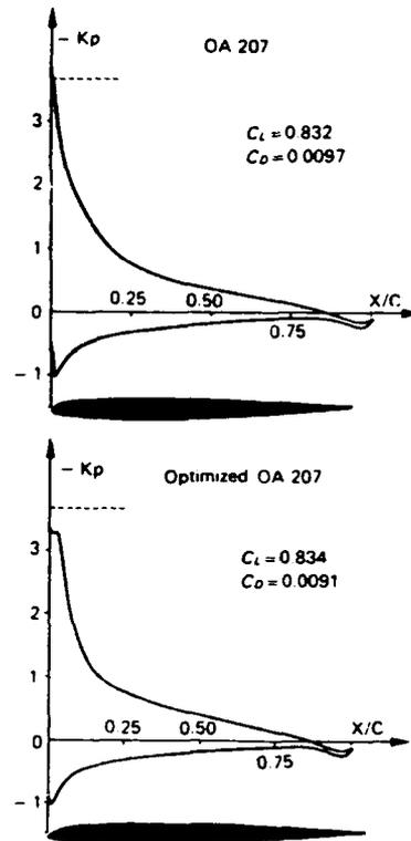
Fig. 56 - Comparison of pressure distributions at  $M = 0.4$ ,  $\alpha = 7.5^\circ$ ,  $Re = 2.10^6$
