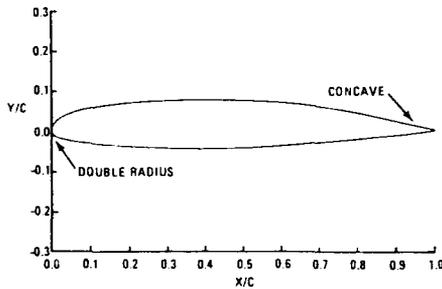
Fig. 36 - Case 2. Geometry previously designed airfoil: geometrically and aerodynamically unacceptable.
