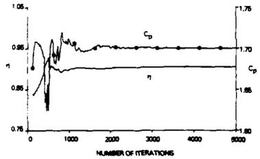
Figure 16. Power and Efficiency Iterative Histories for the Three-Design-Parameter Problem.
