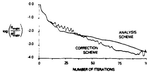
Figure 21. Residual Evolution Histories for the Correction Problem and the Analysis Problem in Free Air (Scheme III).
