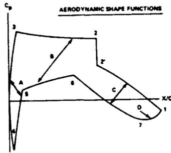
Fig. 18 - Analytical representation of the pressure distribution.
