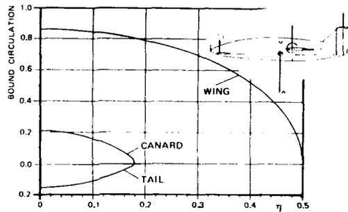
Fig. 17 Spanloads for minimum trimmed induced-drag (three-surface aircraft)
