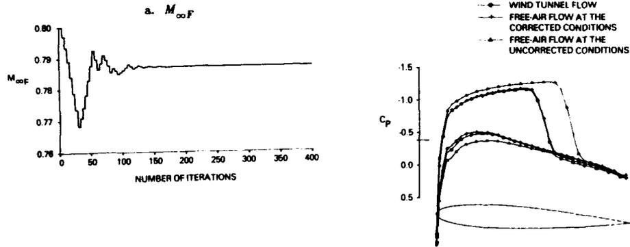
Figure 25. Pressure Distribution on the Airfoil Surface ( $h = 4.6$ ,  $M_{\infty e} = 0.8$ ,  $L_e = 0.35$ ).
