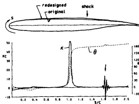
Figure 7: Comparison between original and mixed-inverse redesigned airfoil. Surface angle and curvature distributions on redesigned airfoil.
