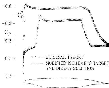
Fig. 9 Designed contour, original target and computed pressure distribution; case LFC1,  $M_\infty = 0.766$ ,  $\alpha = 0^\circ$ ,  $C_L = 0.5166$ ,  $C_D = 0.0001$
