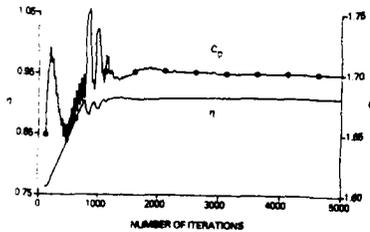
Figure 13. Power and Efficiency Iterative Histories for the Two-Design-Parameter Problem with Perturbed Initial Conditions.
