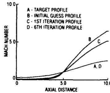
Fig. 82 - 3-D nozzle centerline Mach number contours.
