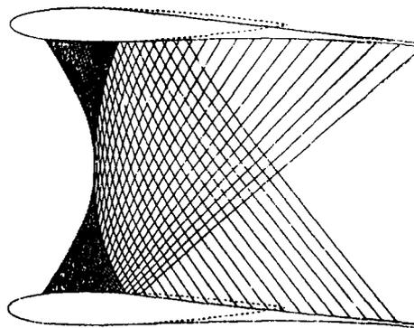
Fig. 10 Lifting choked shock-free cascade designed using fictitious gas [64]
