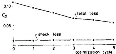
Figure 23: Reduction in total and shock loss during compressor cascade optimization.
