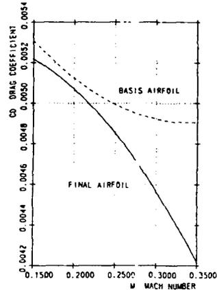
Fig. 33c - Off-design performance  $C_D$  - vs -  $M$  ( $\alpha = 0$ ).
