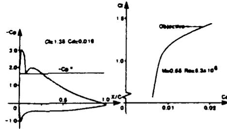
Fig. 26 - HORØ7 airfoil computed performances in take-off conditions.
