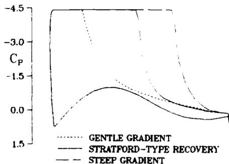
Fig. 7 Types of pressure distributions with various recovery patterns following "rooftop" region
