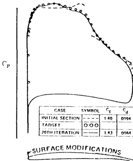
Fig. 12 Airfoil re-design with wavy-wall technique;  $M_\infty = 0.680$
