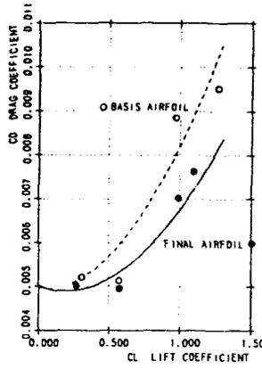
Fig. 33a - Off-design performance  $C_D$  - vs -  $C_L$  ( $M = 0.25$ ).
