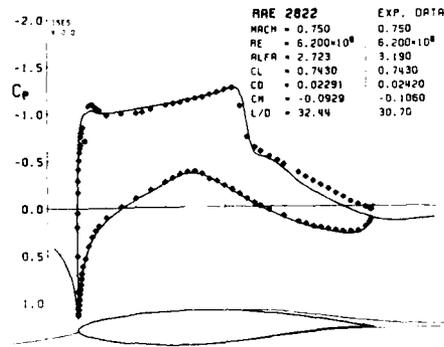
Figure 17: RAE 2822 airfoil calculation and experimental data.
