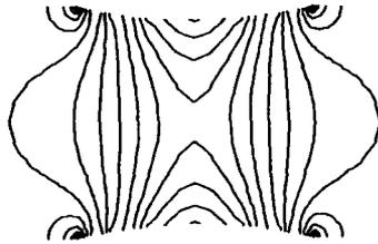
Fig. 10 Computed isobars for the analysis of a flow through the cascade of 12% thick biconvex airfoils at  $M_\infty = 0.62$ .
