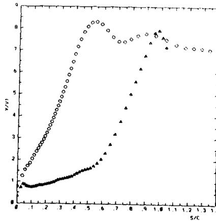
Fig. 9b Off-design velocity distribution ( $M_2 = 0.8$ )
