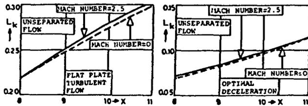
FIG. 6.8 Effects of compressibility on some characteristic image curves for turbulent flow.
