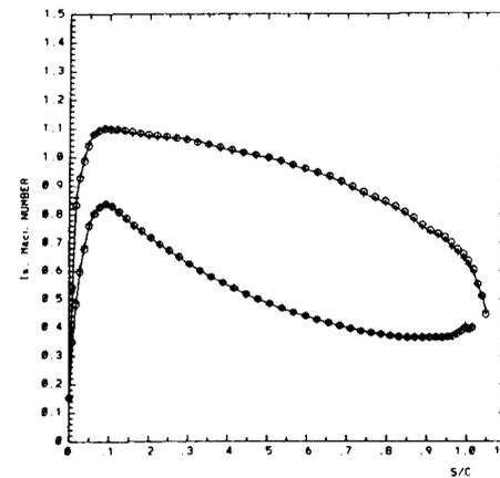
Fig. 13e Calculated (+) and required (O) Mach number distributions after 3 modifications
