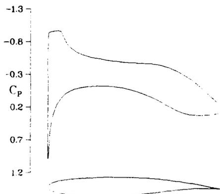
Fig. 12 Pressure distribution on Korn airfoil;
