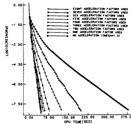
Fig. 14 Typical convergence histories for SFC compressible flow with SLOR and DMR method
