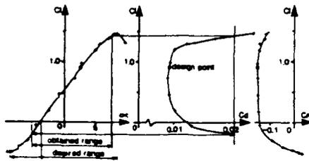
Fig. 61 - OAF102 airfoil. Experimental data  $M = 0.62$ ,  $Re = 1.10^6$ .
