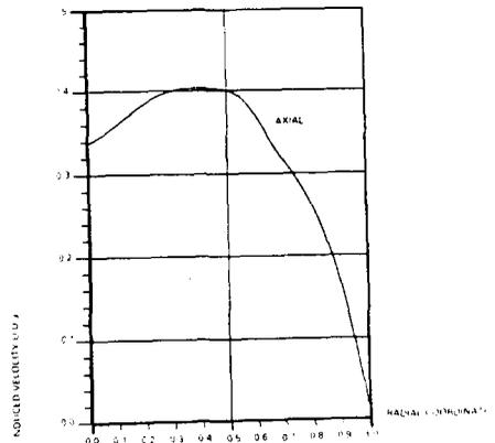
(b) propeller-induced axial velocity
