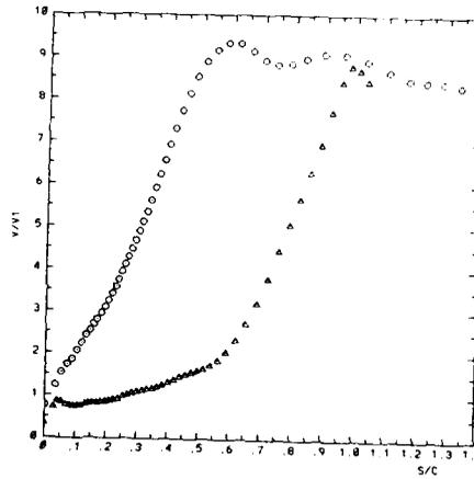
Fig. 9a Off-design velocity distribution ( $M_2 = 1$ )
