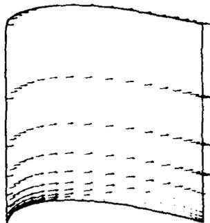
Fig. 41 - Viscous airfoil initial guess velocity field.
