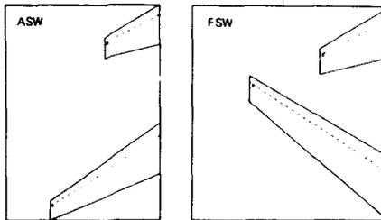
Fig. 18 Spanloads of forward and aft swept wing configurations
