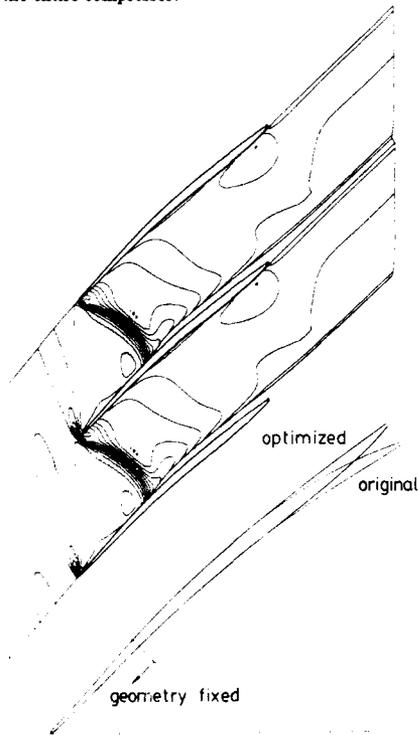
Figure 22: Calculated flow for optimized compressor cascade and geometry comparison.
