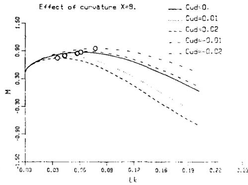
FIG. 10.8 Influence of wall curvature effects on the locus of maximum  $M_2$ -values (Optimum Deceleration Curve)
