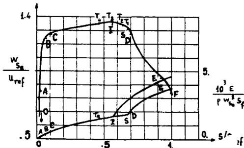
FIG.7.5 The  $W_{se}(s)$ -distribution and the kinetic energy loss distribution corresponding to the optimum image curve of Fig.(7.2)
