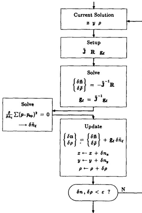
Figure 15: Newton method with embedded optimization (modal-inverse).
