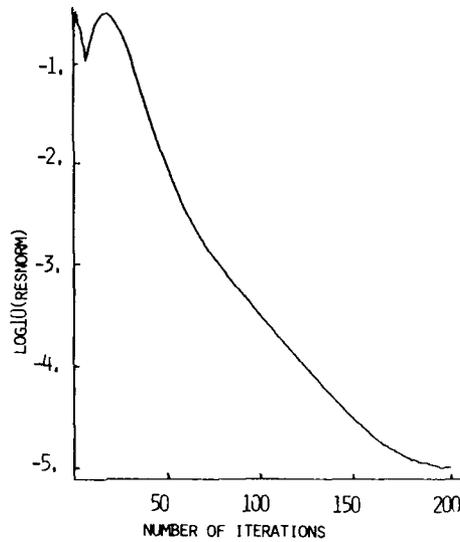
Fig. 7 Convergence history for the inverse design from a cascade of dipoles to a straight channel
