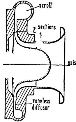
Meridional compressor shapes with measurement locations (--- first new design) (— second new design)
