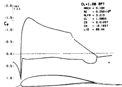
Figure 25: Calculated  $C_p$  distribution for airfoil optimized at  $C_L = 1.08$ .
