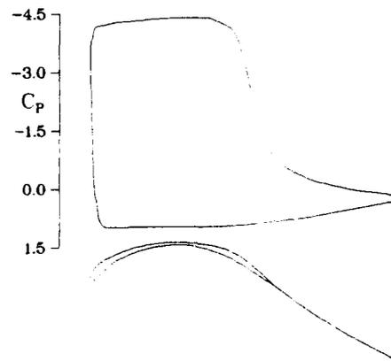
Fig. 8 Maximum lift pressure distribution and corresponding contour
