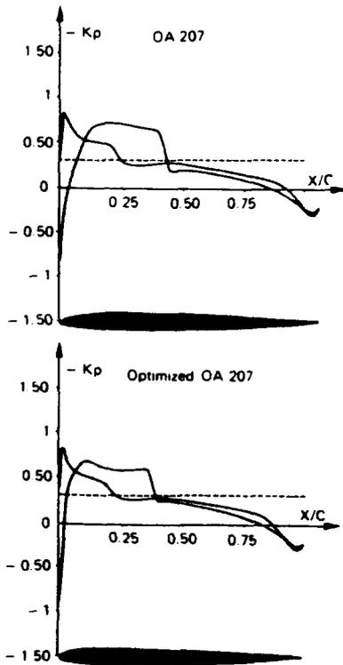
Fig. 55 - Comparison of pressure distributions at  $M = 0.85$ ,  $\alpha = 0.5^\circ$ ,  $Re = 3.7 \cdot 10^6$
