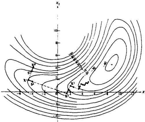
Fig. 7 - Geometric interpretation of the steepest descent method.
