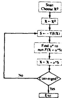
Fig. 6 - Algorithm for the steepest descent method.
