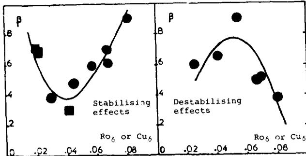
FIG.3.3 Variation of the mean beta-value with the overall Rotation number  $Ro_6$  and Curvature number  $Cu_6$ .
