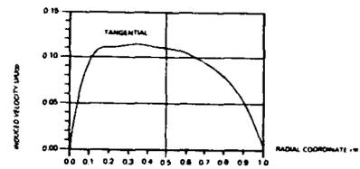
(a) propeller-induced tangential velocity
