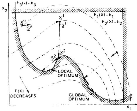
Figure 1. Example of an iterative search procedure
