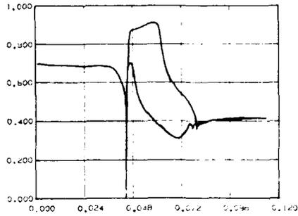
FIG. 10.7 Optimized high subsonic flow, high loaded compressor profile
