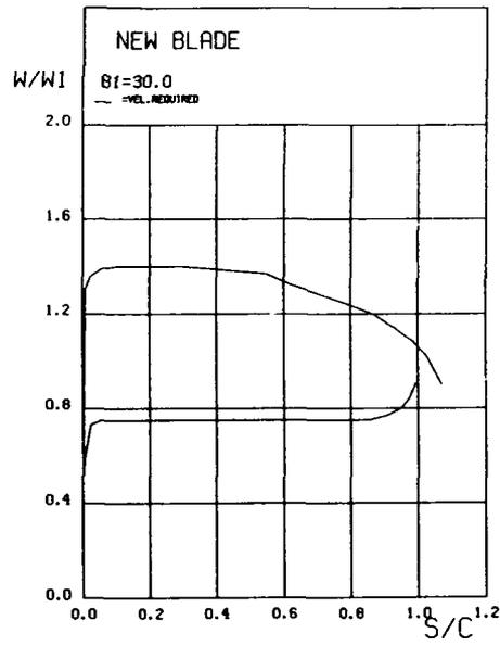
Fig. 4a Required velocity distribution
