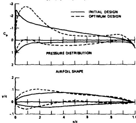
Fig. 46 - Lift maximization,  $M = 0.1$ ,  $\alpha = 6^\circ$ .
