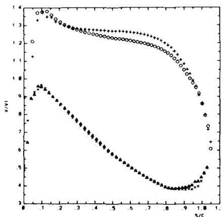
Fig. 7c required velocity (O, Δ) versus distribution obtained after 5 modifications (+, x)
