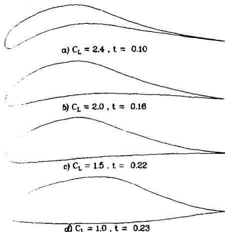
Fig. 18 Effect of design lift on airfoil shape; incompressible flow
