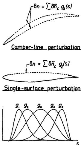
Figure 8: Camber-line and single-surface modal geometry perturbations.
