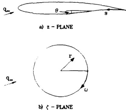
Fig. 11 Mapping of airfoil to circle
