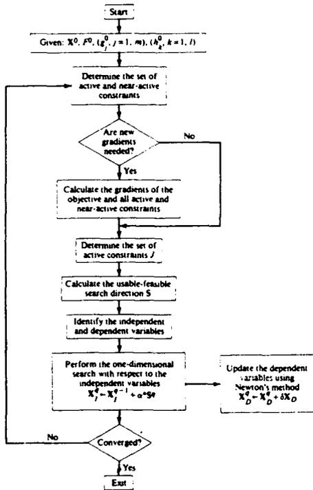
Fig. 11 - Algorithm for the robust feasible directions method.
