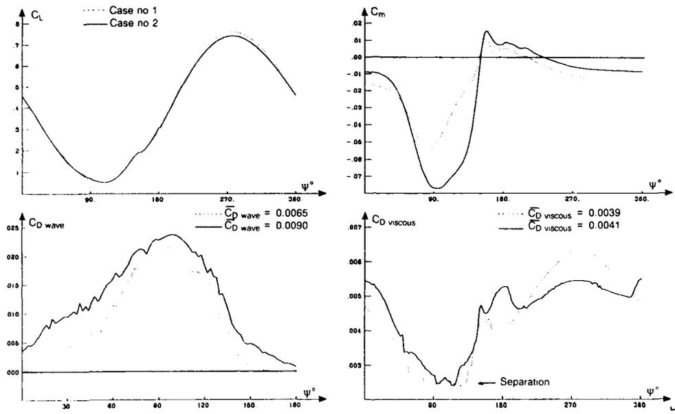
Fig. 92 - Unsteady aerodynamic performance for the optimized airfoils  $C_L = 0.3$ .
