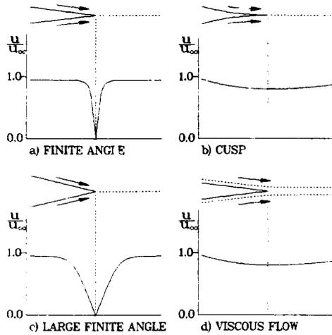
Fig. 3 Possible flow conditions near trailing edge
