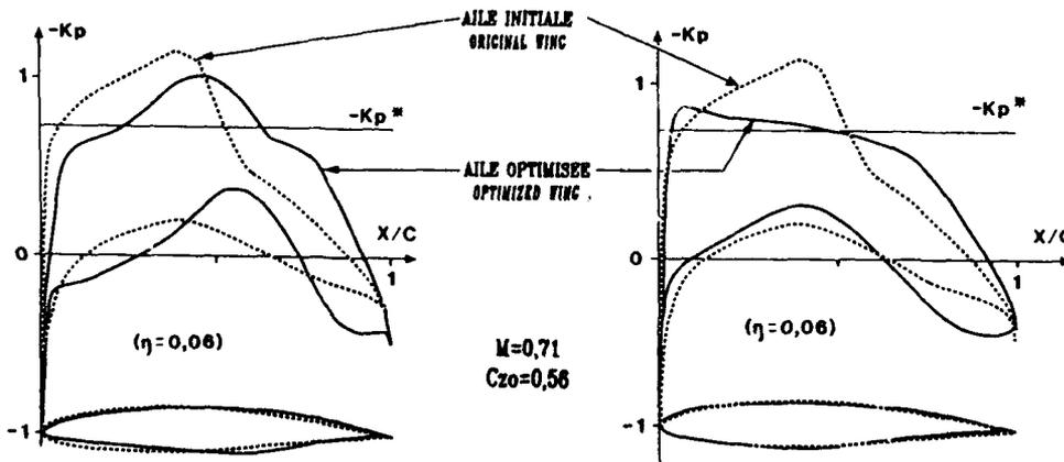
Fig. 34 - Optimization of a rectangular wing. Drag minimization. Constraint:  $C_L \geq C_{L0}$ .
