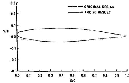
Fig. 37 - Case 2. Comparison of TRO-2D drag optimized airfoil to previous design.
