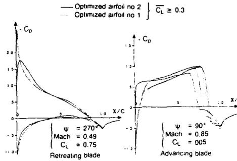
Fig. 91 - Unsteady pressure distribution, optimized airfoils.
