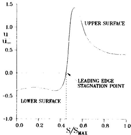
Fig. 4 General form of airfoil speed distribution
