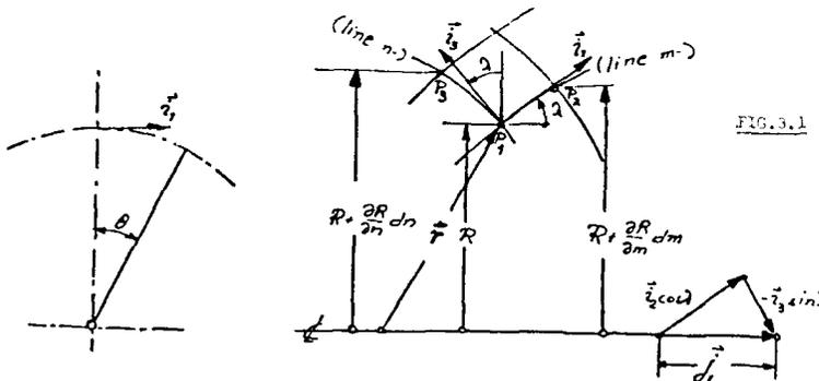
FIG.3.1 Curvilinear orthogonal axially symmetric coordinate system.
