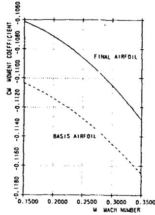
Fig. 33d - Off-design performance  $C_m$  - vs -  $M$  ( $\alpha = 0$ ).
