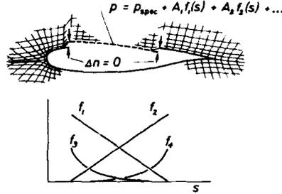
Figure 3: Mixed-inverse problem with two geometry continuity constraints.
