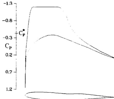
Fig. 5 "Shockless" target pressure distribution and corresponding airfoil
