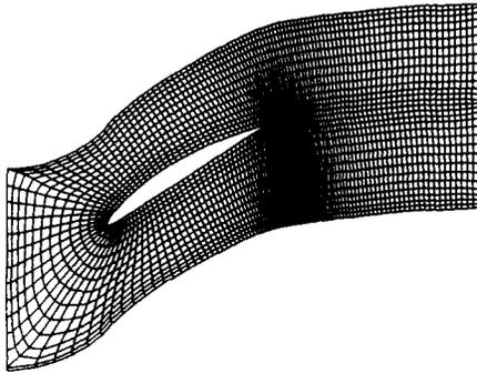
Fig. 10 C-grid discretization
