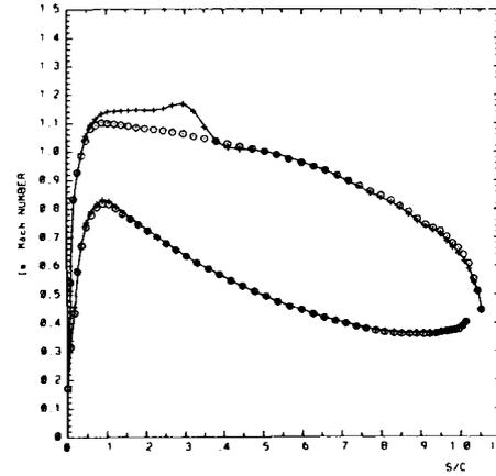
Fig. 13d Calculated (+) and required (O) Mach number distributions after 2 modifications
