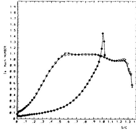
Fig. 14b Calculated (+) and required (o) Mach number distributions after 1 modification
