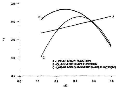
Figure 18. Optimum Blade Angle Perturbations.
