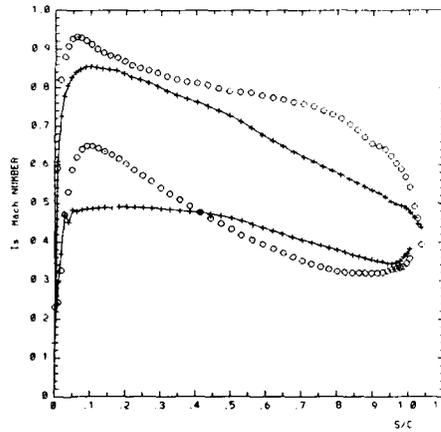
Fig. 12a Initial (+) and required (O) Mach number distributions
