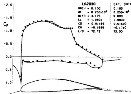
Figure 24: Calculated and experimental surface  $C_p$  for LA203A airfoil.
