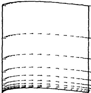
Fig. 40 - Viscous airfoil target velocity field.
