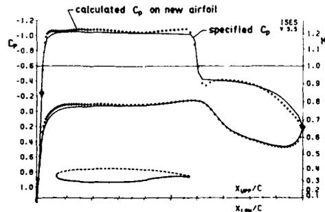
Figure 9 Specified and new calculated  $C_p$  distributions on airfoil redesigned using modal-inverse.
