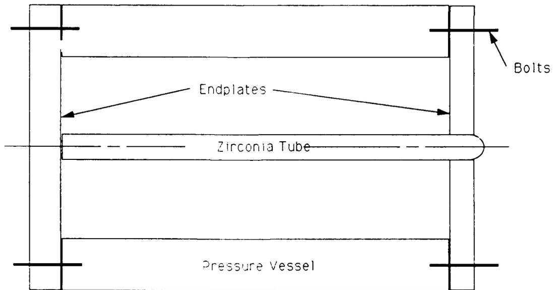
Figure 6-4. Fourth Pressure Vessel Design Option
