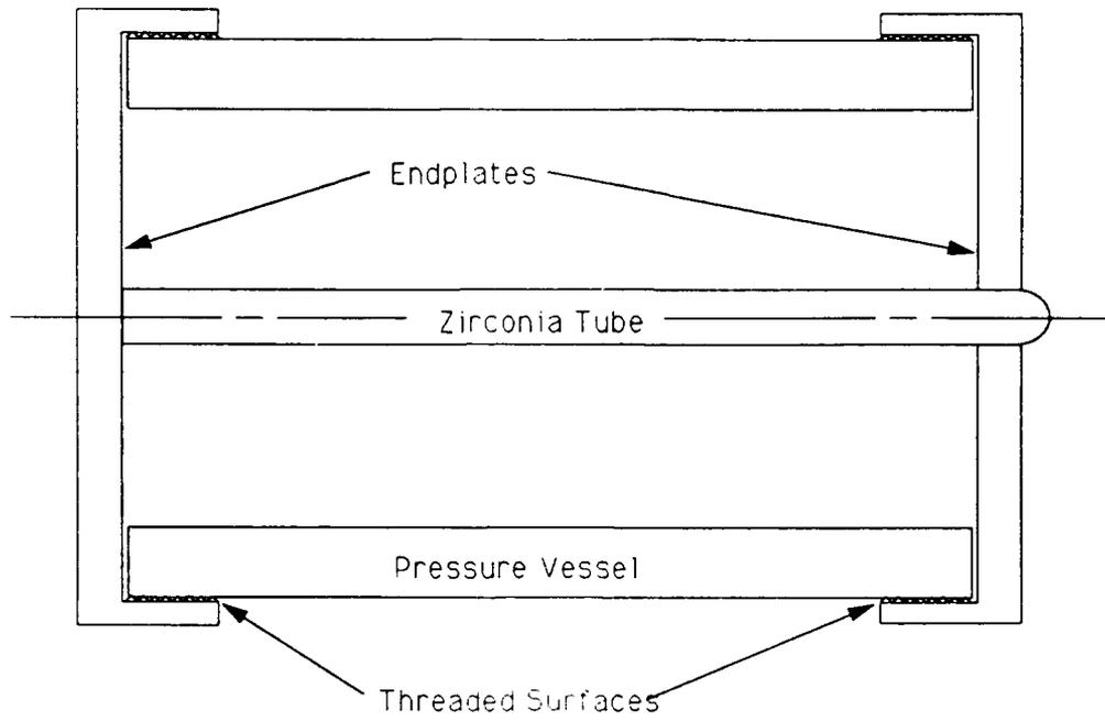
Figure 6-3. Third Pressure Vessel Design Option
