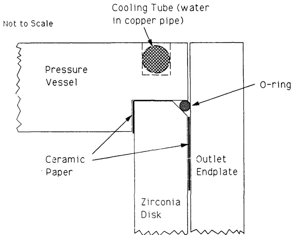
Figure 6-9. Advanced Zirconia-Metal Joint, Design A.
