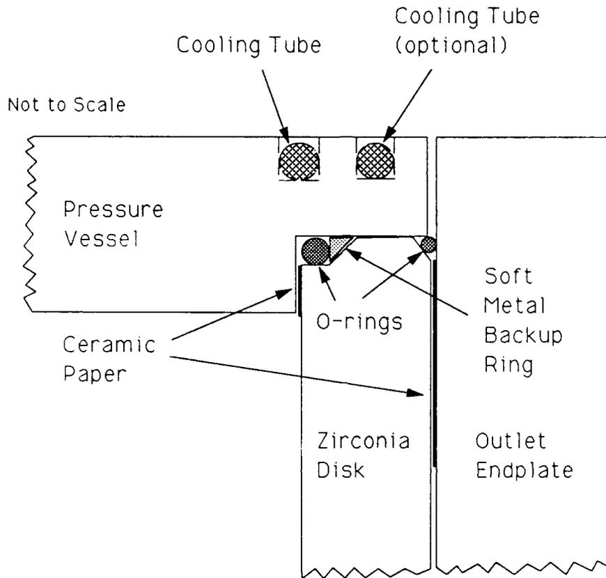
Figure 6-10. Advanced Zirconia-Metal Joint, Design B. Attachment of Endplate to Pressure Vessel not shown. The Backup Ring is typically made of copper, and is used to prevent extrusion of the O-ring.
