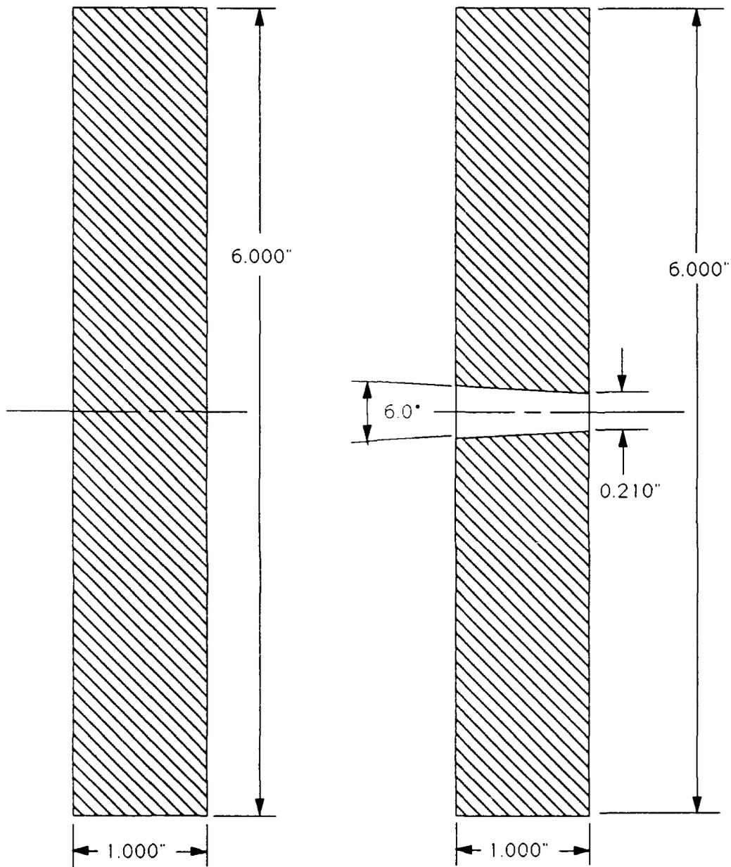
Figure 6-6. Zirconia Disk Cross-section Views. Left drawing is disk as received from supplier. Right drawing is disk ready to be joined to the zirconia tube.
