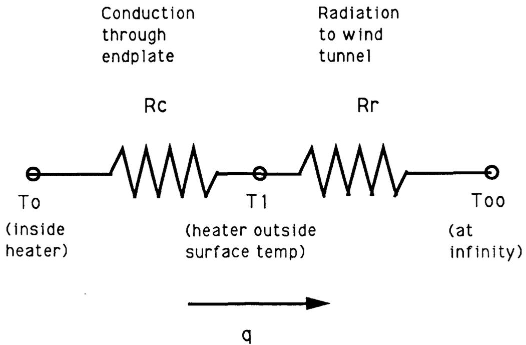
Figure 5-2. End Effects Heat Transfer Model.
