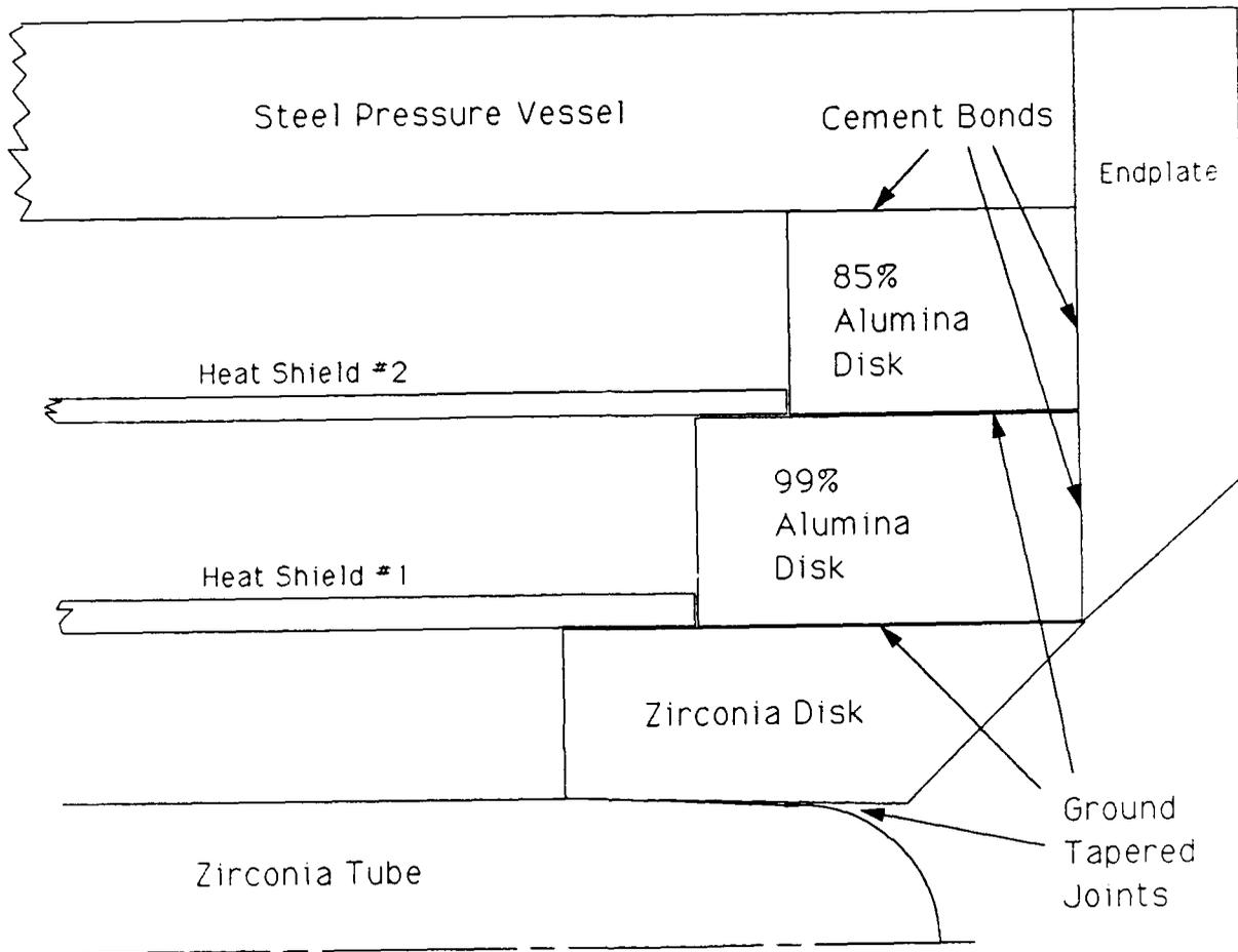
Figure 6-5. Multiple Ground Tapered Joint.
