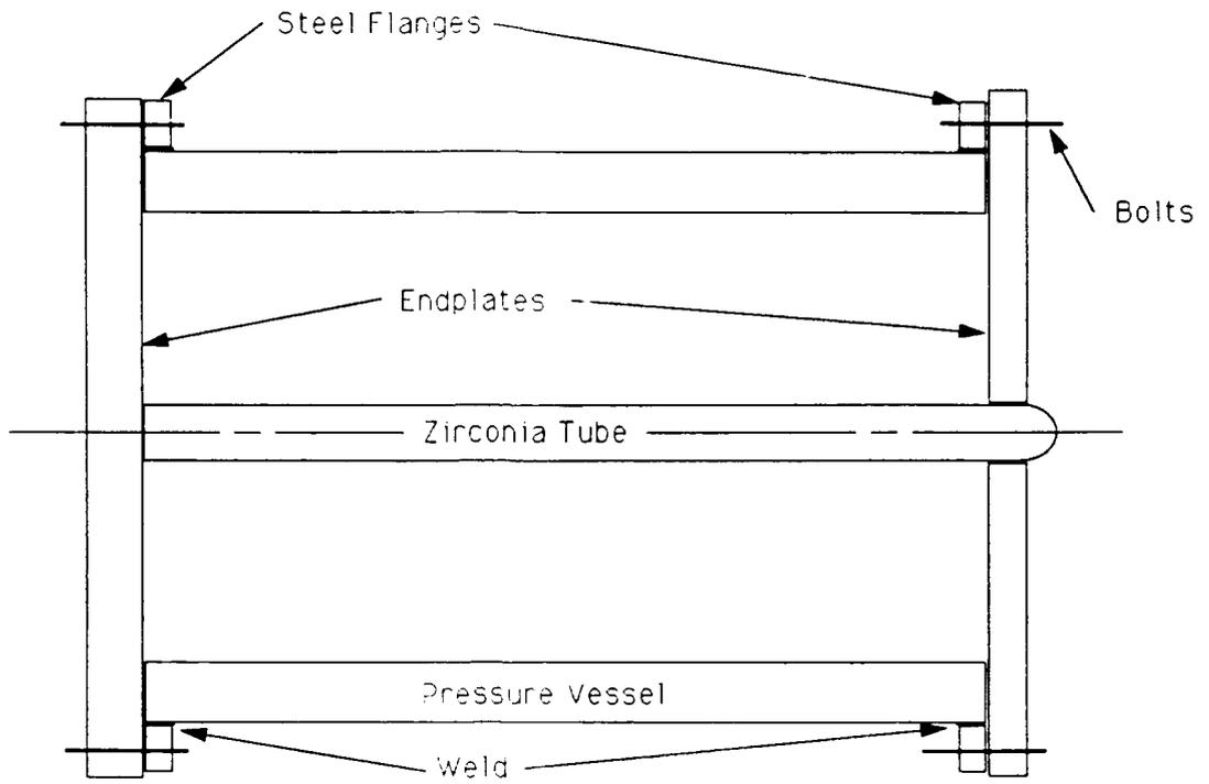
Figure 6-1. First Pressure Vessel Design Option
