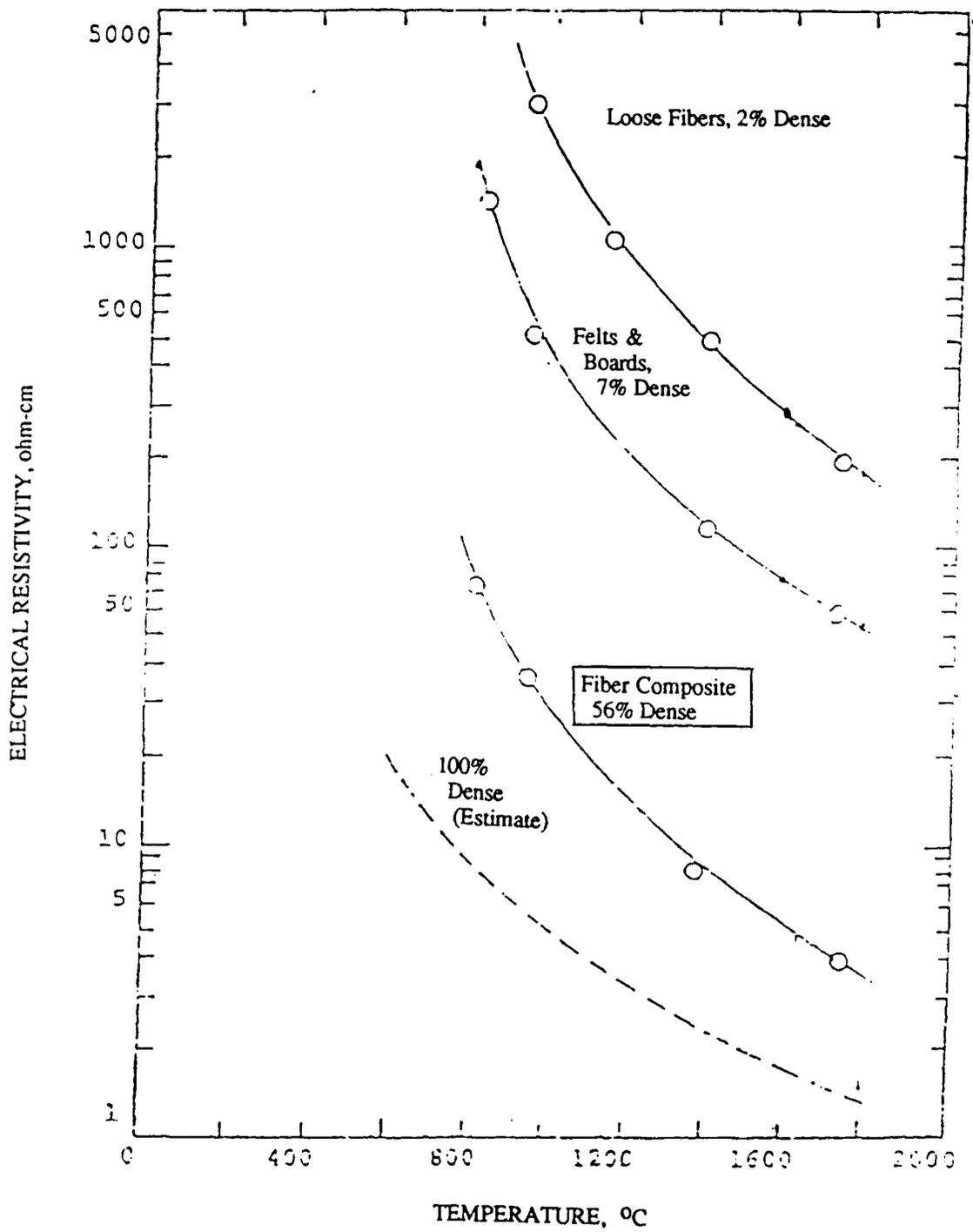
Figure 7-2. Resistivity of zirconia composites.
