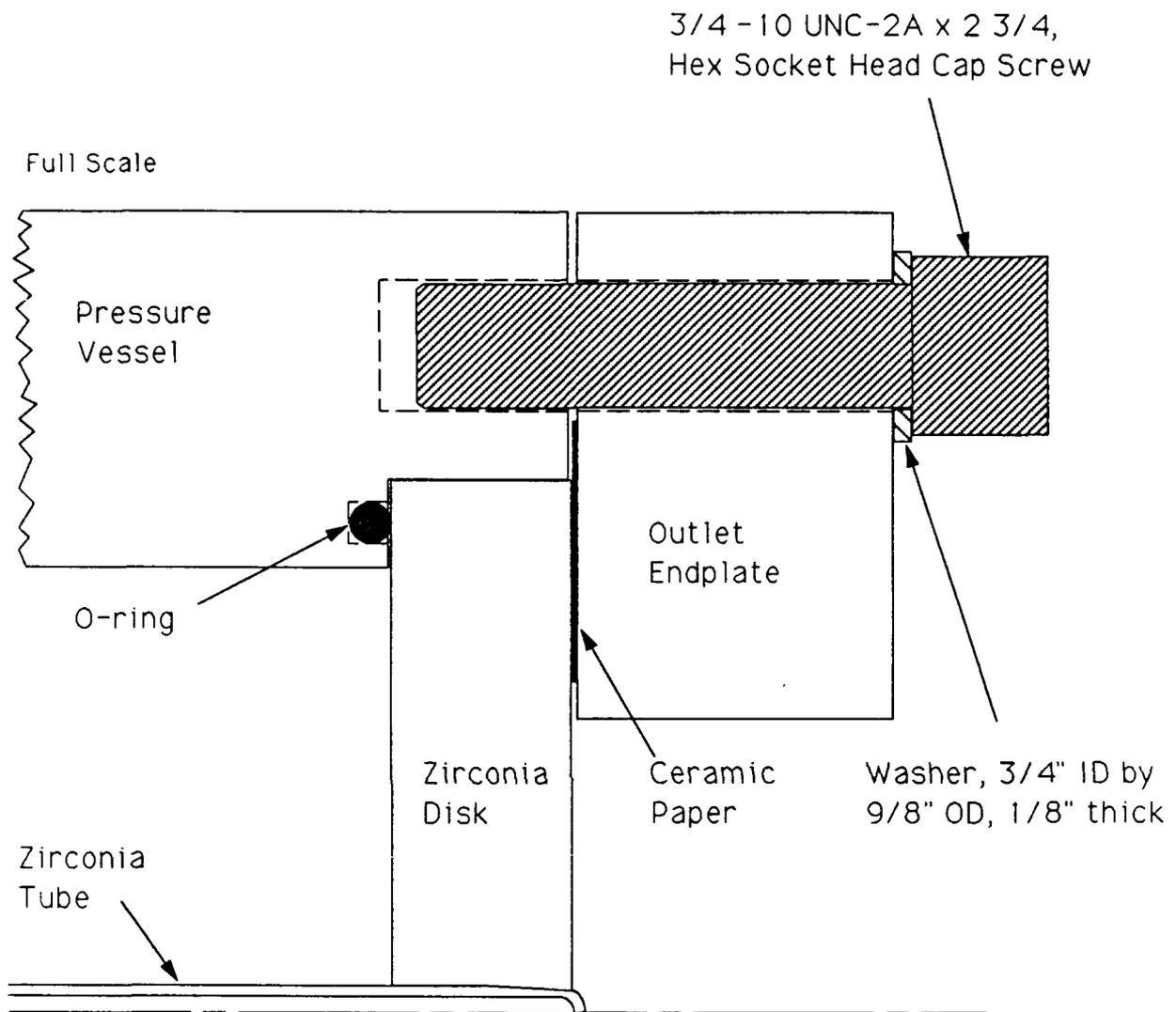
Figure 6-8. Zirconia-Metal Joint Design. Heat shields omitted for clarity.
