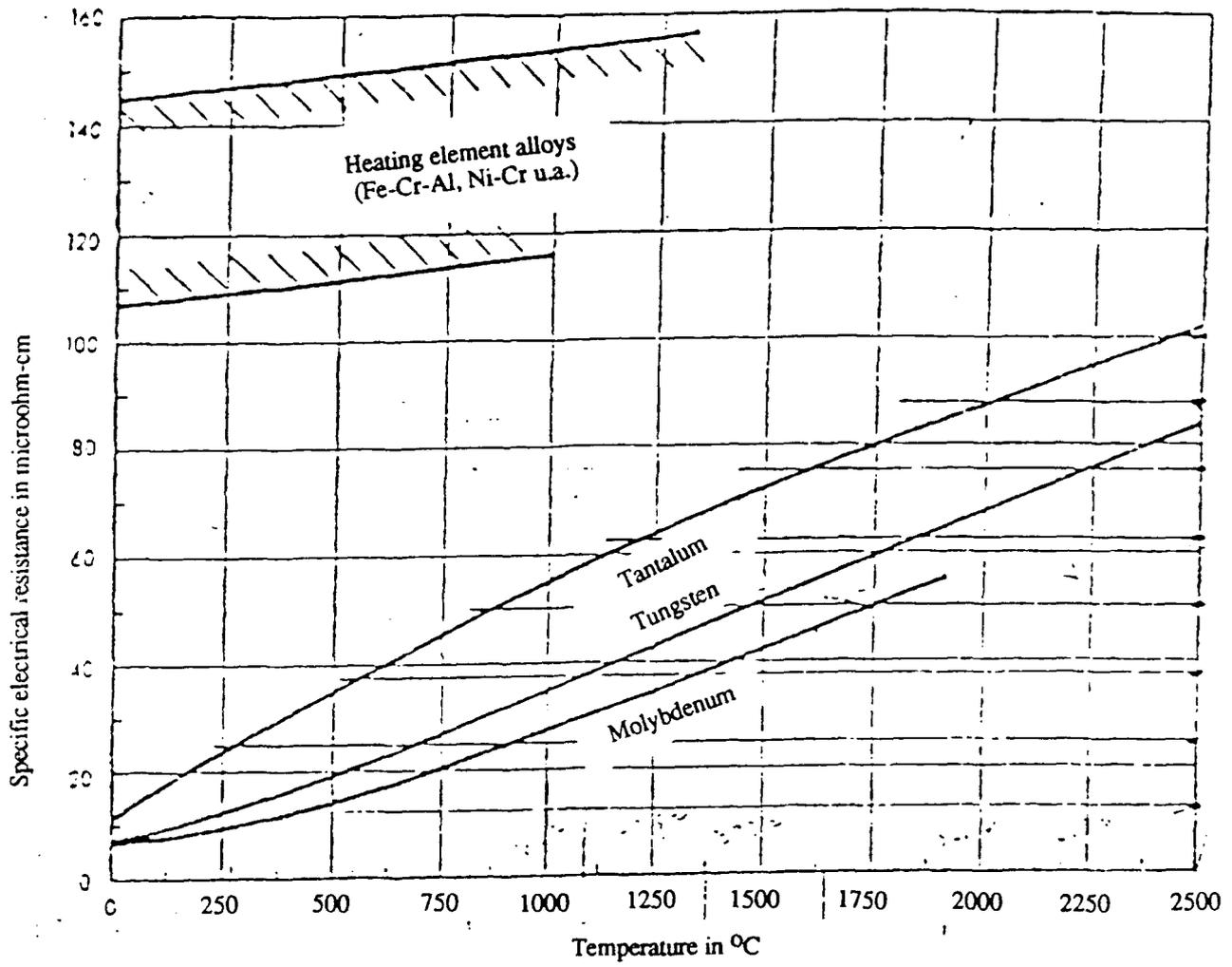
Figure 7-1. Resistivity of tantalum and other metals.
