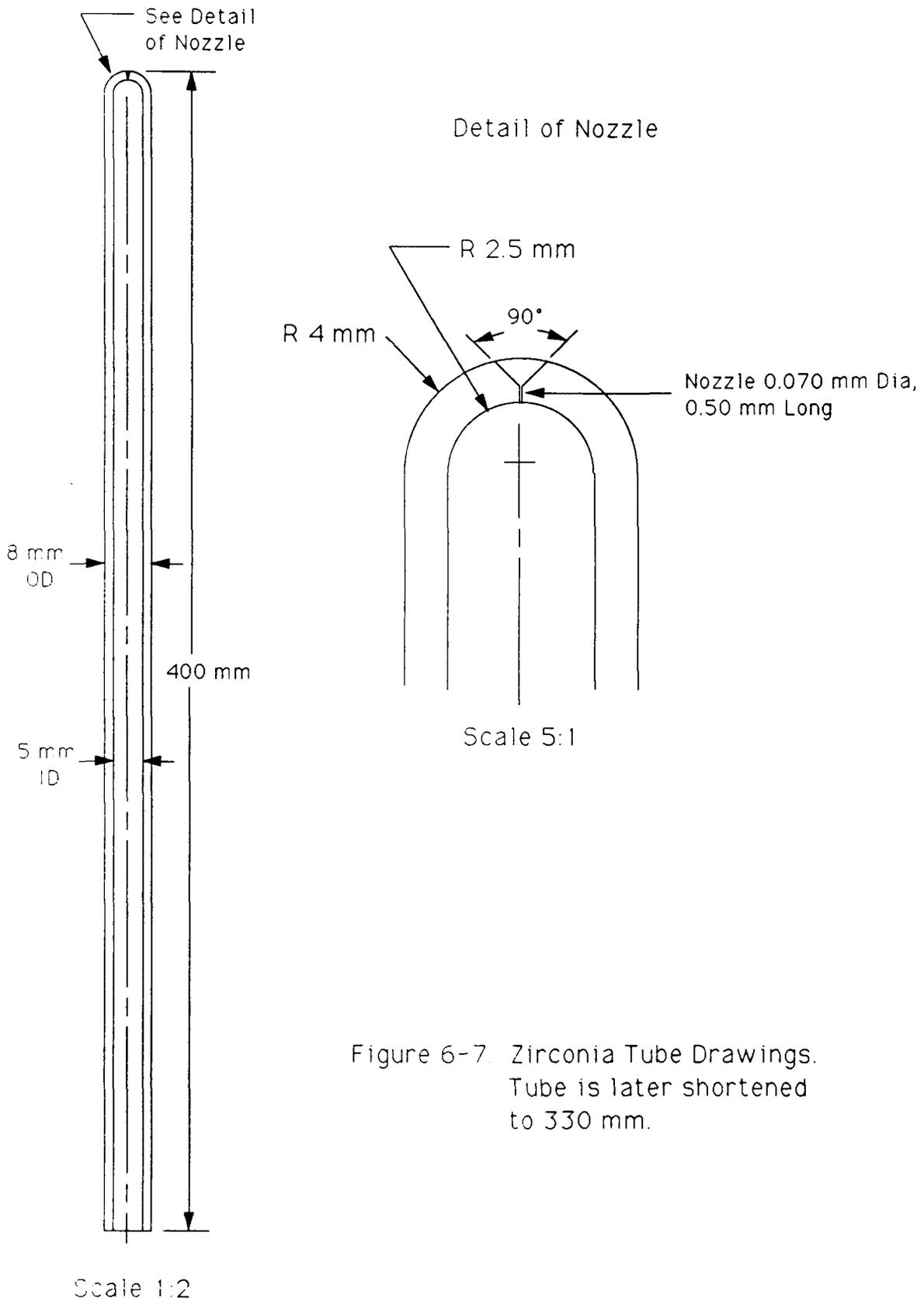
Figure 6-7. Zirconia Tube Drawings. Tube is later shortened to 330 mm.
