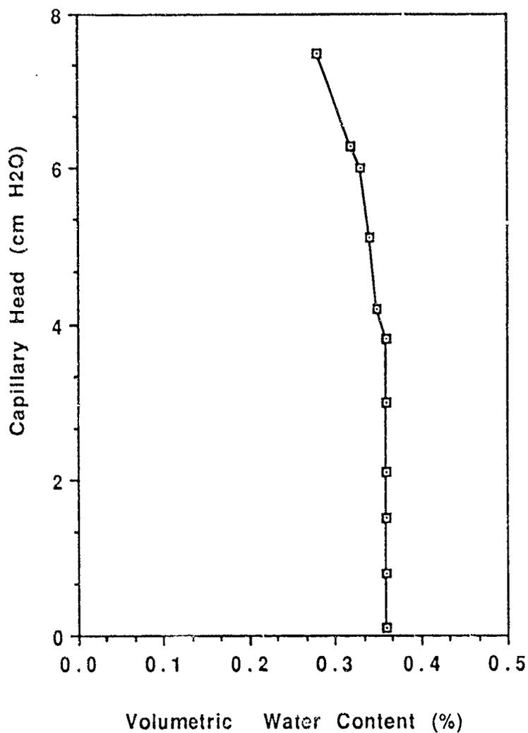
Figure A-2. Capillary Pressure-Volumetric Water Content for JP-4/Water System (0.5mm Sand).
