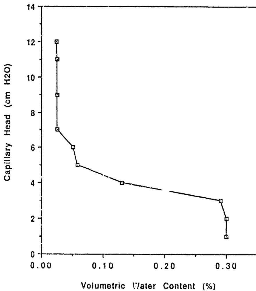
Figure A-4. Capillary Pressure-Volumetric Organic Content for JP-4/Air System (0.6mm Sand).
