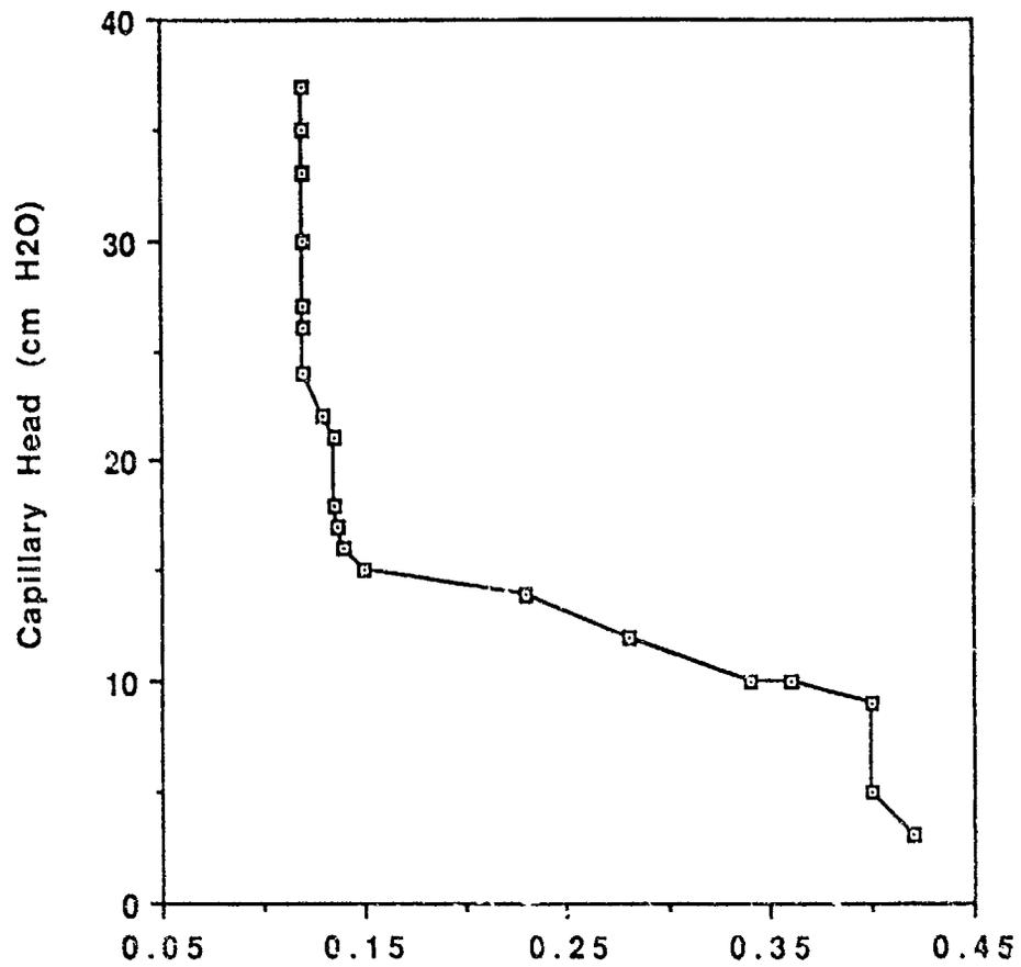
Figure A-3. Capillary Pressure-Volumetric Water Content for Air/Water System (0.5mm Sand).
