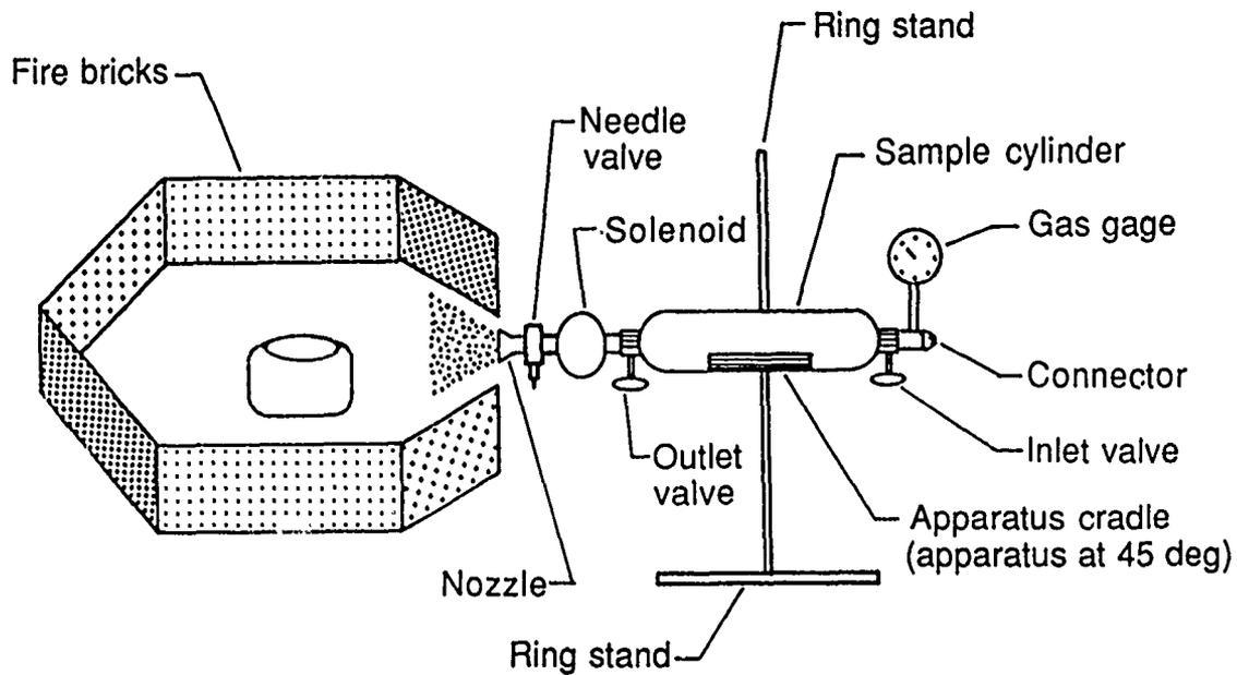
Figure 4. Laboratory-Scale Discharge Extinguishment Apparatus, Configuration 4.
