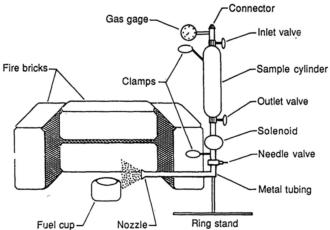
Figure 3. Laboratory-Scale Discharge Extinguishment Apparatus, Configuration 3.
