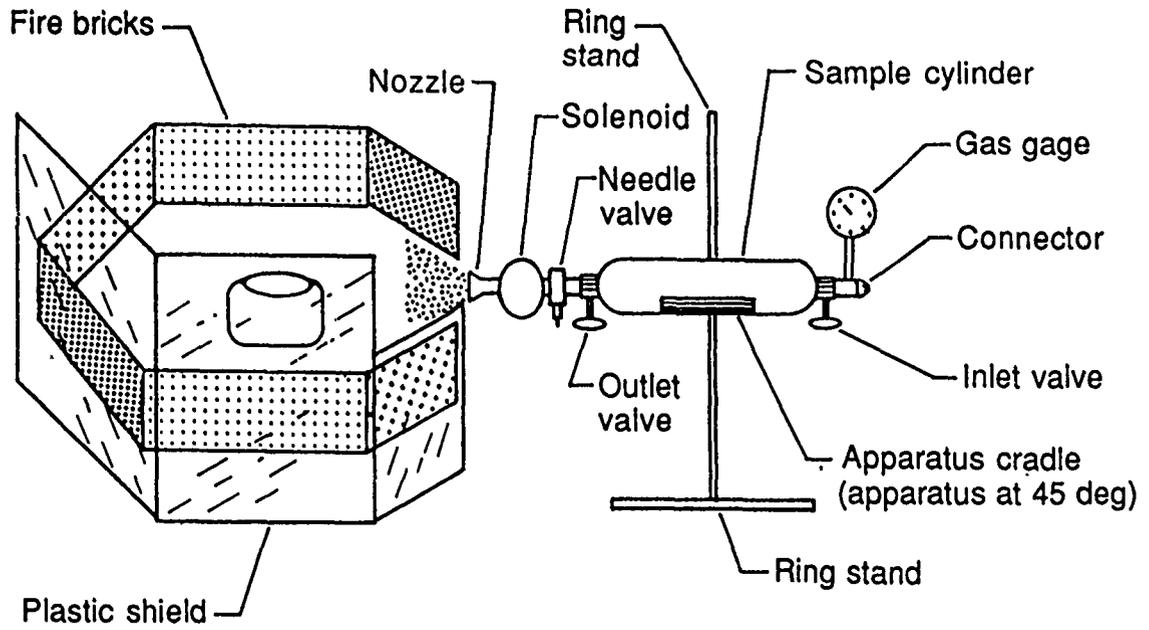
Figure 6. Laboratory-Scale Discharge Extinguishment Apparatus, Configuration 6.
