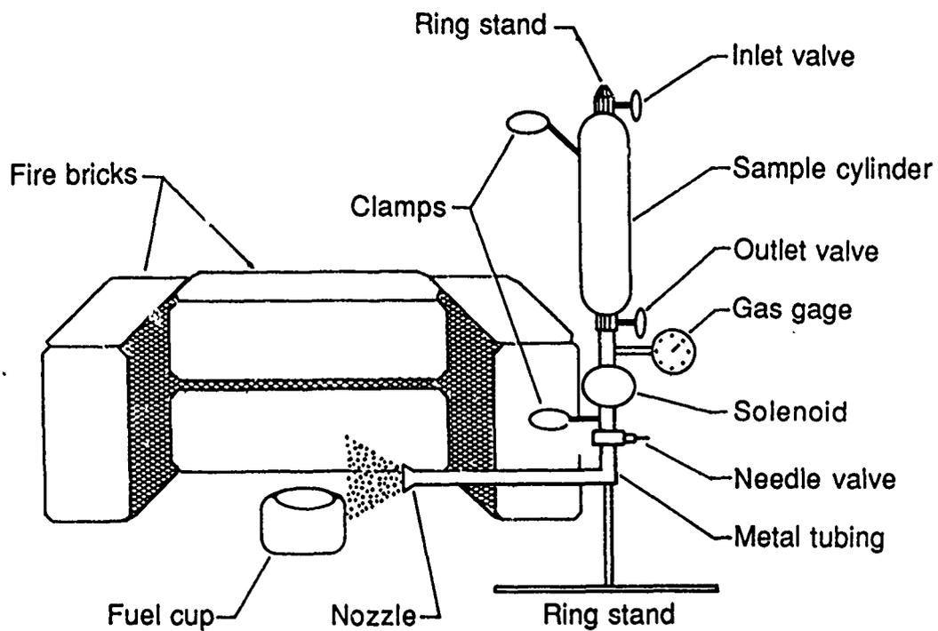
Figure 2. Laboratory-Scale Discharge Extinguishment Apparatus, Configuration 2.
