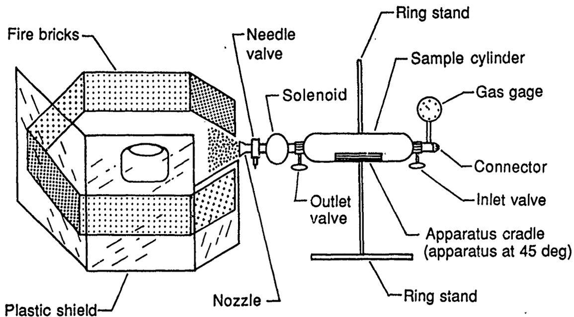
Figure 5. Laboratory-Scale Discharge Extinguishment Apparatus, Configuration 5.
