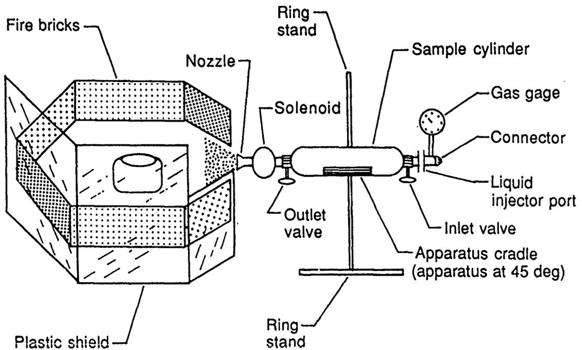
Figure 7. Laboratory-Scale Discharge Extinguishment Apparatus, Configuration 7.
