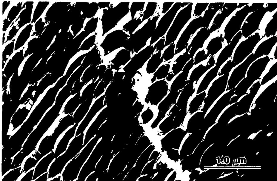
Figure 3. TEM micrograph showing ultramicrotomy damaged structure of cut stone.
