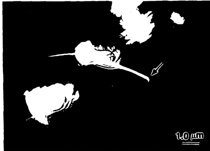
Fig. 8. TEM micrograph of the composite (initial  $C_2S$  particle size,  $0.25 \mu\text{m}$ ) fired at  $1550^\circ\text{C}$ , showing radial microcracking emanating from particles (possibly  $\gamma\text{-}C_2S$ ) and extending along grain boundaries of the matrix. Grain boundary sliding (as arrow indicated) is also observed.
