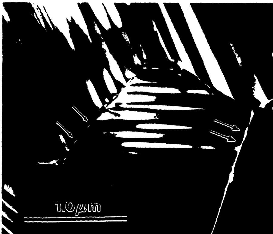
Figure 8: TEM micrograph of polycrystalline  $\text{Ca}_2\text{SiO}_4$  fired for 3 hours at  $1400^\circ\text{C}$ . Here grain growth has increased the stress at the grain boundaries such that some of the grain boundary facets are microcracked.
