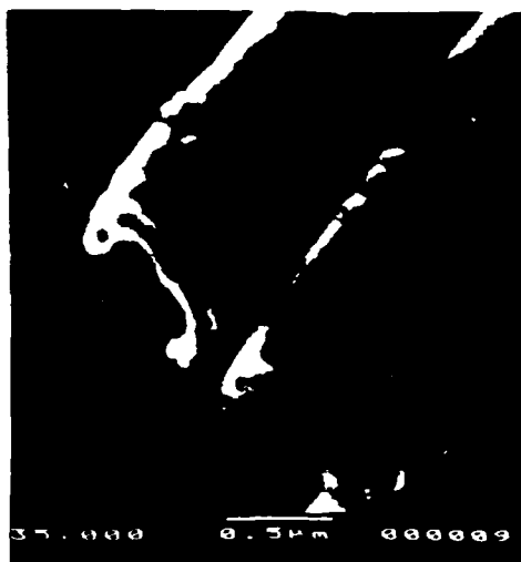
Figure 2. Scanning electron micrograph of template-synthesized polypyrrole tubules.
