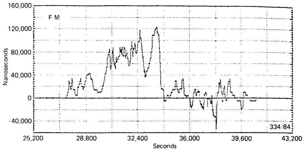
**Figure 3**—Nighttime time-difference deviations from the long-term daytime average recorded by LONARS at NOSC, Nov 30, 1983. The S-M time-difference data, not shown, are similar in magnitude and shape to the F-M data.
