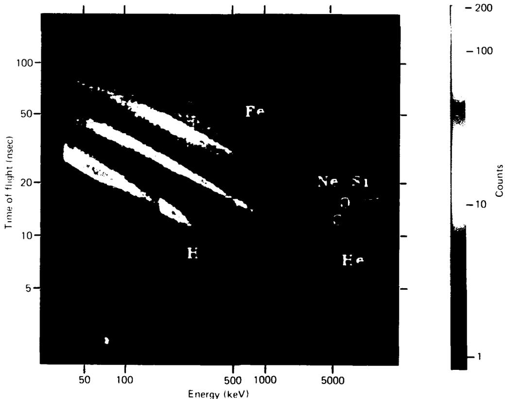
**Figure 3**—Flight pulse-height analysis matrix accumulated by MEPA, September 12, 1984, 21:19 to 23:31 UT ( $L = 5.15$  to  $7.76$ ). Tracks of protons, helium, carbon, oxygen, the neon-silicon group, and iron can be seen. Jumps in intensity along the proton and helium tracks reflect energy boundaries in the priority system.
