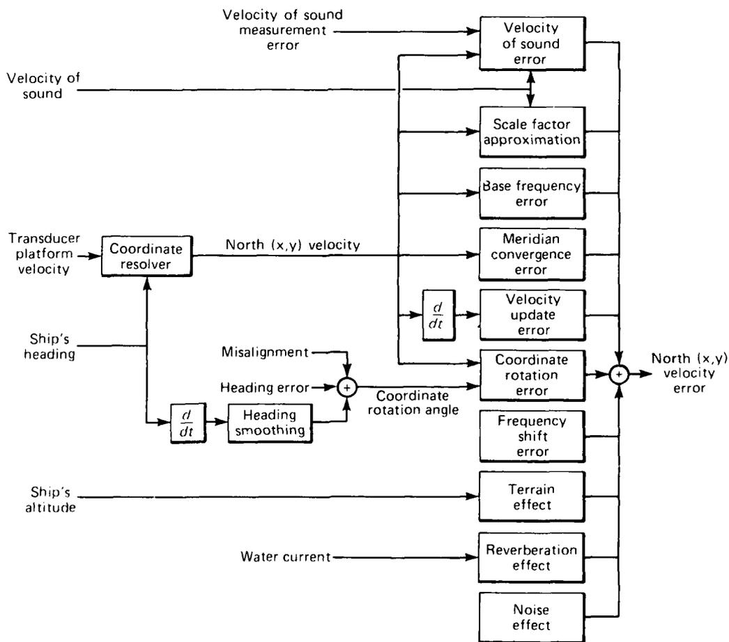
Figure 2—Flow diagram of the velocity error model.
