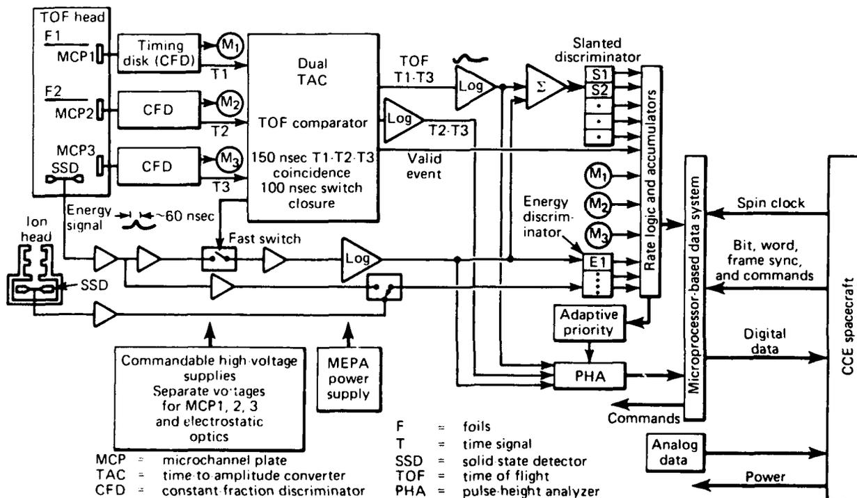
**Figure 2**—Functional block diagram of the MEPA instrument.
