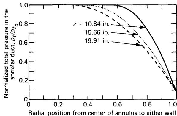
**Figure 2**—Assumed total pressure radial profiles in the CII duct, normalized with respect to the plenum total pressure and calculated to match the plenum and wall pressures and to conserve mass. Mach 2.4; Reynolds number  $(37 \text{ to } 58) \times 10^6/\text{ft}$ .
