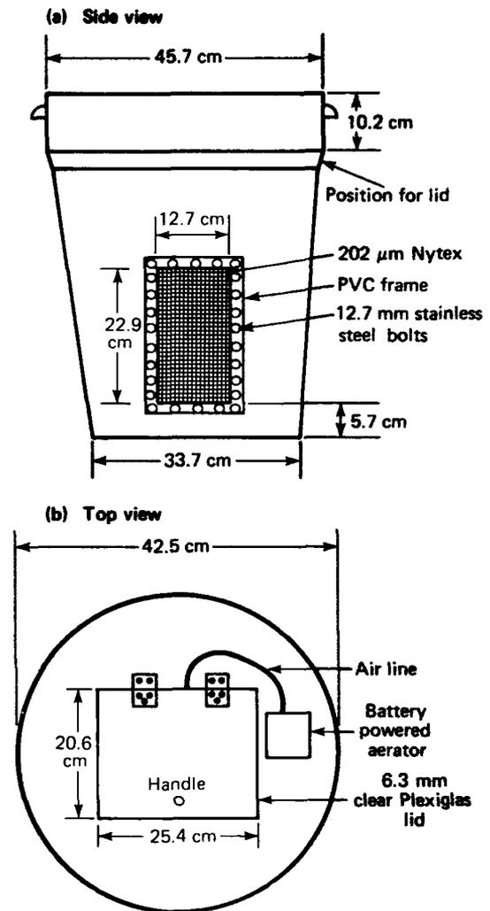
Figure 1—Side and top views of the in-situ test chambers.
