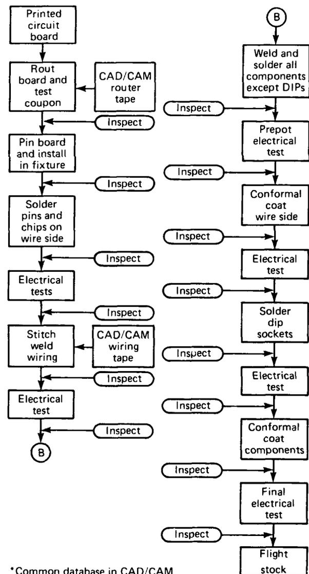
Figure 3—Manufacturing flow chart using unvented socket pins.
