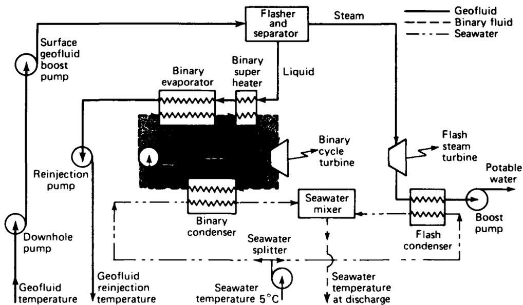
Figure 2—Simplified diagram of GEOTEC plant using a flash-binary cycle.
