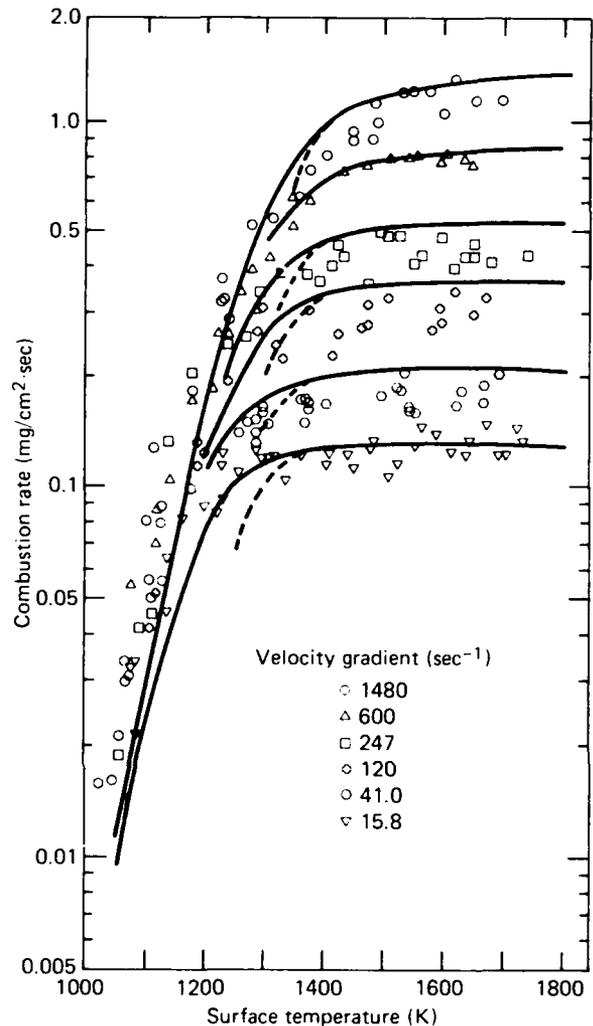
**Figure 2**—The ablation of carbon burning in air. Experimental points<sup>2,3</sup> are compared with calculations<sup>1</sup> for glowing combustion (solid lines) and flaming combustion (dashed lines). The oxygen mass concentration is  $0.284 \times 10^{-3} \text{ g} \cdot \text{cm}^{-3}$ .
