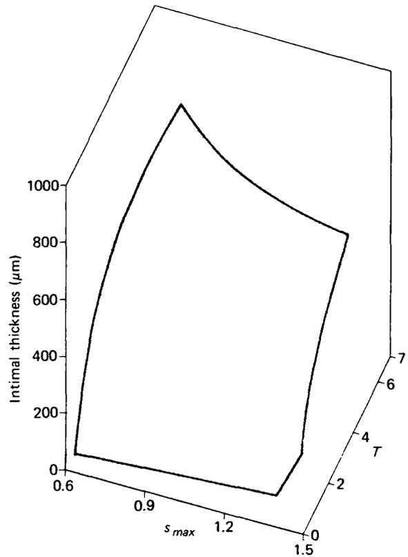
**Figure 1**—Correlation of intimal thickness with nondimensional time,  $T$ , and normalized maximum shear rate,  $s_{max}$ . The region in the  $s_{max} - T$  space within which the correlation applies is indicated by heavy lines; the rest of the surface is included to provide a better sense of its shape. Nondimensional time is defined by  $T = r_o t$ , where  $r_o$  is the removal rate constant at  $s_{max} = 1$  and  $t$  is physical time.
