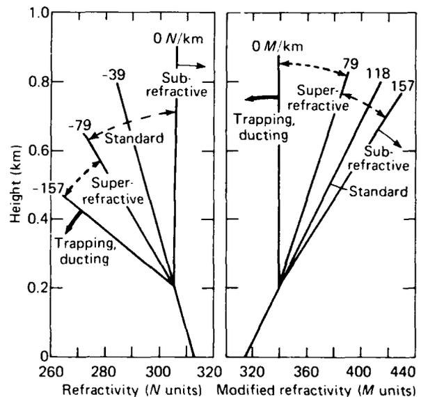
Figure 1— $N$  and  $M$  gradients and refractive effects.
