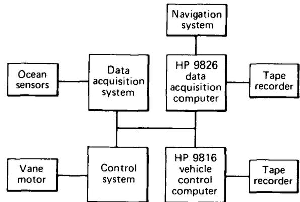
Figure 3—Block diagram of the measurement system.
