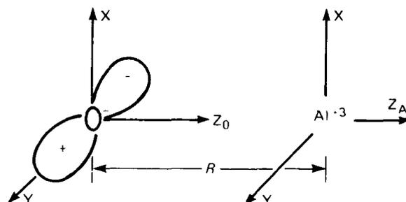
**Figure 1**—Coordinate convention for the aluminum-oxygen centers where the unpaired electron is in a  $\pi$ -orbital ( $2p_y$ ) localized on the oxygen and the  $\text{Al}^{+3}$  nucleus is on the nodal plane of this orbital.
