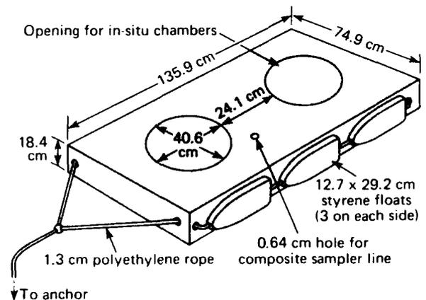
Figure 2—Raft used to house the test chambers in the river.
