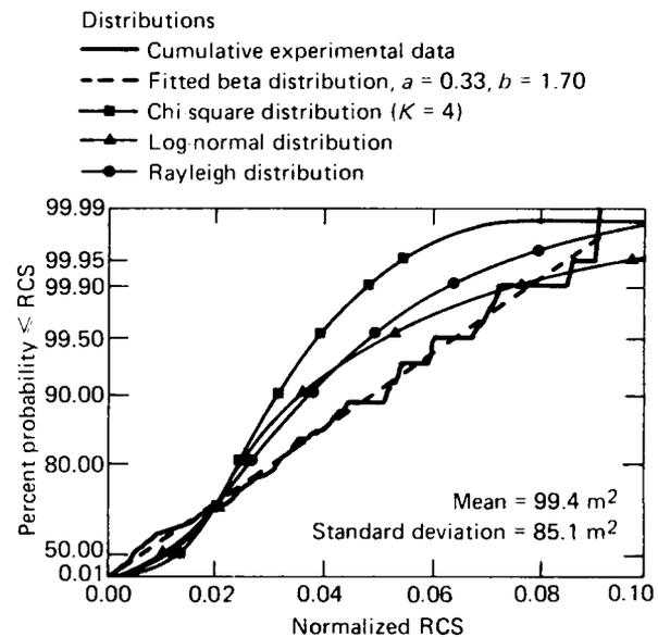
**Figure 3**—RCS of Boeing 727-100C in the wing plane; 0.95 GHz; horizontal polarization; data window 85° to 95°.
