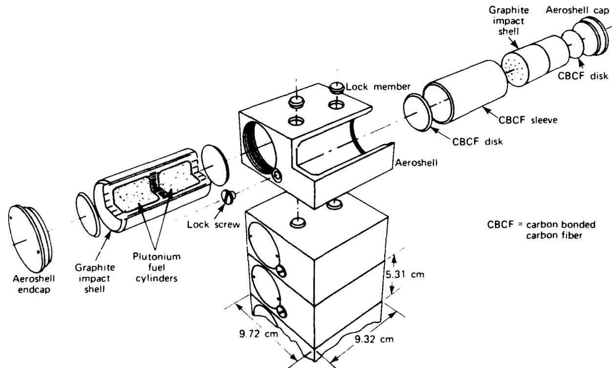
Figure 1—The General Purpose Heat Source.
