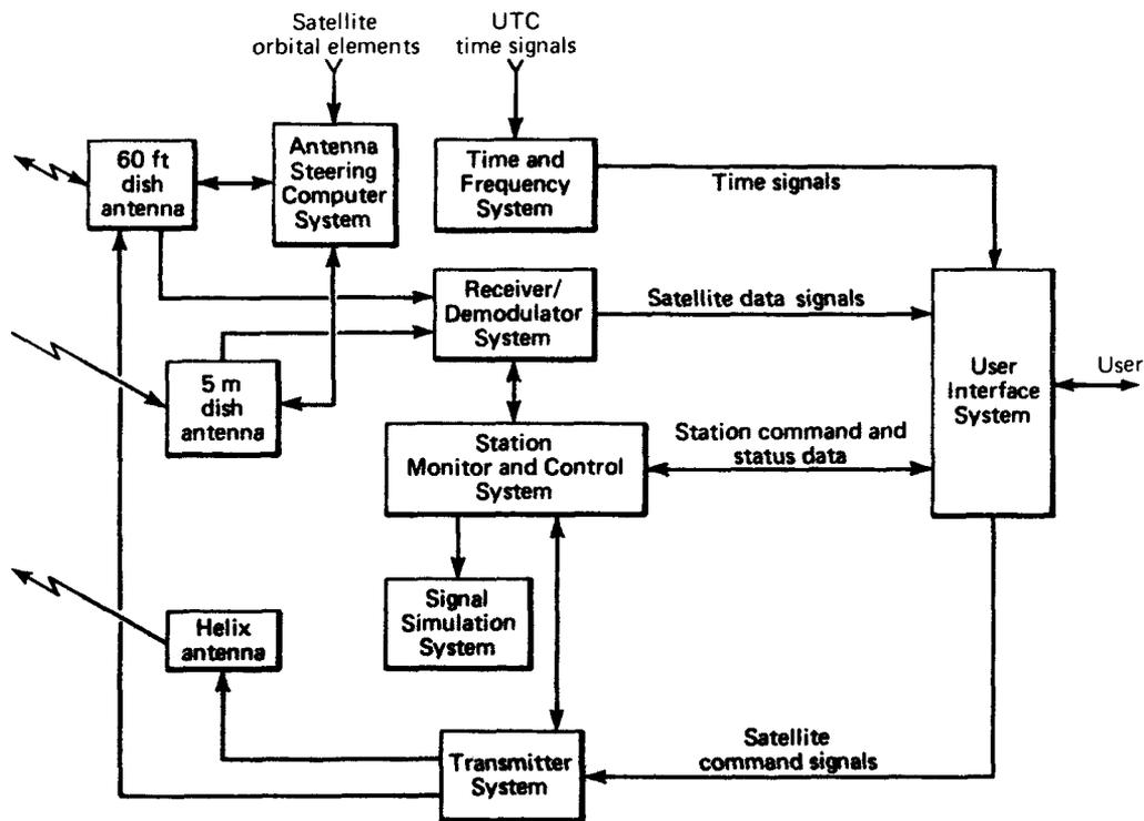
Figure 1—Block diagram of the Satellite Tracking Facility.
