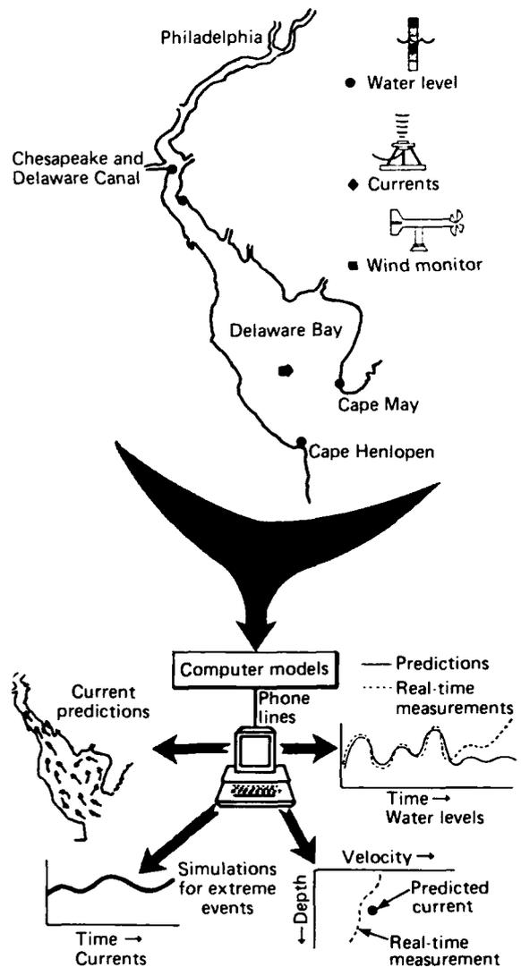
Figure 1—The real-time measurement system.
