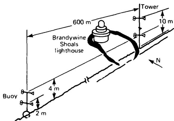
Figure 3—Schematic of the buoy and tower installation.
