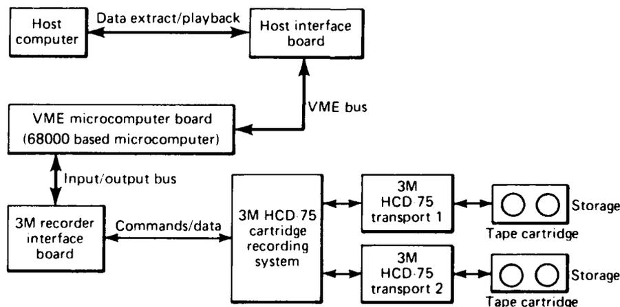
Figure 3—Block diagram of the 3M/CMTU.
