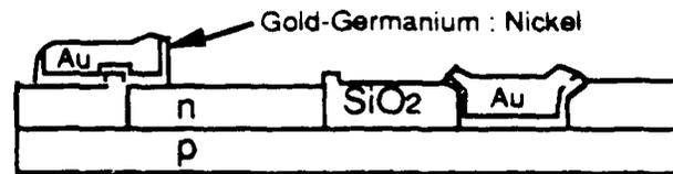
Assuming the range of operation frequency is between 2 ~ 200 GHz, the thickness of n-layer is chosen as 1  $\mu\text{m}$  by previous discussion.
