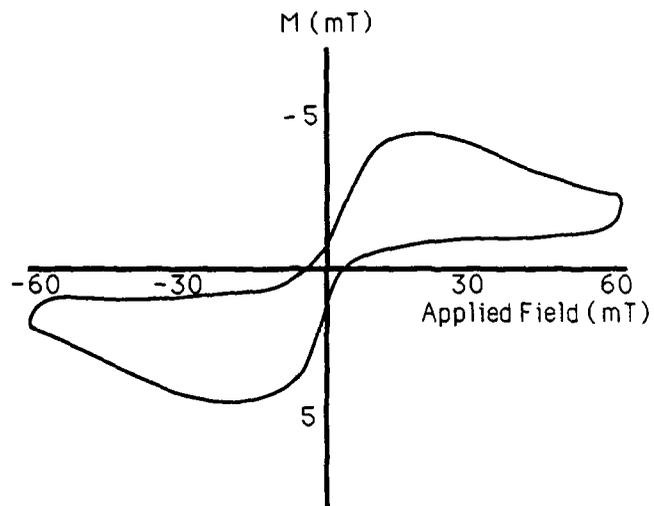
Figure 1: a typical magnetisation curve for a large grained sample of YBCO measured at 77K.
