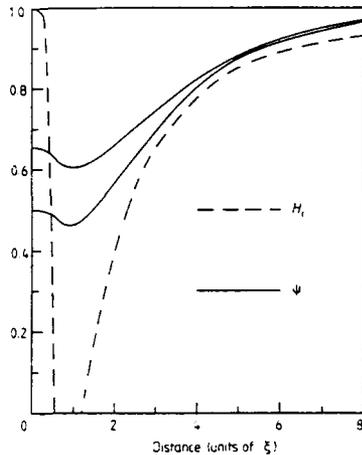
**Figure 8.** The variation of  $H_c$  and  $\psi$  near a low-angle grain boundary of  $6^\circ$  inclination if  $T_c$  goes to zero at a strain of 10%. The order parameter is plotted for both zero and critical current.
