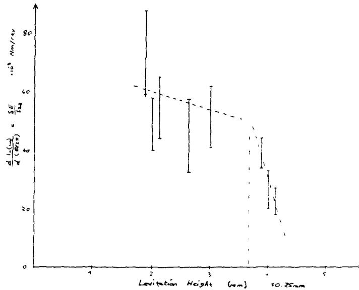
Diagram 2.6: Variation of loss with levitation height
