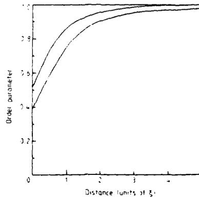
Figure 1. Variation of order parameter with distance from the boundary  $\Lambda = \xi$ . The two curves are for  $j = 0$  and for  $j = 0.5$ .  $j = 1$  is the bulk depairing current and 0.5 the critical current of the barrier
