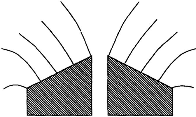
figure 1 the magnetic field profile close to the pole of the hollow conical magnet.
