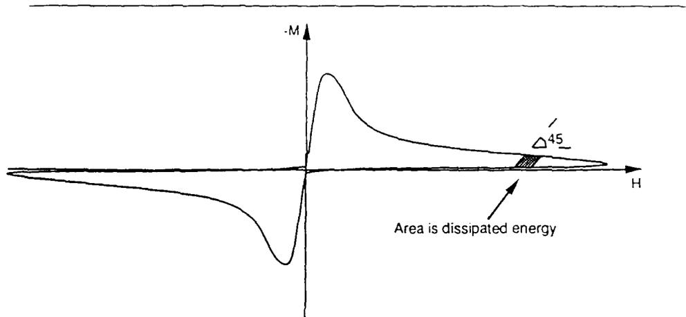
Diagram 1.2: Hysteretic loss on a magnetisation diagram
