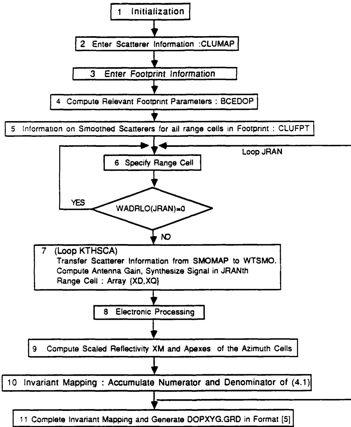
Figure 4.1 Simulation of a single footprint : DOPXYS
