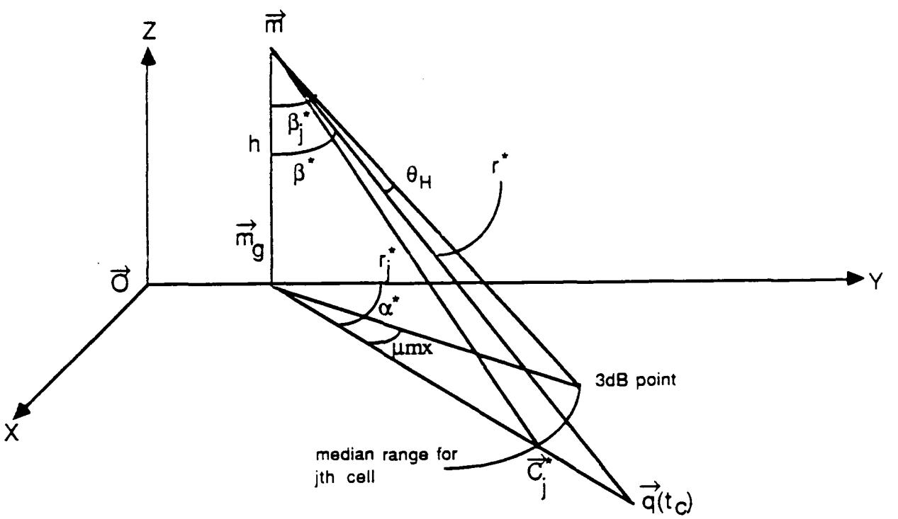
Figure A.3 Maximum relative azimuth angle  $\mu_{mx}$ ,  $\theta_H$  = half beamwidth.
