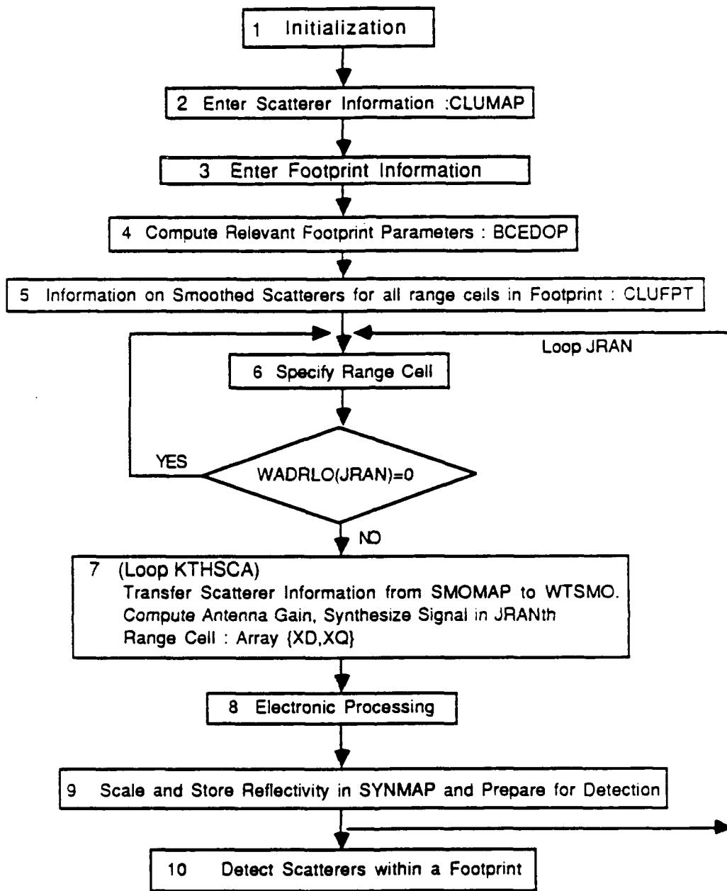
Figure 3.1 Simulation of a single footprint : DOPFPS
