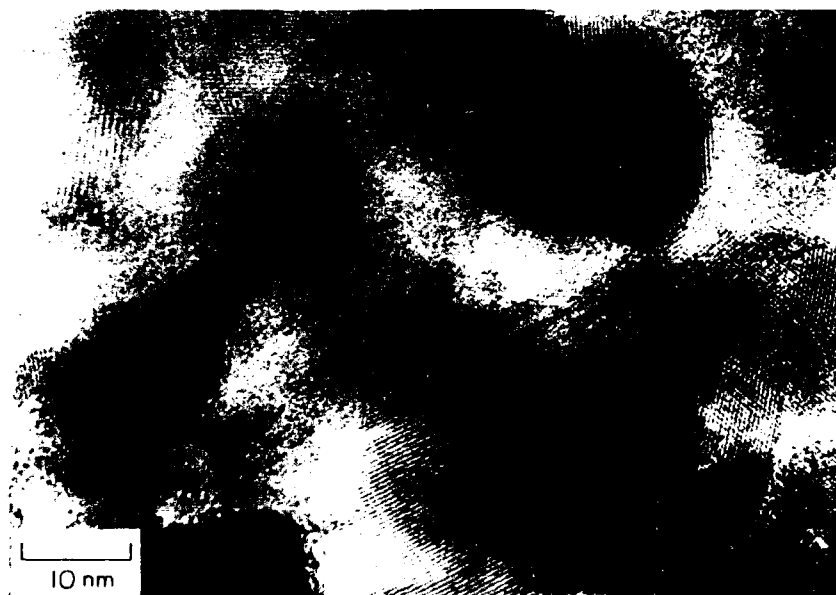
FIGURE 16 High-resolution transmission electron micrograph of nanophase \text{TiO}_2 (rutile) after sintering for one-half hour at 500^\circ\text{C} (Siegel and Hahn, 1987).
