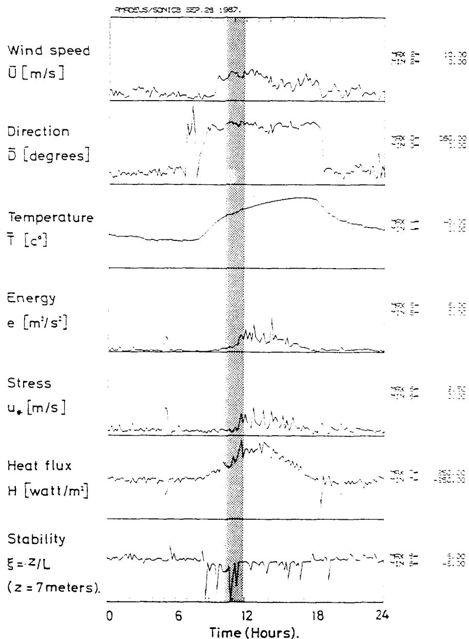
Figure 21: 10-min mean values for Run # 6.
