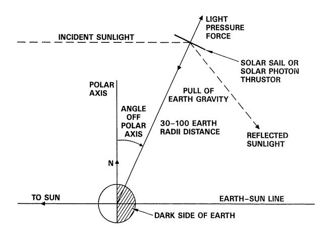
Fig. 2 - The Statite Concept
