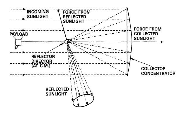
Fig. 1 - The Solar Photon Thruster Concept
