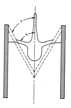
Figure 6. <u>Schematic Collapse of a Typical Shaped Charge With a Conical Liner (Walters and Zukas 1989)</u>.
