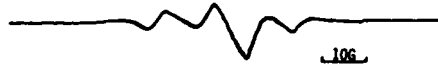
Fig. TCNQ-oT=1:1 1% film : subtraction of the low power ( 1.98 mW ) spectrum from the high power ( 198 mW ) spectrum.
