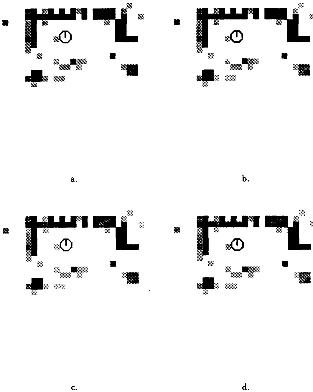
Figure G-6: Examples of the final Room 914 model using the linear update algorithm with Hysteresis = 3 and various rise times.
