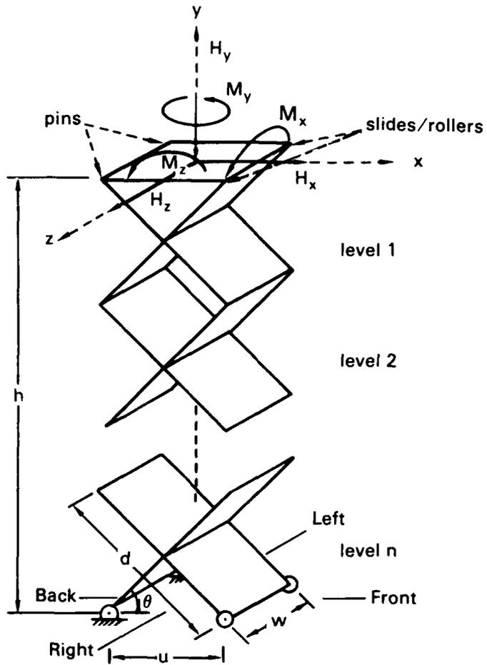
Figure 1. Nomenclature: applied loads and scissor lift dimensions.
