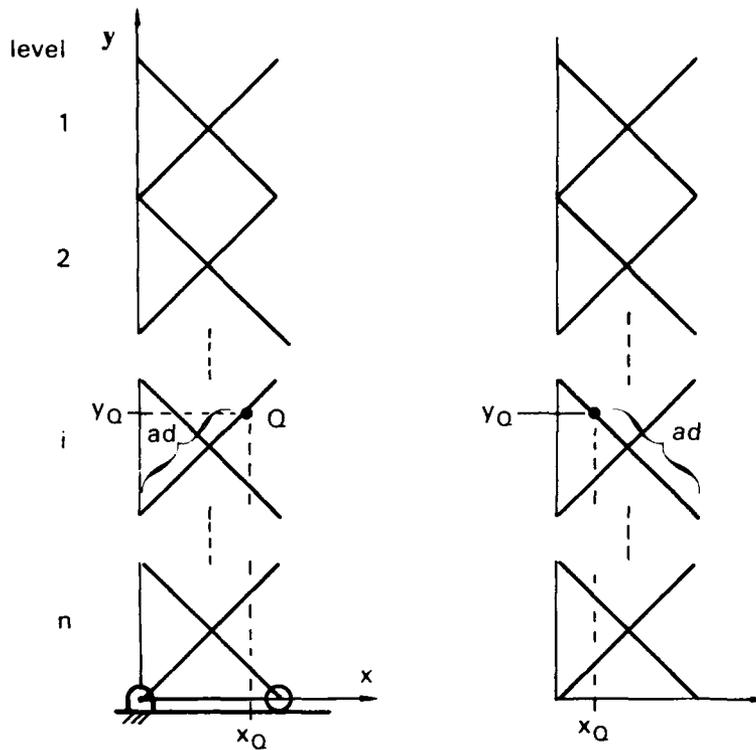
Figure 21. Coordinates of a point on the lift.
