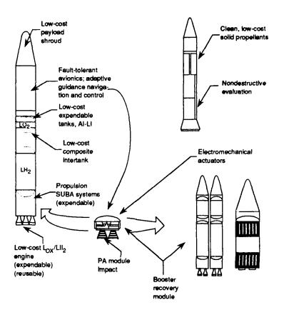
Figure 7-5 Advanced Launch System Vehicle Technologies
