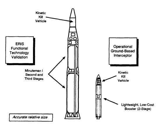
Figure 5-10 ERIS Functional Technology Validation Kinetic Kill Vehicle
