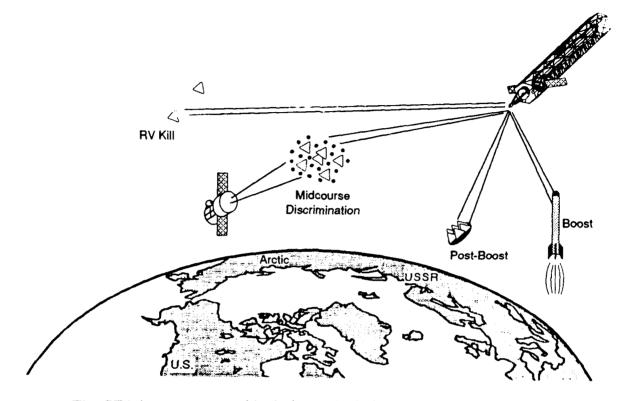
Figure 6-4 Space-Based Neutral Particle Beam Concept
